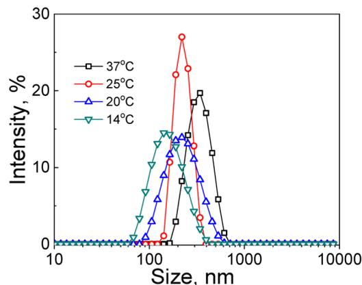
Fig. 3 The hydrodynamic size of PMVC<sub>58</sub>-*b*-PVPON<sub>65</sub> copolymer vesicles analyzed in solutions at 37 °C (black squares), (b) 25 °C (red circles), (c) 14 °C (blue up-triangles), and (d) 4 °C (green down-triangles) as measured by DLS.
