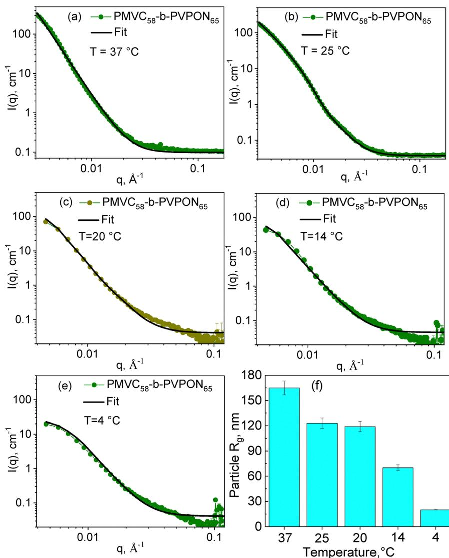
**Fig. 4** SANS plots of the PMVC<sub>58</sub>-*b*-PVPON<sub>65</sub> vesicle solutions and their Guinier fits (solid lines) at (a) 37 °C, (b) 25 °C, (c) 20 °C, (d) 14 °C, and (e) 4 °C. (f) The dependence of particle  $R_g$  on solution temperature obtained from SANS plot fits (a)–(e).
