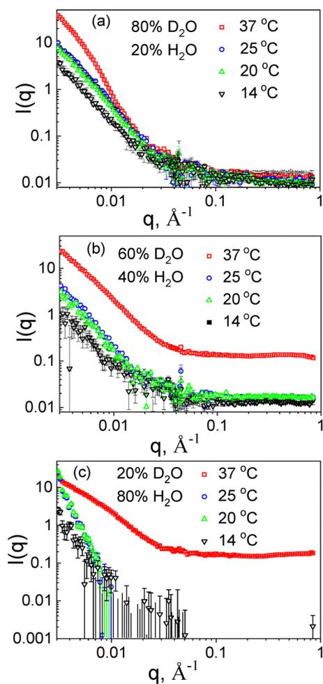
Fig. 6 Contrast-matching SANS plots of PMVC<sub>58</sub>-*b*-PVPON<sub>65</sub> vesicles prepared in a solvent mixture of (a) 80/20% D<sub>2</sub>O/H<sub>2</sub>O, (b) 60/40% D<sub>2</sub>O/H<sub>2</sub>O, and (c) 20/80% D<sub>2</sub>O/H<sub>2</sub>O.
