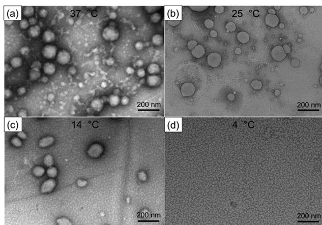
Fig. 2 TEM images of PMVC<sub>58</sub>-*b*-PVPON<sub>65</sub> polymersomes dried on TEM grids from solutions at (a) 37 °C, (b) 25 °C, (c) 14 °C, and (d) 4 °C.
