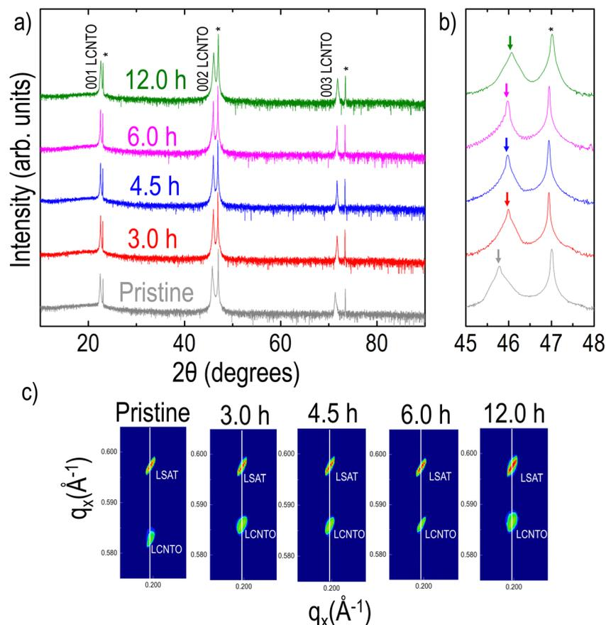
**Fig. 1** (a) XRD  $\theta$ - $2\theta$  patterns of the LCNTO thin films before and after reduction at 900 °C with varying reduction times (substrate peaks are indicated with \*). (b) XRD  $\theta$ - $2\theta$  patterns around the 002 peaks (the 002 Bragg reflections from the LCNTO thin film and the substrates are denoted as arrows and asterisks, respectively). (c) XRD RSMs are shown around the asymmetric 103 reflection of the films and substrates.
