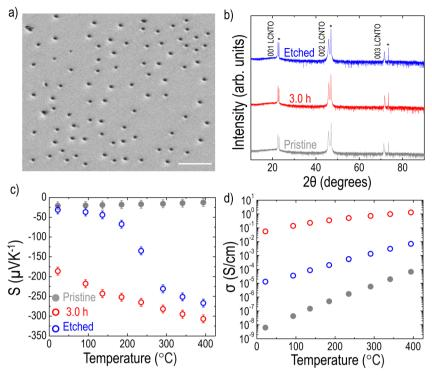
Fig. 7 (a) SEM image of the LCNTO sample reduced at 900 °C 3.0 h after etching in nitric acid (scale bar: 1  $\mu$ m). (b) XRD  $\theta$ –2 $\theta$  patterns of the pristine, reduced, and etched LCNTO thin films (substrate peaks are indicated with \*). Temperature dependencies of (c) S and (d)  $\sigma$  of the pristine, reduced, and etched LCNTO thin films measured from 20 to 400 °C.
