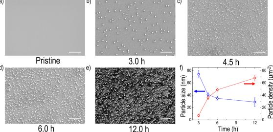
Fig. 2 SEM images of the surface of LCNTO thin films: (a) before exsolution and (b) after exsolution at 900 °C for 3.0 h, (c) 4.5 h, (d) 6.0 h, and (e) 12.0 h. (f) The relationship between particle size and density of the exsolved samples, obtained by processing the SEM images using ImageJ software. The scale bar indicates 1 µm.
