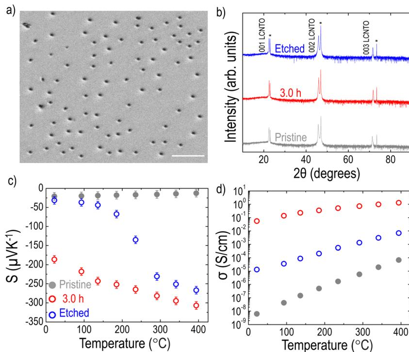
Fig. 7 (a) SEM image of the LCNTO sample reduced at 900 °C 3.0 h after etching in nitric acid (scale bar: 1 μm). (b) XRD  $\theta$ - $2\theta$  patterns of the pristine, reduced, and etched LCNTO thin films (substrate peaks are indicated with \*). Temperature dependencies of (c)  $S$  and (d)  $\sigma$  of the pristine, reduced, and etched LCNTO thin films measured from 20 to 400 °C.
