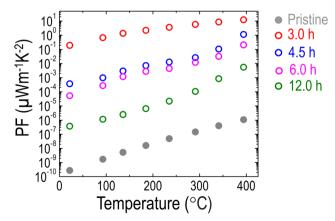
Fig. 6 Temperature dependencies of the PF of the LCNTO thin films before and after reduction at 900 °C with varying reduction times.
