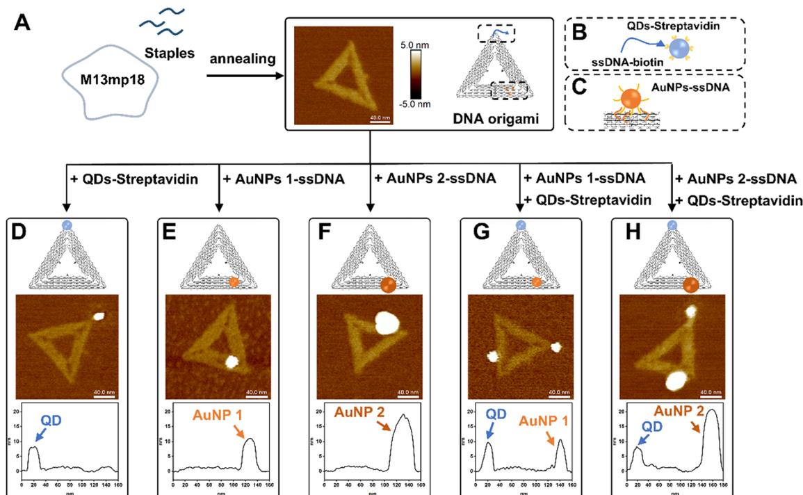
**Fig. 1** Synthesis and functionalisation of DNA origami with QDs and AuNPs. (A) Schematic of DNA origami synthesis. (B) Cartoon of DNA origami functionalised with QDs via biotin–streptavidin coupling, and (C) of ssDNA functionalised AuNPs complementary hybridisation on predefined sticky ends of DNA origami. Schematic, topographic AFM image and corresponding height profile of DNA origami modified with (D) one QD, (E) AuNP 1, (F) AuNP 2, (G) AuNP 1 and QD, and (H) AuNP 2 and QD.
