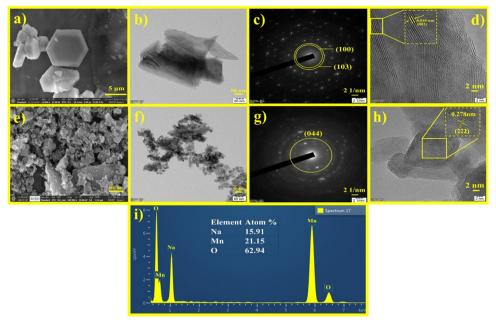
Fig. 3 HRSEM images of (a) Na<sub>0.6</sub>MnO<sub>2</sub> and (e) Mn<sub>2</sub>O<sub>3</sub>; (b) and (f) HRTEM images of Na<sub>0.6</sub>MnO<sub>2</sub> and Mn<sub>2</sub>O<sub>3</sub>; (c) and (g) SAED patterns of Na<sub>0.6</sub>MnO<sub>2</sub> and  $Mn_2O_3$ ; (d) and (h) lattice fringes of  $Na_{0.6}MnO_2$  and  $Mn_2O_3$ ; (i) EDX elemental analysis of  $Na_{0.6}MnO_2$ .
