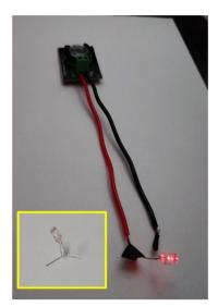
Fig. 13 Digital image of the Zn||Na<sub>0.6</sub>MnO<sub>2</sub> battery powering a red LED. Inset: LED without connection to the Zn||Na<sub>0.6</sub>MnO<sub>2</sub> battery.
