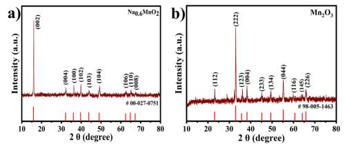
Fig. 2  $\,$  XRD patterns of the hydrothermally synthesized (a)  $Na_{0.6}MnO_2$  and (b)  $Mn_2O_3$ .
