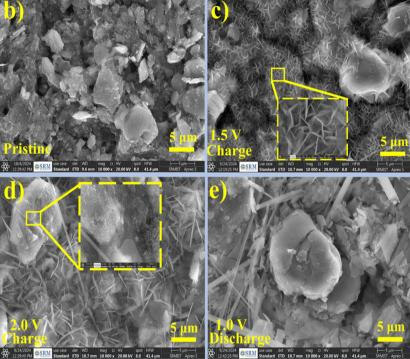
Fig. 8 (a) Charge-discharge curve of the  $Na_{0.6}MnO_2$  electrode during the first cycle, SEM images for the (b) pristine electrode; (c) charged to 1.5 V; (d) fully charged state (2.0 V); (e) fully discharged state at 1.0 V.
