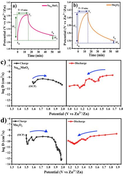
Fig. 9 Single GITT curves of (a) Na<sub>0.6</sub>MnO<sub>2</sub>; (b) Mn<sub>2</sub>O<sub>3</sub>; (c) diffusion coefficient values of Na<sub>0.6</sub>MnO<sub>2</sub> during charge-discharge; (d) diffusion coefficient values of Mn<sub>2</sub>O<sub>3</sub> during charge-discharge
