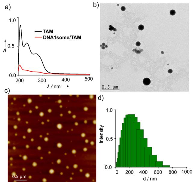
**Fig. 1** (a) Comparison of the absorption spectra of free **TAM** and **TAM** present in the filtrate of **DNA1some/TAM**. (b) AFM and (c) TEM images of **DNA1some/TAM**. (d) DLS size distribution of **DNA1some/TAM** aggregates.
