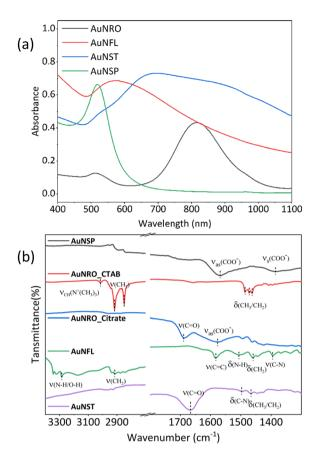
Fig. 2 (a) Vis-NIR absorption spectra (400-1100 nm) of AuNSP-citrate, AuNRO-CTAB, AuNFL-dopamine, and AuNST-PVP, [ $Au^0$ ] = 0.2 mM. (b) ATR-FTIR spectra of the same.
