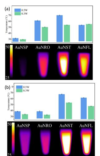
Fig. 3 Plateau temperatures reached after 5 min. of irradiation at 808 nm (a) or 1064 nm (b) of AuNP suspensions: AuNSP-citrate, AuNRO-citrate, AuNFL-dopamine, and AuNST-PVP, [Au<sup>0</sup>] = 0.2 mM.
