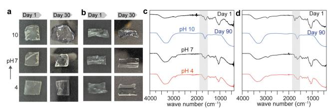
Fig. 4 Photographs of (a) CMC-CA (CMC: CA = 1:1) and (b) CMC-CA-Al (CMC: CA = 1:1 soaked in 0.1 M Al<sup>3+</sup> solution) dual-cross-linked hydrogel films taken before and after immersion in aqueous solutions of pH = 4, 7 and 10 for up to 30 days. Solid-state attenuated FTIR transmittance plots of (c) CMC-CA and (d) CMC-CA-Al hydrogels acquired before and after exposure to pH 4, 7 and 10 for 90 days.
