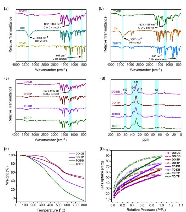
Fig. 1 (a) and (b) FT-IR spectra of **DOIDB** and **TOITP** with their monomers and organic linkers. (c) FT-IR spectra, (d) solid-state  $^{13}$ C NMR, (e) TGA and (f) CO<sub>2</sub> adsorption–desorption isotherms of **DOIDB**, **DOITP**, **TOIDB**, and **TOITP**.
