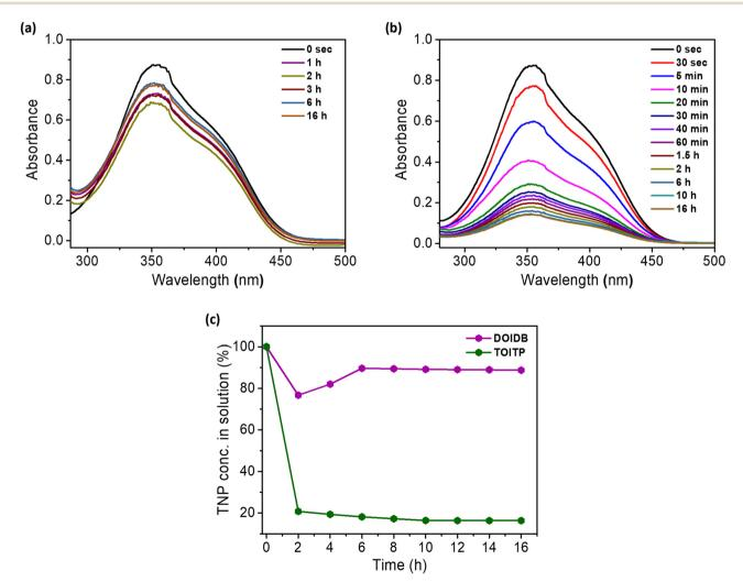
Fig. 8 (a) and (b) UV-vis absorption spectra of TNP solutions with **DOIDB** and **TOITP** in MeOH, showing changes in the concentrations of TNP at different intervals of time. (c) Percentage of TNP left in the solution after the equilibrium is reached for each of the polymers.
