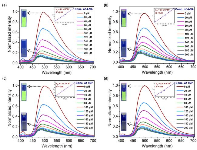
Fig. 5 (a) and (b) Fluorescence quenching of the suspensions of **DOIDB** and **TOITP** in MeOH, respectively, with increasing concentrations of 4-NA; the Stern-Volmer plots are shown in the insets. (c) and (d) Fluorescence quenching of the suspensions of **DOIDB** and **TOITP** in MeOH, respectively, with increasing concentrations of TNP; the corresponding Stern-Volmer plots are shown in the insets.
