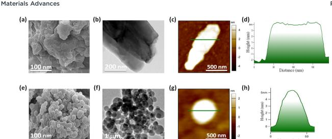
Fig. 2 (a) and (b) SEM and TEM images of DOIDB, respectively. (c) and (d) AFM image and height-profile diagram of the nanosheet of DOIDB. (e) and (f) SEM and TEM images of TOITP, respectively. (g) and (h) AFM image and height-profile diagram of the nanosphere of TOITP
