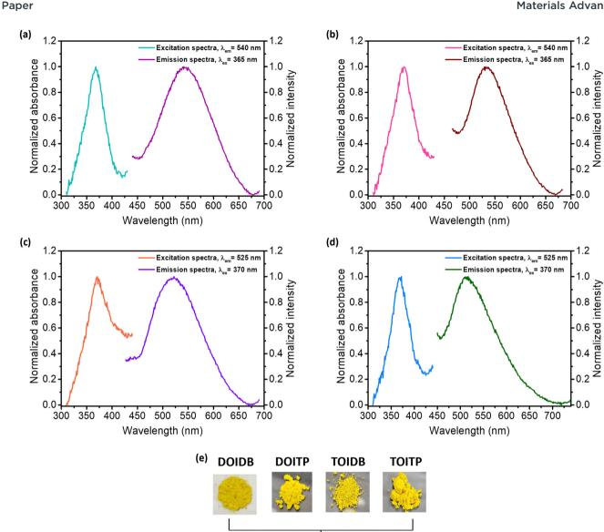
Fig. 3 Solid-state fluorescence excitation and emission spectra of (a) DOIDB, (b) DOITP, (c) TOIDB and (d) TOITP, respectively. (e) Images of the polymers in room light and under exposure to 360 nm radiation.
