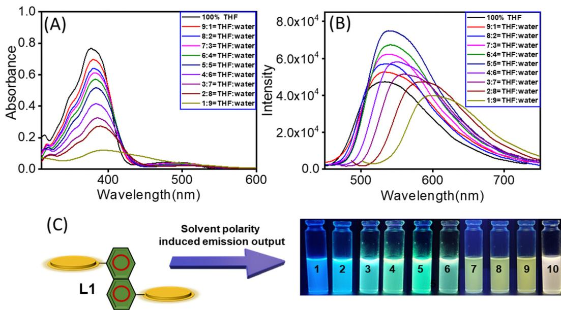
Fig. 1 (A) UV-Vis and (B) emission spectra of **L1** in THF and different THF:water mixtures. (C) Photographs showing the change in fluorescence colours of **L1** upon irradiation with 365 nm light at different ratios of the THF:water mixtures.
