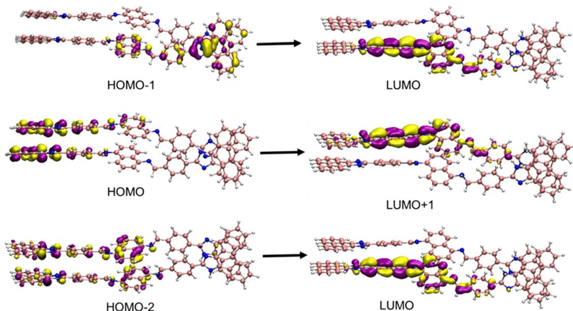
Fig. 5 Frontier molecular orbitals of the calculated minima structure of the **L1** dimer involved in the main absorption peak at wB97XD/def2-TZVPP in a THF : water = 1 : 9 mixture. [C: pink, N: blue, H: white]. The density of the molecular orbitals is shown in yellow and violet with an isosurface value of 0.03.
