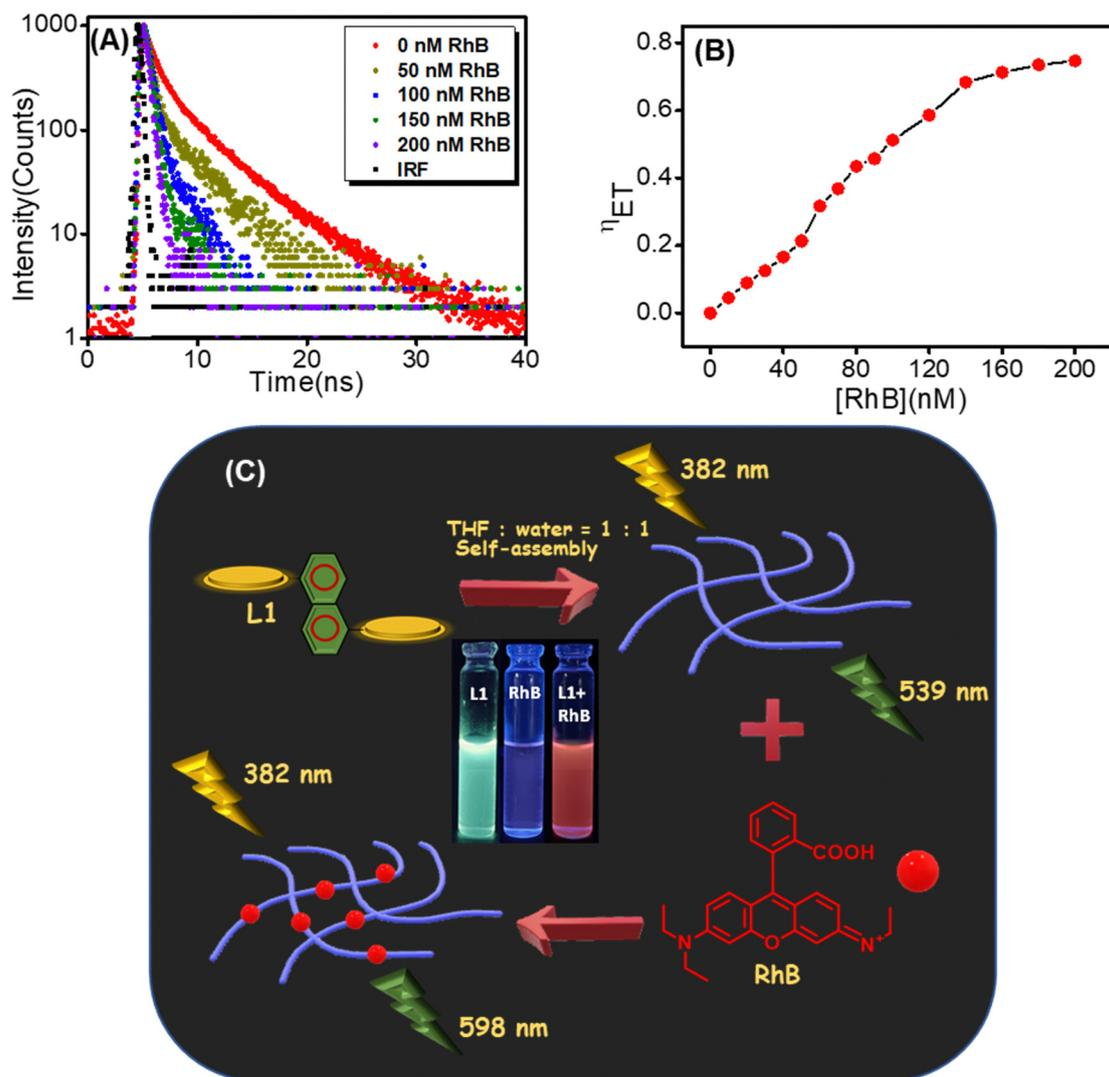
Fig. 8 (A) Fluorescence lifetime decay profiles ( $\lambda_{\text{Ext}} = 382$  nm, monitored at 539 nm) of **L1** upon the addition of different concentrations of RhB (0–200 nM). IRF – instrument response time. (B) Energy transfer efficiency as a function of [RhB]. (C) Schematic representation of the self-assembled **L1**/RhB-based light-harvesting system.
