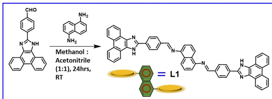
Scheme 1 Schematic representation of the synthesis of **L1**.
