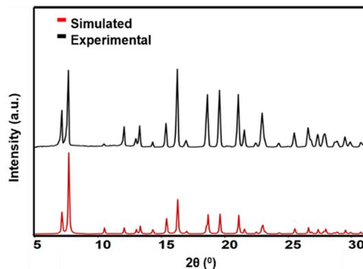
Fig. 1 Comparison of ZIF-7 PXRD patterns: simulated pattern from single crystal X-ray diffraction data<sup>31</sup> (red) and experimental pattern (black).
