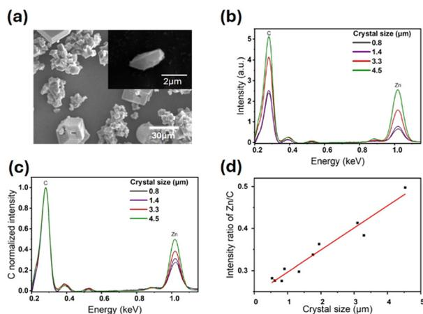
**Fig. 4** (a) Typical SEM image of a ZIF-7 prism-like crystal with a representative individual prism-like crystal where the EDX spectrum is collected, (b) absolute and (c) C-normalized EDX spectra of several selected ZIF-7 prism-like crystals of various sizes, and (d) EDX peak intensity ratio of Zn/C as a function of ZIF-7 prism-like crystal size; the solid red line is shown for illustrative purposes only.
