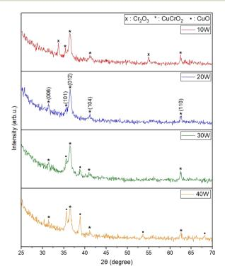
Fig. 2  $\,$  XRD diffractograms of films deposited at varying copper powers and annealed at 800  $\,^{\circ}$ C.
