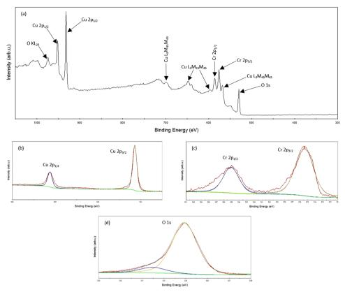
Fig. 3 XPS spectra of the CuCrO<sub>2</sub> film deposited with a copper sputtering power of 20 W: (a) survey spectrum; (b) Cu-2p state; (c) Cr-2p state; (d) O-1s state.
