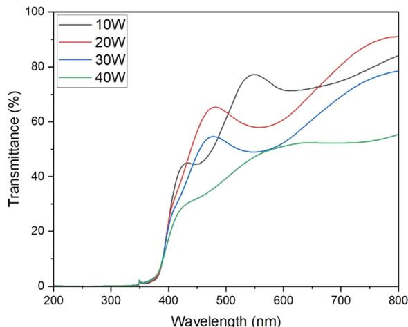
Fig. 5 Optical transmissions of CuCrO<sub>2</sub> films deposited with various copper sputtering powers.
