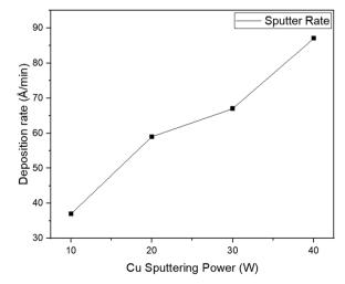
Fig. 1 Sputtering rate for various copper sputtering powers.
