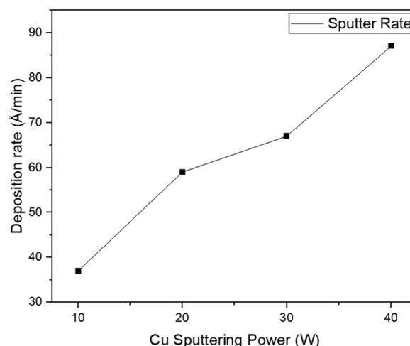
Fig. 1 Sputtering rate for various copper sputtering powers.
