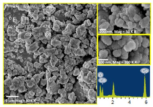
FESEM images of green synthesized Co<sub>3</sub>O<sub>4</sub> NPs at different magnifications: (a) at 30 000 (b) at 50 000, (c) at 100 000 magnifications, and (d) EDX spectrum.
