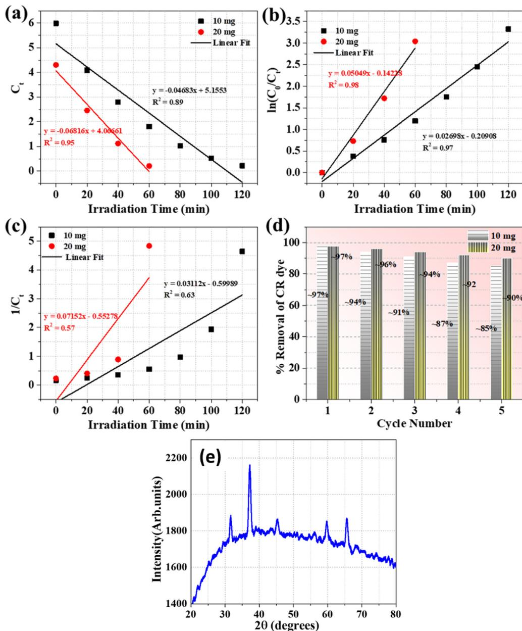
Fig. 10 Kinetics of CR dye: (a) Pseudo-zero-order, (b) Pseudo-first-order, and (c) Pseudo-second-order, (d) reusability of TFG- $\text{Co}_3\text{O}_4$ , and (e) stability of TFG- $\text{Co}_3\text{O}_4$ .
