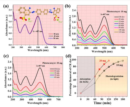
Fig. 8 Photodegradation of CR dye using Co<sub>3</sub>O<sub>4</sub> NPs.
