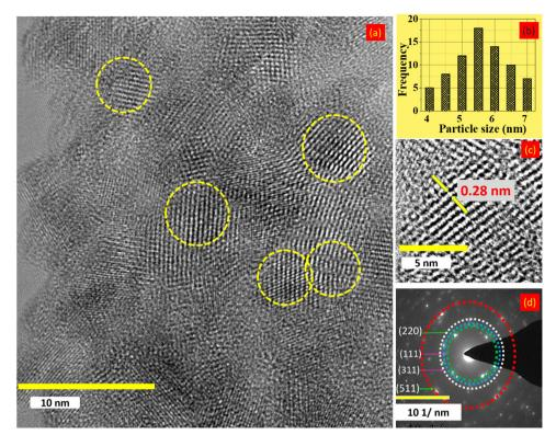
Morphological exploration of TFG-mediated Co<sub>3</sub>O<sub>4</sub> NPs: (a) TEM image, (b) particle size distribution, (c) d-spacing HRTEM, and (d) SAED pattern.
