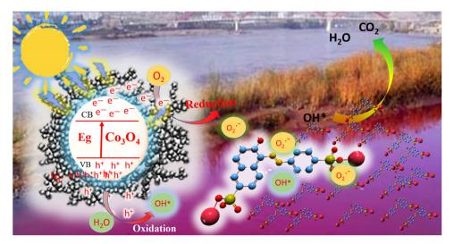
Proposed photocatalytic degradation mechanism of Co<sub>3</sub>O<sub>4</sub> NPs.
