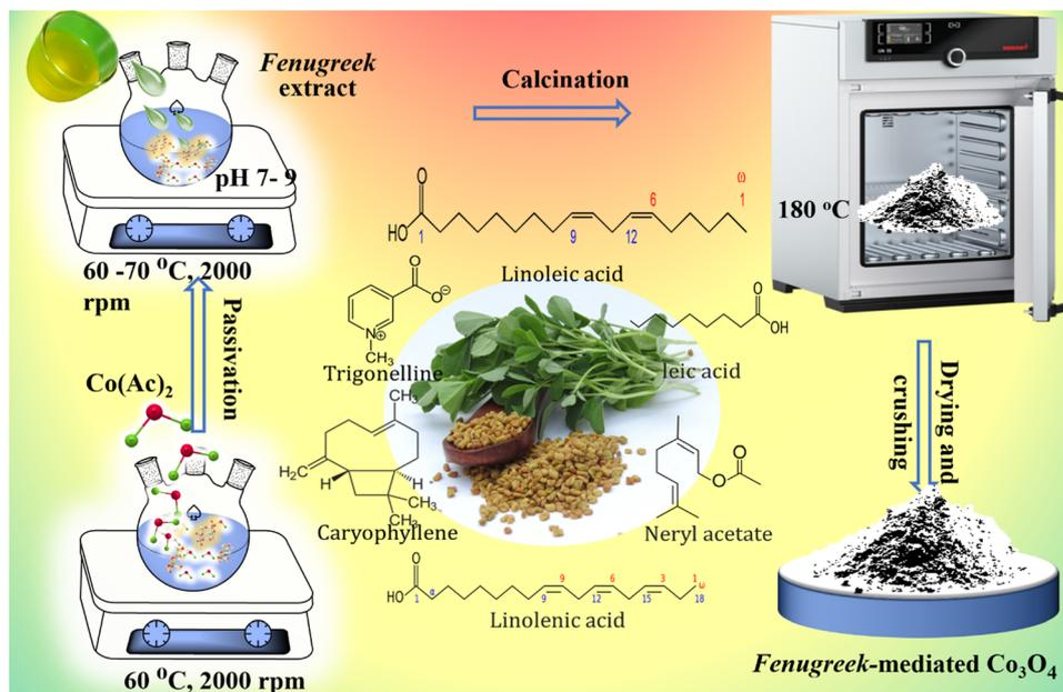
Fig. 1 Synthesis of *Trigonella foenum-graecum*-mediated  $\text{Co}_3\text{O}_4$  nanoparticles.
