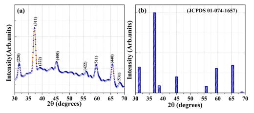
Fig. 2 (a) XRD pattern of TFG mediated  $Co_3O_4$  NPs and (b) standard JCPDS of  $Co_3O_4$ .
