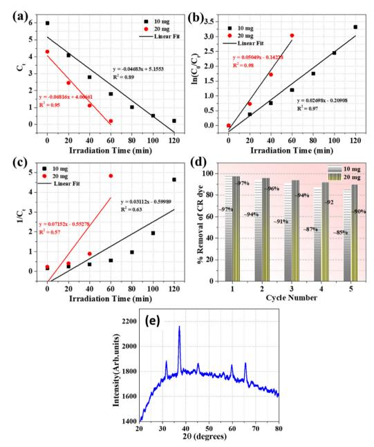
Fig. 10 Kinetics of CR dye: (a) Pseudo-zero-order, (b) Pseudo-first-order, and (c) Pseudo-second-order, (d) reusability of TFG- $Co_3O_4$ , and (e) stability of TFG- $Co_3O_4$ .
