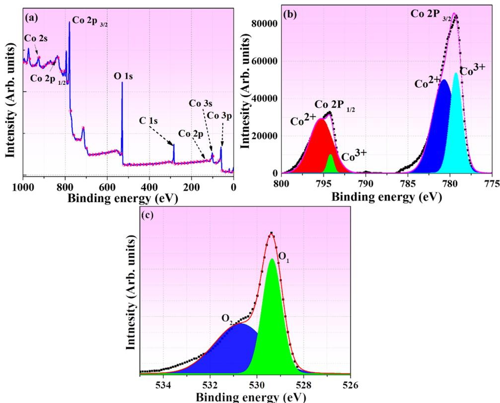
Fig. 7 XPS analysis of  $\text{Co}_3\text{O}_4$  NPs: (a) Holistic elemental survey (b) cobalt chemical environment – Co 2p spectra, and (c) oxygen's role in  $\text{Co}_3\text{O}_4$  Structure – O 1s Spectra.
