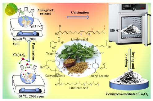
Fig. 1 Synthesis of Trigonella foenum-graecum-mediated Co<sub>3</sub>O<sub>4</sub> nanoparticles.
