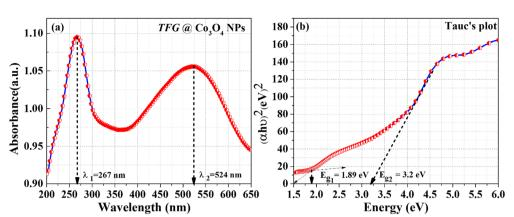
Fig. 4 UV-vis. analysis of (a) TFG-mediated Co<sub>3</sub>O<sub>4</sub> NPs (b) Tauc plot of Co<sub>3</sub>O<sub>4</sub> NPs.
