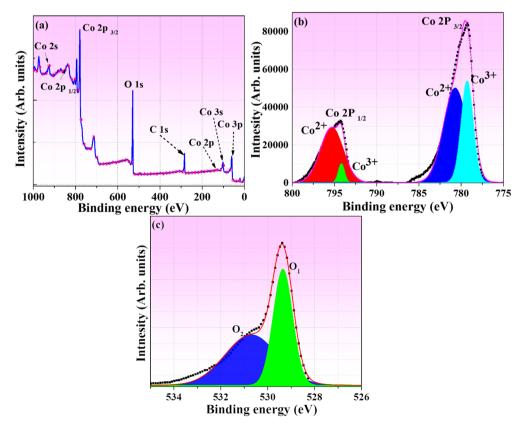
Fig. 7 XPS analysis of  $Co_3O_4$  NPs: (a) Holistic elemental survey (b) cobalt chemical environment – Co 2p spectra, and (c) oxygen's role in  $Co_3O_4$  Structure – O 1s Spectra.
