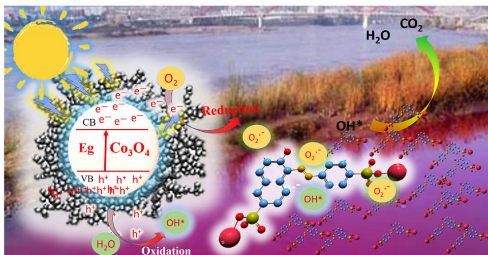
Fig. 9 Proposed photocatalytic degradation mechanism of  $\text{Co}_3\text{O}_4$  NPs.
