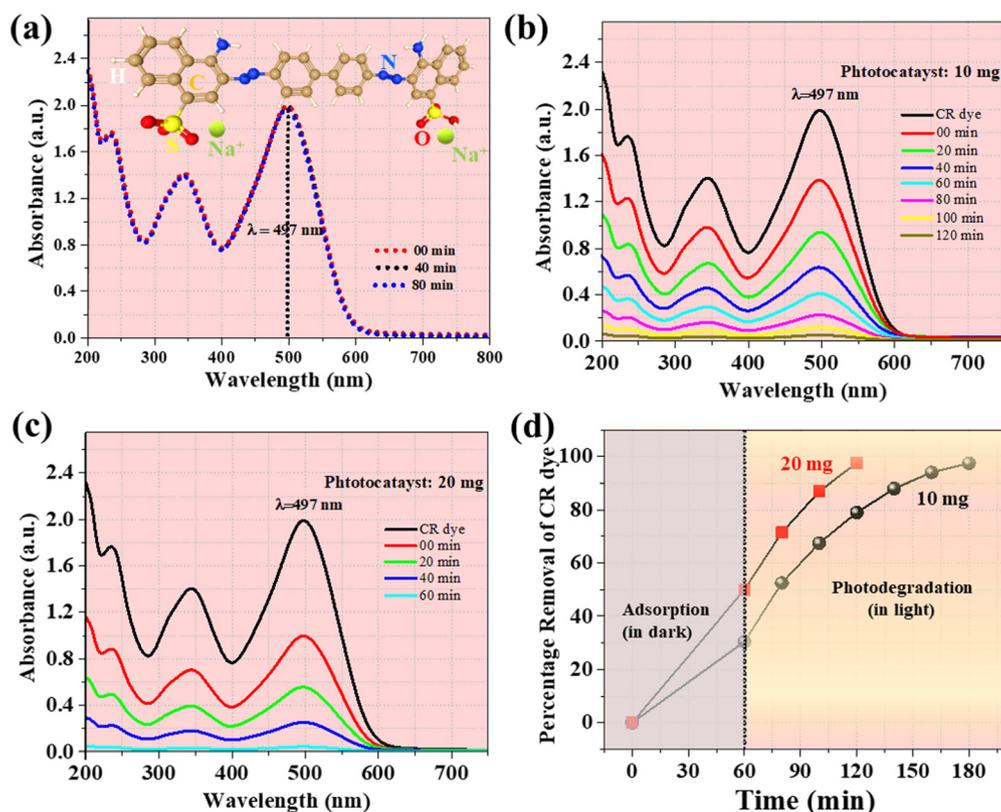
Fig. 8 Photodegradation of CR dye using  $\text{Co}_3\text{O}_4$  NPs.
