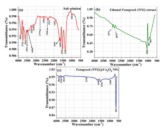
Fig. 3 FTIR analysis of (a) agueous solution of the cobalt salt, (b) ethanol TFG seeds extract, and (c) TFG/Co<sub>3</sub>O<sub>4</sub> NPs.
