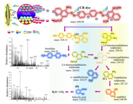
Fig. 11 The GC-MS predicted fragmentation pattern of CR dye photodegradation in the presence of bio-active CP-Co<sub>3</sub>O<sub>4</sub> NPs.
