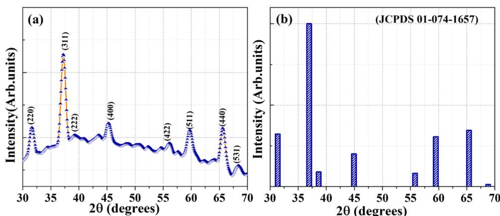
Fig. 2 (a) XRD pattern of TFG mediated Co<sub>3</sub>O<sub>4</sub> NPs and (b) standard JCPDS of Co<sub>3</sub>O<sub>4</sub>.
