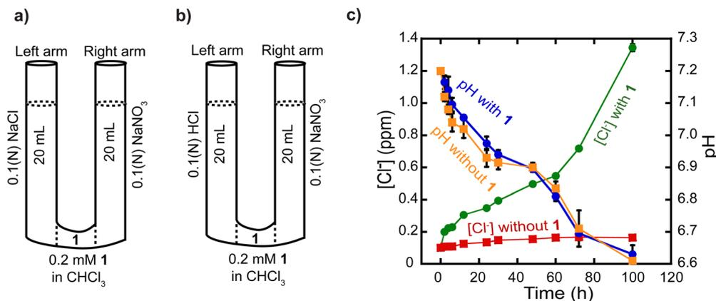
Fig. 6 Transport of  $\text{Cl}^-$  anions across a U-tube. (a) and (b) Simple representation of the experimental setup. (c) Monitoring the  $\text{Cl}^-$  anions concentration and the pH over time using a pH meter and a  $\text{Cl}^-$  selective electrode, respectively. Error bars represent standard deviations from two runs. Some error bars, though present, are so small that they are overshadowed by the symbols representing the data points.
