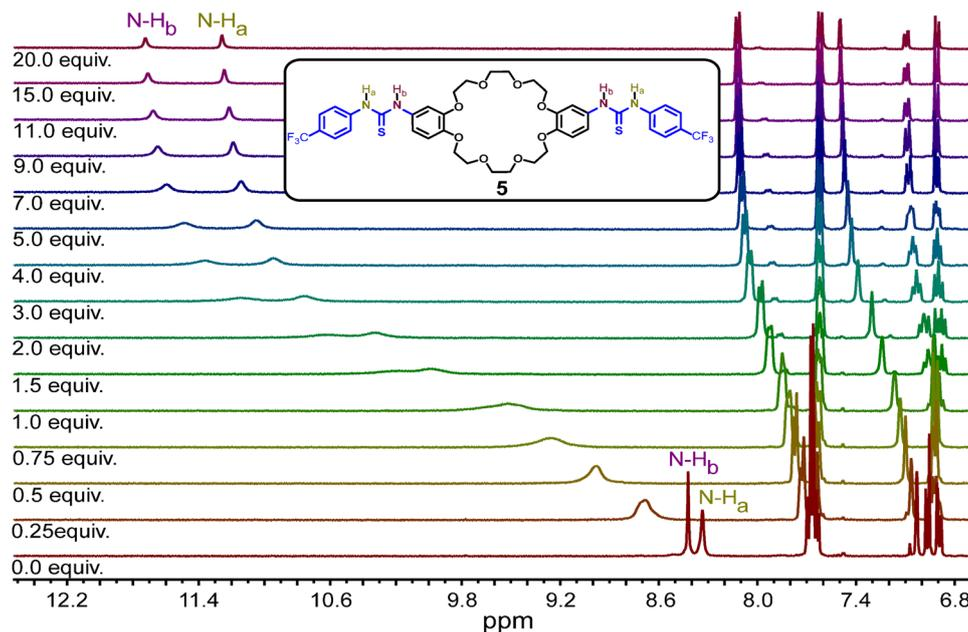
Fig. 2 Recognition and binding of  $\text{Cl}^-$  anions by thiourea units on ring **5**.  $^1\text{H}$  NMR spectra showing the chemical shift of the N–H signals during the titration of ring **5** with different equivalents of TBACl in acetonitrile- $d_3$ .
