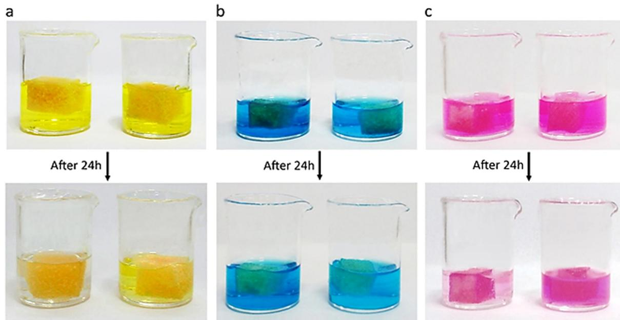
Fig. 4 Supporting PNIPAM<sub>1</sub> on a polyurethane sponge to remove dye impurities from water. Dye solutions (5 ml, 50 ppm) including (a) FL, (b) MB, and (c) RhB were incubated with the PNIPAM<sub>1</sub>-sponge (left) and unmodified sponge (right) as the control for 24 h at room temperature and without shaking. FL and RhB solutions were almost colorless after 24 h incubation with the PNIPAM<sub>1</sub>-sponge but the MB solution was still blue.
