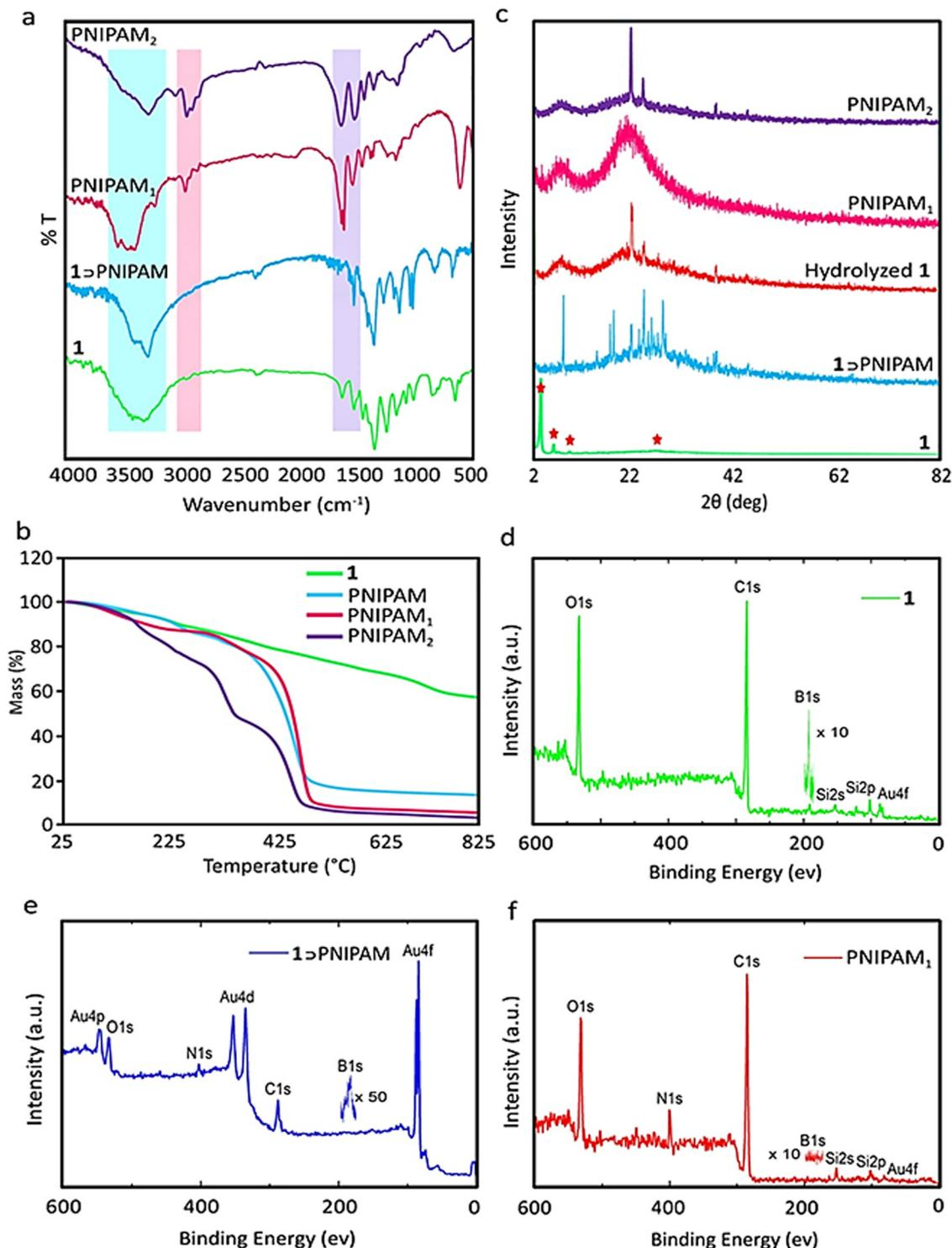
Fig. 2 (a) IR spectra of **1**, **1** to PNIPAM, PNIPAM<sub>1</sub> and PNIPAM<sub>2</sub>. (b) TGA thermograms of **1**, **1** to PNIPAM, PNIPAM<sub>1</sub> and PNIPAM<sub>2</sub>. (c) XRD diffractograms of **1**, **1** to PNIPAM, hydrolyzed **1**, PNIPAM<sub>1</sub> and PNIPAM<sub>2</sub>. (d–f) XPS survey of **1**, **1** to PNIPAM and PNIPAM<sub>1</sub>, respectively.
