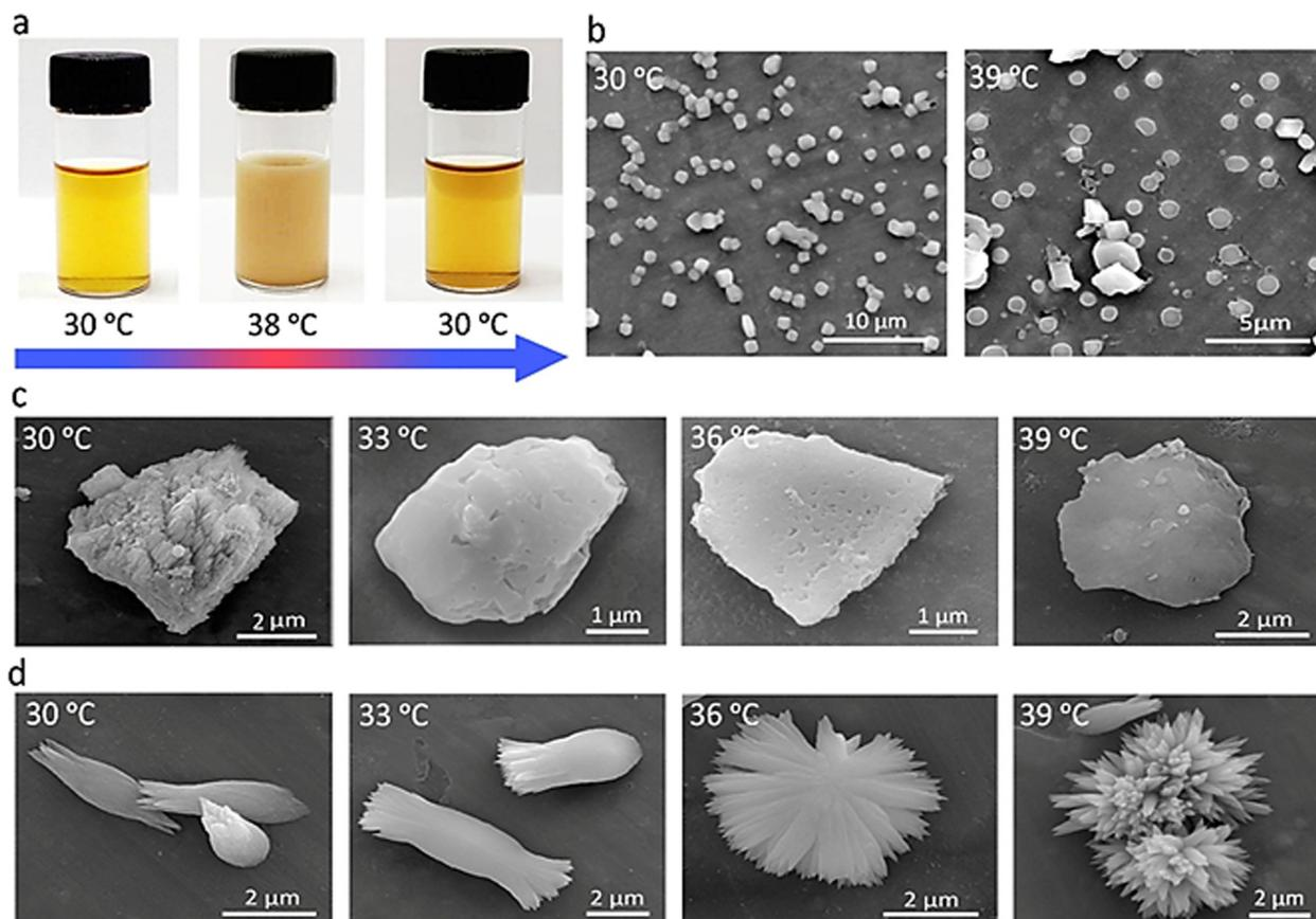
**Fig. 3** (a) LCST of PNIPAM scaffolds was in the range of 36–38 °C. The colloidal dispersions were precipitated at 39 °C after 10–15 minutes. (b) SEM images of PNIPAM1 at 30 °C and 39 °C. SEM images of PNIPAM1 (c) and PNIPAM2 (d) at different temperatures ranging from 30 °C to 39 °C.
