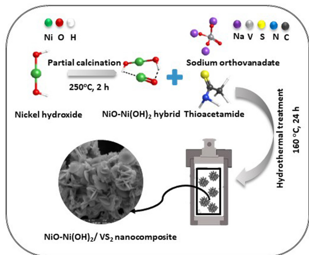
Scheme 1 The synthesis process of NiO–Ni(OH) 2 /VS 2 nanocomposite.
