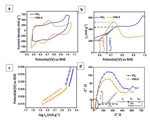
Fig. 6 (a) CVs; (b) LSV curves; (c) the relevant Tafel plots derived from LSV curves; and (d) EIS Nyquist plots of pristine VS<sub>2</sub> and VN0.8 with the corresponding equivalent circuit.
