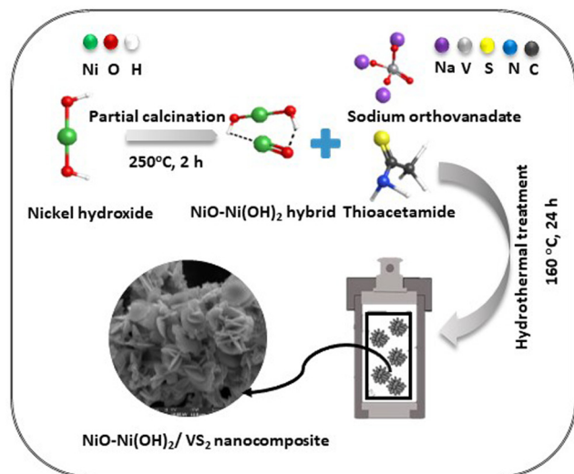
Scheme 1 The synthesis process of NiO–Ni(OH) 2 /VS 2 nanocomposite.
