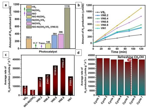
Fig. 7 (a) Comparison of photocatalytic HER over as prepared photocatalyst; (b) amount of hydrogen produced of pristine VS<sub>2</sub>, VN0.2, VN0.4, VN0.6, VN0.8 and VN1 photocatalysts; (c) average rate of photocatalytic H<sub>2</sub> production for pristine VS<sub>2</sub>, NiO-Ni(OH)<sub>2</sub>, VN0.2, VN0.4, VN0.6, VN0.8 and VN1 photocatalysts; and (d) cyclic reusability of VN0.8 under visible light irradiation under the same photocatalytic conditions.
