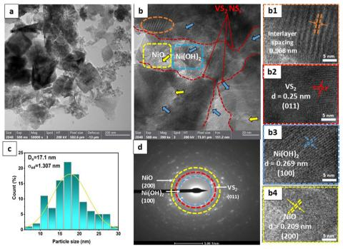
Fig. 3 (a) and (b) HR-TEM images of VN0.8 at different magnifications; highlighted regions of (b) show an interlayer spacing (b1), the lattice spacing of VS<sub>2</sub> (b2), Ni(OH)<sub>2</sub> (b3) and NiO (b4); (c) particle size distribution histogram for VN0.8, and (d) the shows the corresponding SAED pattern.
