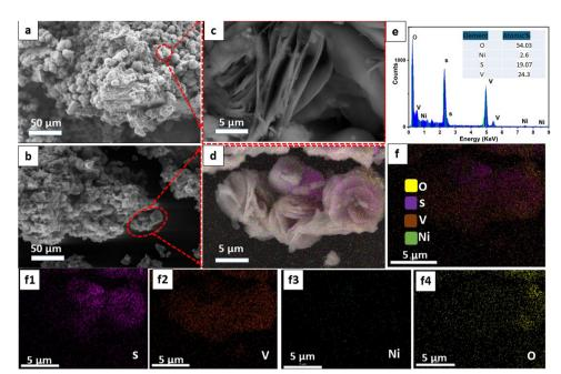
Fig. 2 (a) and (b) Low magnification SEM images of the  $VS_2$  sample and VN0.8, respectively; (c) and (d) high magnification SEM images of the  $VS_2$  sample and VN0.8, respectively; (e) EDX data of VN0.8; and (f) the corresponding EDX elemental mappings.
