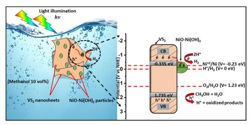
Fig. 10 Plausible photocatalytic HER mechanism on NiO-Ni(OH)<sub>2</sub>/VS<sub>2</sub> nanocomposite.
