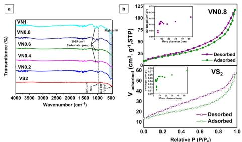
Fig. 5 (a) FT-IR spectra of the pristine and supported VS<sub>2</sub> samples, and (b) BET nitrogen adsorption and desorption isotherms of VS<sub>2</sub> and VN0.8 and pore size distributions (inset).
