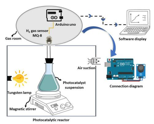
Scheme 2 The setup of the experimental apparatus for the photocatalytic H<sub>2</sub> production.
