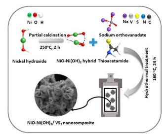
Scheme 1 The synthesis process of NiO-Ni(OH)<sub>2</sub>/VS<sub>2</sub> nanocomposite.
