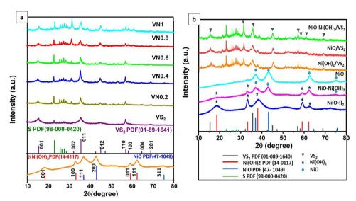
Fig. 1 XRD patterns of (a) pristine VS<sub>2</sub>, NiO-Ni(OH)<sub>2</sub> and NiO-Ni(OH)<sub>2</sub>/VS<sub>2</sub> nanocomposites; and (b) Ni-based cocatalysts and their corresponding VS<sub>2</sub> nanocomposites
