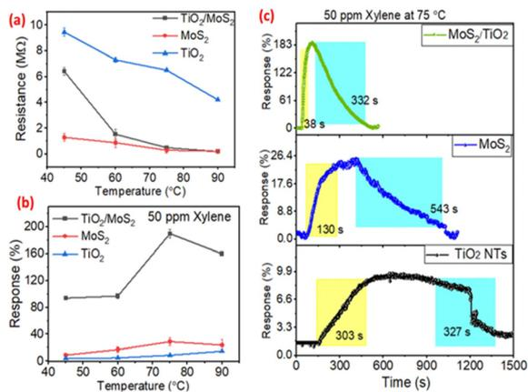
Fig. 3 (a) Baseline resistance change vs. temperature, (b) corresponding response magnitude ( $\Delta R/R_a$  in %) vs. temperature for all three sensors, and (c) response characteristics of all three sensors at optimized 75 °C temperature.
