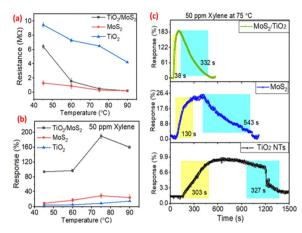
Fig. 3 (a) Baseline resistance change vs. temperature, (d) corresponding response magnitude ( $\Delta R/R_a$  in %) vs. temperature for all three sensors, and (c) response characteristics of all three sensors at optimized 75 °C temperature
