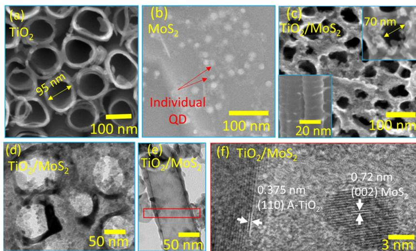
Fig. 1 SEM micrographs of (a) pure  $\text{TiO}_2$  nanotube arrays, (b)  $\text{MoS}_2$  quantum dots, and (c) a  $\text{MoS}_2/\text{TiO}_2$  composite; (d) and (e) TEM image of the  $\text{MoS}_2/\text{TiO}_2$  composite and (f) HRTEM image showing the coexistence of  $\text{TiO}_2$  and  $\text{MoS}_2$ .
