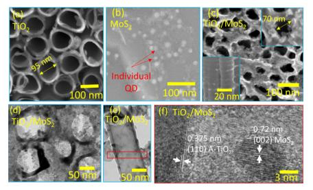
Fig. 1 SEM micrographs of (a) pure TiO2 nanotube arrays, (b) MoS2 quantum dots, and (c) a MoS2/TiO2 composite; (d) and (e) TEM image of the MoS<sub>2</sub>/TiO<sub>2</sub> composite and (f) HRTEM image showing the coexistence of TiO<sub>2</sub> and MoS<sub>2</sub>.
