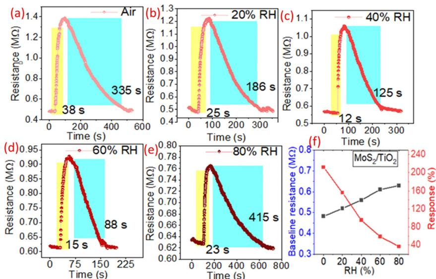
Fig. 5 (a–e)  $\text{MoS}_2/\text{TiO}_2$  sensor resistance variation with different relative humidity levels (air, 20–80% RH) at a fixed xylene concentration of 50 ppm at 75 °C and (f) change in the baseline resistance and response magnitude (%) of the  $\text{MoS}_2/\text{TiO}_2$  sensor at different humidity levels.
