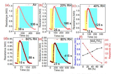
Fig. 5 (a–e)  $MoS_2/TiO_2$  sensor resistance variation with different relative humidity levels (air, 20–80% RH) at a fixed xylene concentration of 50 ppm at 75 °C and (f) change in the baseline resistance and response magnitude (%) of the  $MoS_2/TiO_2$  sensor at different humidity levels.
