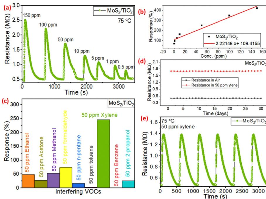
Fig. 4 (a)  $\text{MoS}_2/\text{TiO}_2$  nanotube sensor resistance change for different xylene concentrations (in ppm). (b) Corresponding absolute response magnitude vs. xylene concentration (in ppm). (c) Selectivity study of xylene over other interfering VOCs, (d) long-term stability study of the sensor for 30 days with an interval of 1 day, and (e) repeatability test for six continuous cycles at a 50 ppm concentration. All measurements were performed at an optimized temperature of 75 °C.
