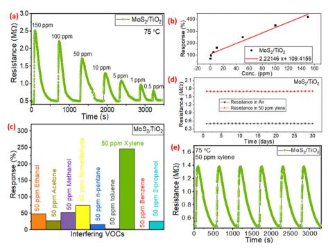
Fig. 4 (a)  $MoS_2/TiO_2$  nanotube sensor resistance change for different xylene concentrations (in ppm). (b) Corresponding absolute response magnitude vs. xylene concentration (in ppm). (c) Selectivity study of xylene over other interfering VOCs, (d) long-term stability study of the sensor for 30 days with an interval of 1 day, and (e) repeatability test for six continuous cycles at a 50 ppm concentration. All measurements were performed at an optimized temperature of 75 °C.
