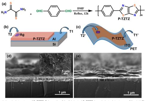
Fig. 1 (a) Synthesis and chemical structure of P-TZTZ. Schematic of the fabricated P-TZTZ-based photodetectors on (b) a rigid Si substrate (PD1) and (c) on a flexible ITO-coated PET substrate (PD2). Cross-sectional HR-SEM images of (d) PD1 and (e) PD2. The inset of (d) shows uniform deposition of the synthesized polymer.
