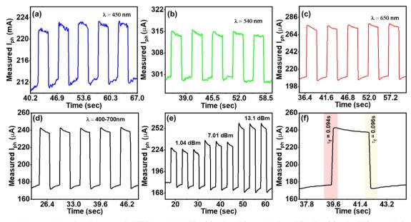
Fig. 5 Temporal characteristics of the fabricated P-TZTZ-based rigid PD1: (a) at  $\lambda = 450$  nm with  $P_{in} = 3.01$  dBm, (b) at  $\lambda = 540$  nm with  $P_{in} = 3.89$  dBm, and (c) at  $\lambda = 650$  nm with  $P_{in} = 5.11$  dBm, (d) broadband white light source, (e) with varying  $P_{in}$  for broadband white light source and (f) transient performance
