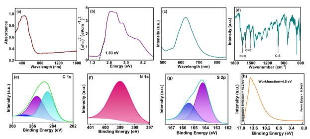
Fig. 2 Material characterization of the synthesized P-TZTZ: (a) the solid-state UV-vis and (b) emission spectra of the P-TZTZ polymer, (c) Tauc plot indicating  $E_q$ , (d) FTIR spectra, (e) XPS core level scan of the C 1s, (f) N 1s and (g) S 2p, and (h) UPS spectra showing the work function of the synthesized P-TZTZ.
