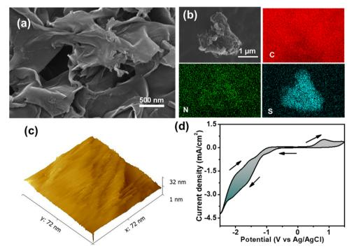
Fig. 3 (a) The FESEM image of the P-TZTZ polymer. (b) The EDX elemental mapping of the polymer. (c) STM image and (d) cyclic voltammogram of the P-TZTZ film on GCE.
