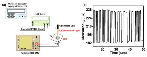
Fig. 8 Application of the fabricated PDs in visible lightwave communication: (a) experimental setup and (b) detected PRBS pattern measured using a Keithley 2450 SMU
