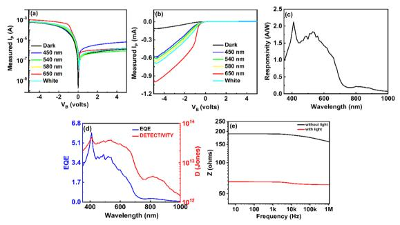
Fig. 4 Electrical characterization of fabricated PD: measured I-V characteristics of PD1 in (a) the logarithmic scale and (b) the linear scale. (c) Measured R in the 380 nm to 1000 nm range. (d) Measured EQE and calculated D values in the 380 nm to 1000 nm range. (e) Impedance analysis of PD1.
