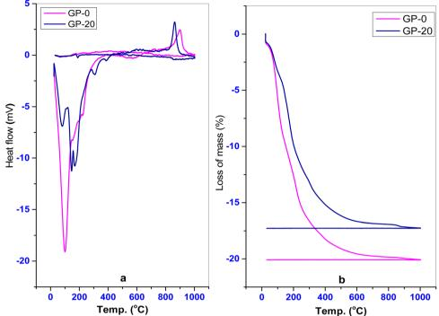
Fig. 6 (a) Differential thermal analysis, DTA and (b) thermogravimetric analysis, TGA of GP-0 and GP-20
