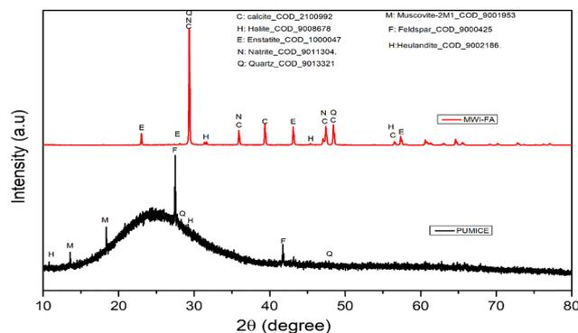
Fig. 3 XRD diffractogram of MWI-FA and pumice.
