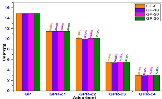
Fig. 16 Four-cycle recyclability potential of the geopolymers.
