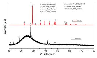
Fig. 3 XRD diffractogram of MWI-FA and pumice.
