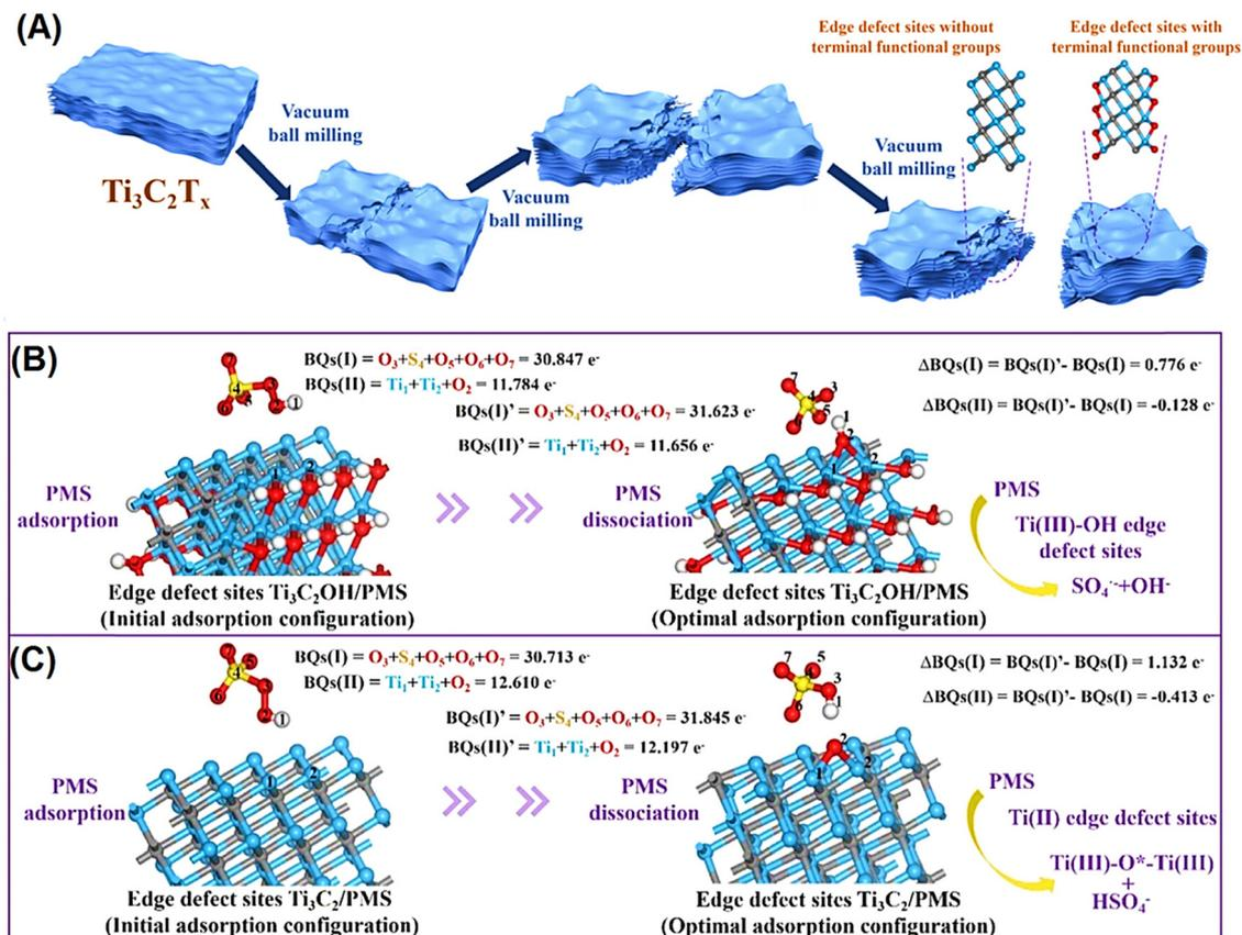
Fig. 6 (A) A visual representation showing the synthetic pathway for a bulk MXene ( $\text{Ti}_3\text{C}_2\text{T}_x$ ) and edge-rich defective  $\text{Ti}_3\text{C}_2\text{T}_x$  is presented. (B) The (010)  $\text{Ti}_3\text{C}_2\text{OH}/\text{peroxymonosulfate}$  (PMS) system along with its corresponding Bader charge. (C) The (010)  $\text{Ti}_3\text{C}_2/\text{PMS}$  system and its corresponding Bader charge. Reproduced with permission from ref. 83. Copyright 2023 American Chemical Society.
