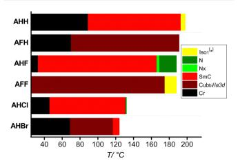
Fig. 1 Phase transitions of AXY compounds as observed on 2nd cooling at a rate of 10 K min<sup>-1</sup>.
