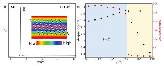
Fig. 4 (a) SAXS diffractograms of the SmC phase for AHF at 128 °C and (b) temperature dependence of d-spacing and coherence of AHF upon heating
