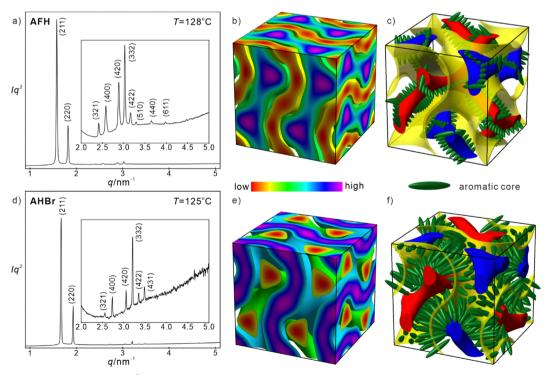
Fig. 3 SAXS diffractograms of the Cub<sub>b</sub>/ $Ia\bar{3}d$  phase for (a) **AFH** at 128 °C and (d) **AHBr** at 125 °C; (b) and (e) the reconstructed ED maps for two compounds, high ED is in purple and low ED is in red; and (c) and (f) the schematic model of molecular packing for two compounds.
