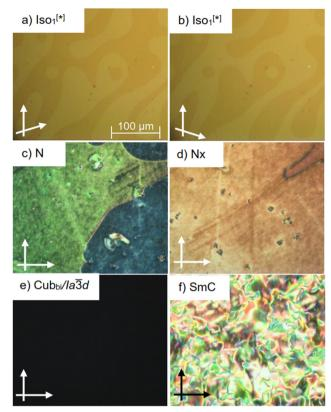
Fig. 2 Optical micrographs on cooling for: (a) and (b) the chiral  $Iso_1^{[\star]}$ phase at 185 °C of compound AFF under slightly uncrossed polarizers either in a clockwise or in an anticlockwise direction (see white arrows): (c) the N phase of compound AHF at 183 °C; (d) the N<sub>x</sub> phase of compound AHF at 168 °C; (e) the double-gyroid achiral Cub<sub>bi</sub>/la3d phase of compound AFH at 90 °C and (f) the schlieren texture in the SmC phase of compound AHF at 140 °C.
