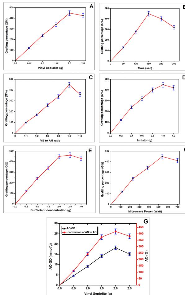
Fig. 1 Effect of different reaction parameters on grafting percentage of AN-PB onto VS. (A) Effect of substrate on  $G\%$ , (B) effect of exposure time on  $G\%$ , (C) effect of VS to AN ratio on  $G\%$ , (D) effect of initiator on  $G\%$ , (E) effect of surfactant on  $G\%$ , (F) effect of microwave irradiation power on  $G\%$ , and (G) effect of VS on AO-GD and AO%.
