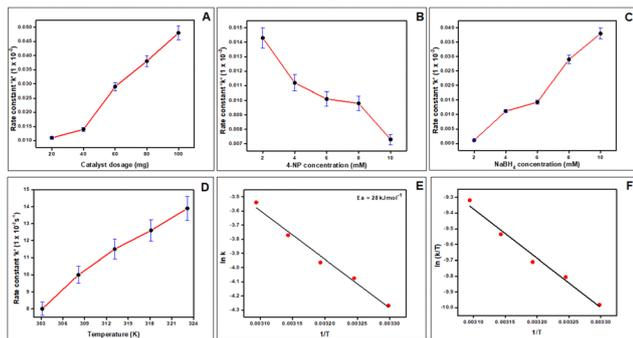
Fig. 7 Detailed UV study of various reaction parameters, (A) effect of catalyst dose on rate constant, (B) effect of 4-NP conc. on rate constant, (C) effect of NaBH<sub>4</sub> conc. on rate constant, (D) effect of temperature on rate constant, (E) Arrhenius plot, here  $1/T$  is plotted vs.  $\ln k$  and activation energy is calculated from slope of the line, (F) plot of  $1/T$  versus  $\ln(k/T)$  to calculate thermodynamic parameters:  $\Delta H$ ,  $\Delta S$  and  $\Delta G$ .
