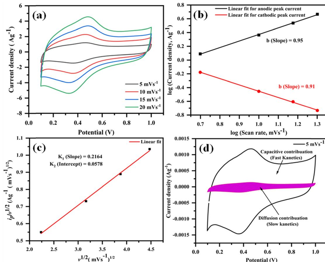
Fig. 12 The anodic and cathodic peaks at low scan rates as illustrated by CV plots (5–20  $\text{mV s}^{-1}$ ) (a); plot of  $\log i_p$  vs.  $\log v$  for (b); the peak current  $(i_p)/(\text{scan rate})^{1/2}(v)^{1/2}$  vs.  $(v)^{1/2}$  plot (c); plot of capacitive contribution to the total current in CV curve of  $\text{rGO}/\text{Cu}(\text{II})$  at  $5 \text{ mV s}^{-1}$  (d).
