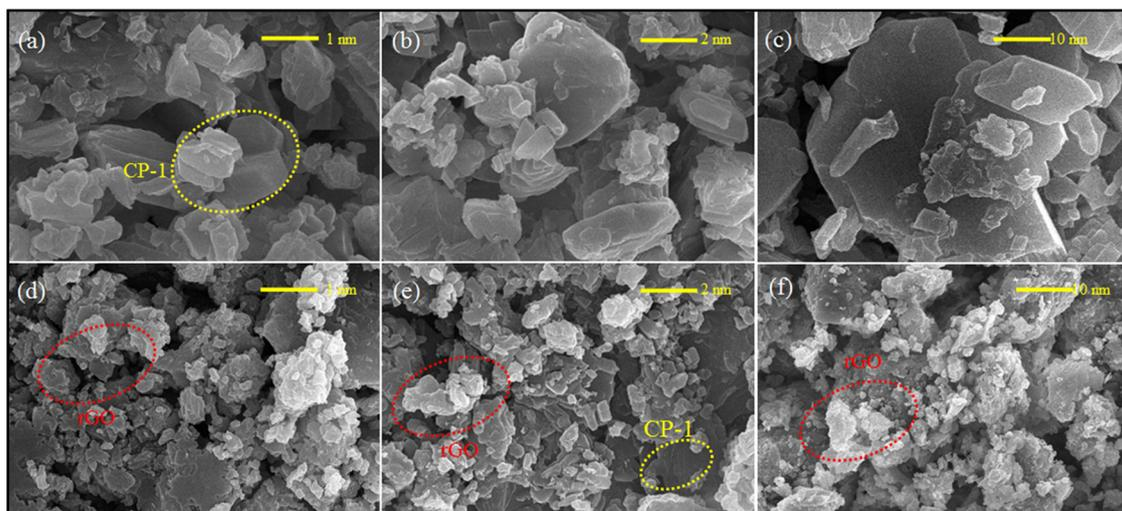
Fig. 2 SEM images of the prepared **CP-1** showing the particle morphology at different magnification ranges (a)–(c), images of the **rGO@CP-1** composite represent the adhering of **rGO** on **CP-1** at different magnification ranges (d) and (e), and surface morphological behavior of **CP-1** and **rGO@CP-1** were executed within the 1–10 nm scale range. (yellow circles represent **CP-1** particles and red circles for **rGO**).
