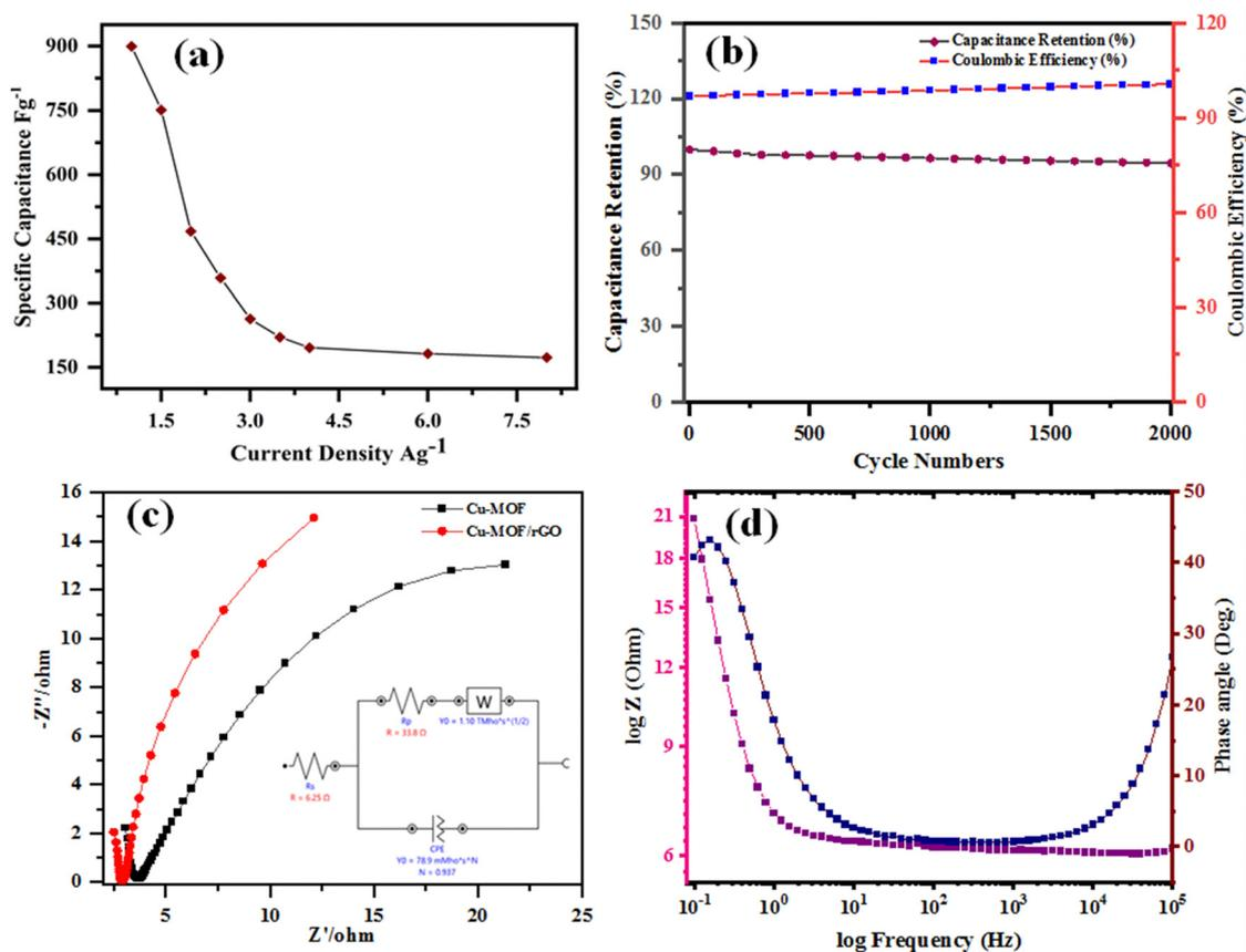
Fig. 11 (a) Specific capacitance vs. current density for the composite electrode, (b) cycling stability profile of CP-1 and the composite electrode up to 2000 cycles at a current density of 8.0 A  $\text{g}^{-1}$ , (c) Nyquist plots of CP-1 and rGO@CP-1 electrode materials with the inset showing the equivalent circuit of the composite, and (d) Bode plot of rGO@CP-1 electrode.
