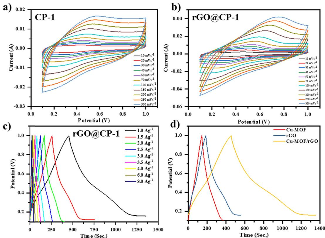
Fig. 10 (a) and (b) CV curve profile of **CP-1** and the composite (**rGO@CP-1**), and (c) GCD profile of the composite (**rGO@CP-1**) at different current densities, and (d) comparative GCD profile of **CP-1**, **rGO**, and the composite material at a current density of  $1.0 \text{ A g}^{-1}$ .
