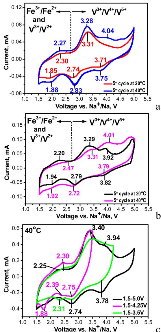
Fig. 3 CV curves in sodium-half cells at a scanning rate of 0.1 mV s<sup>-1</sup> for NFVPS/C (a) and NFVPS/rGO (b) at 20 and 40 °C within a voltage window of 1.5–5.0 V; CV curves at a scanning rate of 1 mV s<sup>-1</sup> for NFVPS/C at 40 °C within different voltage windows (c).
