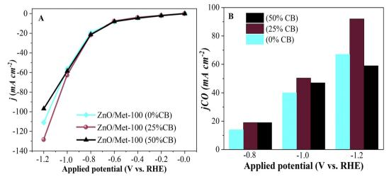
Fig. 10 (A) Electrochemical polarization curve of the ZnO/Met-31 µL treated electrode with variations in carbon black concentrations at different applied potentials. (B) Partial current density at different applied potentials
