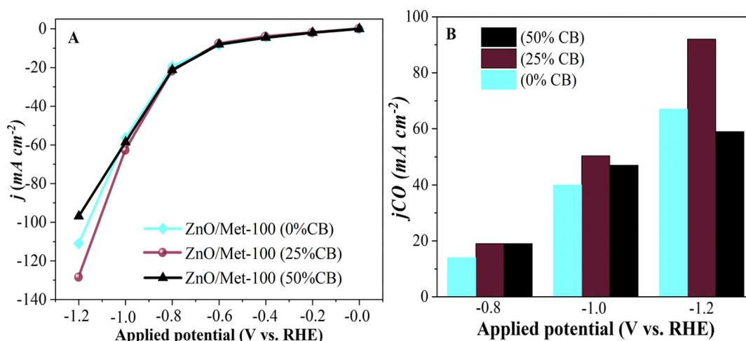
Fig. 10 (A) Electrochemical polarization curve of the  $\text{ZnO/Met-31 } \mu\text{L}$  treated electrode with variations in carbon black concentrations at different applied potentials. (B) Partial current density at different applied potentials.
