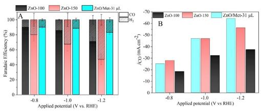
Fig. 7 (A) Faradaic efficiency obtained in a continuous flow of CO<sub>2</sub> and 0.5 M of KOH applying the potential during 20 min for the ZnO electrode (0.2 mg cm<sup>-2</sup>) in carbon black (50% catalyst/C), (B) partial current density for CO formation.
