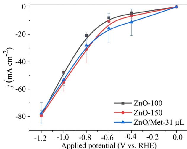
Fig. 6 Polarization curves obtained in the electrochemical flow cell with  $30 \text{ mL min}^{-1}$  of  $\text{CO}_2$  and  $5 \text{ mL min}^{-1}$  of  $\text{KOH}$  (0.5 M), applying the potential during 100 s for the ZnO electrode ( $0.2 \text{ mg cm}^{-2}$ ) in carbon black (50% catalyst/C).
