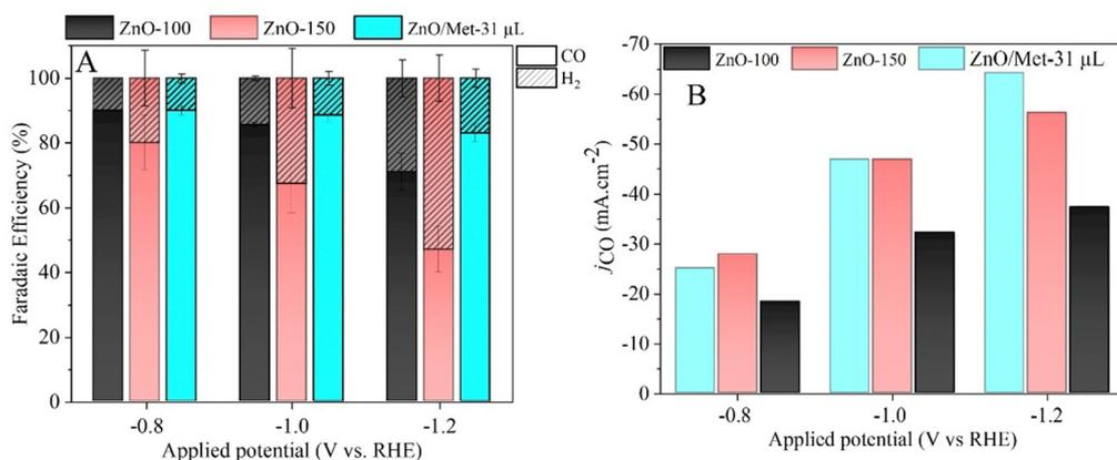
Fig. 7 (A) Faradaic efficiency obtained in a continuous flow of  $\text{CO}_2$  and 0.5 M of KOH applying the potential during 20 min for the ZnO electrode ( $0.2 \text{ mg cm}^{-2}$ ) in carbon black (50% catalyst/C), (B) partial current density for CO formation.
