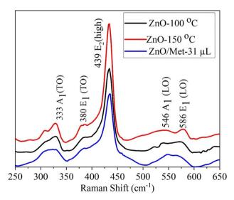
Fig. 3 Raman spectra of ZnO samples prepared by hydrothermal process.
