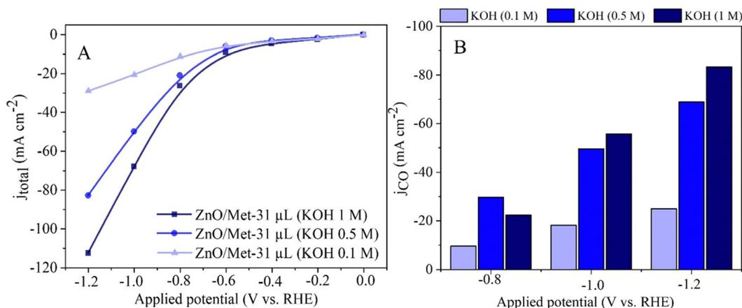
Fig. 8 (A) Polarization curves of the ZnO/Met-31  $\mu\text{L}$  under different concentrations of KOH electrolyte. (B) The partial current density for CO ( $J_{CO}$ ) formation in different concentrations of KOH.
