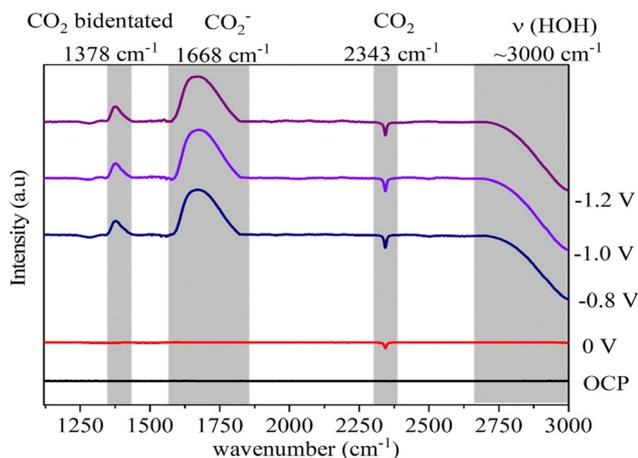
Fig. 11 *In situ* FTIR spectra of electrochemical reduction of CO<sub>2</sub> on ZnO electrode treated with monoethanolamine at different potentials.
