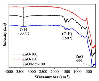
Fig. 2 FTIR spectra of the ZnO samples prepared at different temperatures (100, 150  $^{\circ}\text{C}$  and ZnO/Met-31  $\mu\text{L}).$
