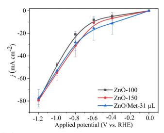
Fig. 6 Polarization curves obtained in the electrochemical flow cell with 30 mL min $^{-1}$  of CO $_2$  and 5 mL min $^{-1}$  of KOH (0.5 M), applying the potential during 100 s for the ZnO electrode (0.2 mg cm $^{-2}$ ) in carbon black (50% catalyst/C).
