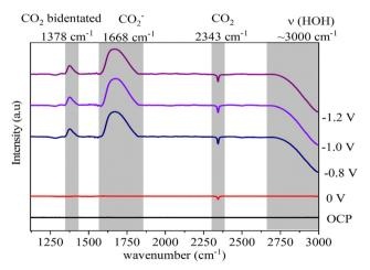
Fig. 11 In situ FTIR spectra of electrochemical reduction of CO<sub>2</sub> on ZnO electrode treated with monoethanolamine at different potentials.
