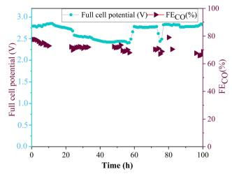
Fig. 12 Long-term stability of ZnO/Met-31 μL GDE by applying a current of -50 mA cm<sup>-2</sup> during 100 h of reaction.
