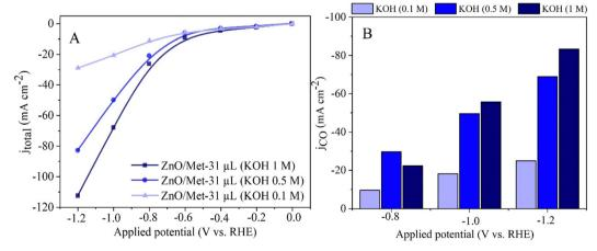
Fig. 8 (A) Polarization curves of the ZnO/Met-31 µL under different concentrations of KOH electrolyte. (B) The partial current density for CO (J<sub>CO</sub>) formation in different concentrations of KOH.
