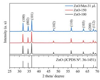
Fig. 1 XRD patterns of the ZnO samples prepared at different temperatures (100, 150 °C and ZnO/Met-31  $\mu$ L).
