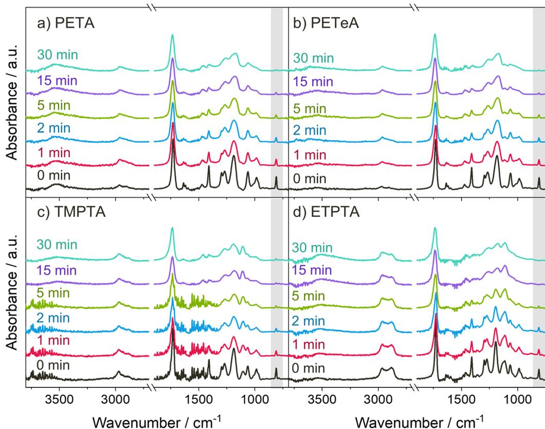
Fig. 1 UV polymerization of the acrylate monomers. (a)–(d) FTIR spectra of the monomer thin films after different UV exposure times. The peak highlighted in gray corresponds to the  $=\text{C}-\text{H}$  bending at  $810\text{ cm}^{-1}$  used for calculation of the degree of polymerization (see Fig. 2).
