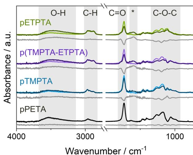
Fig. 4 FTIR spectra of crosslinked acrylate films before (light color) and after (dark color) VPI with a 15-hour DEZ hold at  $120\text{ }^{\circ}\text{C}$ . The difference spectra are shown as gray lines. Relevant absorption bands are highlighted in gray. \*marks a new peak that appears upon reaction with DEZ. pPETA was UV-polymerized for 5 min, pTMPTA, p(TMPTA-ETPTA) and pETPTA for 10 min.
