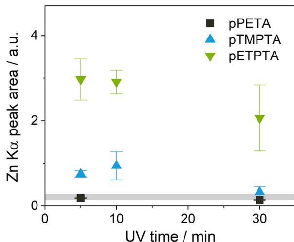
Fig. 3 Zn loading of crosslinked acrylate films with different UV exposure times after VPI at  $120\text{ }^{\circ}\text{C}$  with a 15-hour DEZ hold based on the XRF Zn  $K\alpha$  peak area. The gray area indicates the average Zn loading of a Si wafer subjected to the same VPI process.
