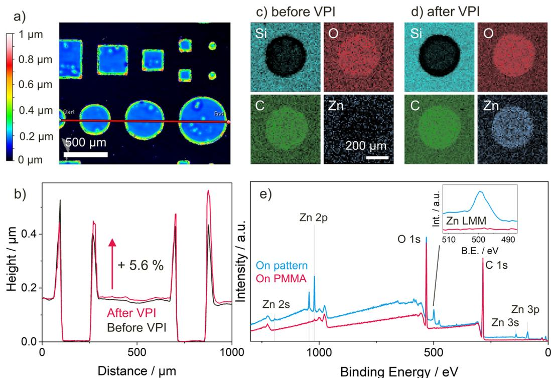
**Fig. 6** Selective Zn infiltration (5 h DEZ, 120 °C) of a p(TMPTA-ETPTA) pattern on PMMA. (a) Optical Profilometry of the pattern before VPI, (b) height profile before and after VPI cut along pink line in (a), (c) and (d) EDX elemental maps of a p(TMPTA-ETPTA) feature on PMMA (c) before and (d) after VPI. (e) XPS survey scan of samples on the p(TMPTA-ETPTA) pattern and on PMMA after VPI. The inset shows a zoom on the Zn  $L_{3M_{4.5}M_{4.5}}$  Auger peak.
