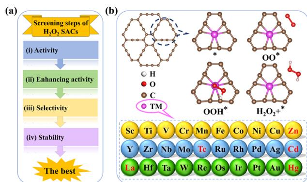
Fig. 1 (a) Schematic diagram of screening H<sub>2</sub>O<sub>2</sub> SACs. (b) 2e<sup>−</sup> ORR pathways on TM–GY.
