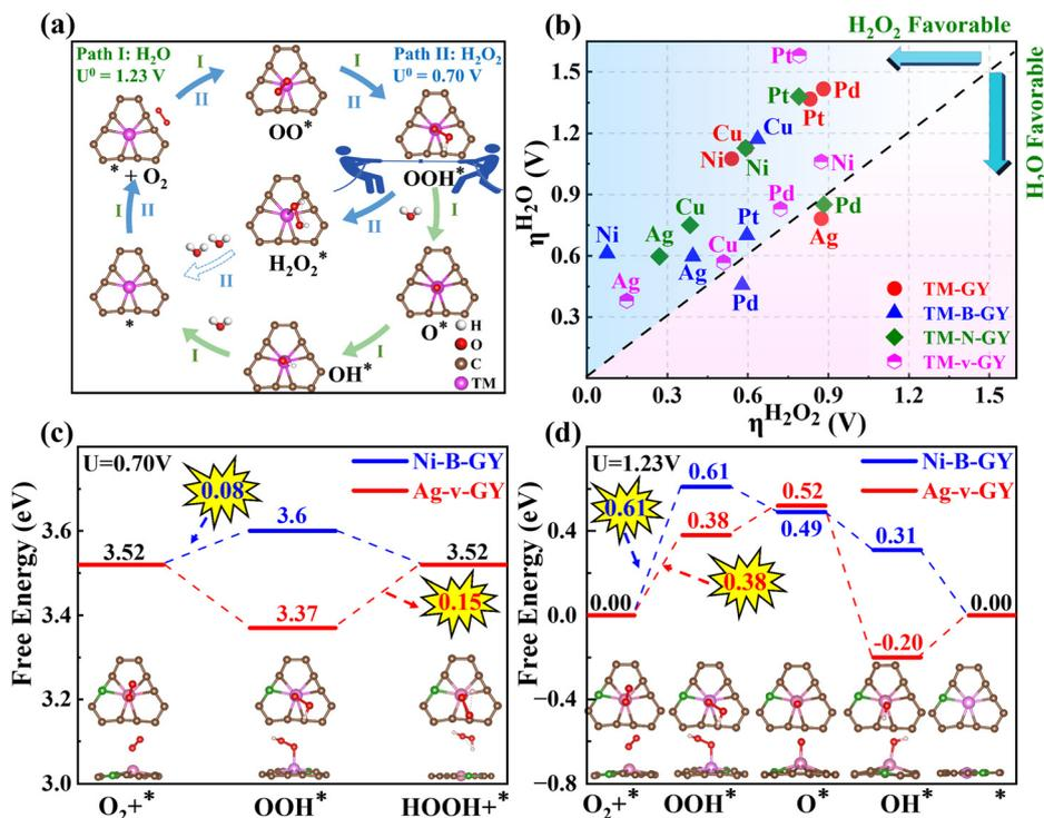
Fig. 4 The selectivity of TM-NM-GY catalysts: (a) Schematic illustration of the 2e<sup>-</sup> and 4e<sup>-</sup> ORR pathways. (b) Overpotential for 2e<sup>-</sup> and 4e<sup>-</sup> ORR. (c) and (d) Free energy diagrams comparing 2e<sup>-</sup> and 4e<sup>-</sup> ORR for Ag-v-GY and Ni-B-GY, highlighting their superior catalytic activity.
