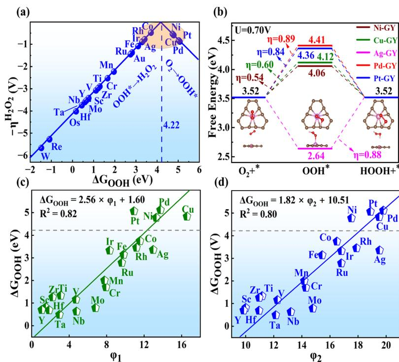
Fig. 2 (a) The volcano plot of  $\Delta G_{OOH}$  and the overpotential. (b) Free energy diagram for  $2e^-$  ORR on TM-GY candidates (TM = Ni, Cu, Ag, Pd and Pt). (c) and (d) The scaling relationship between  $\Delta G_{OOH}$  and  $\phi_1$ ,  $\phi_2$  for TM-GY.
