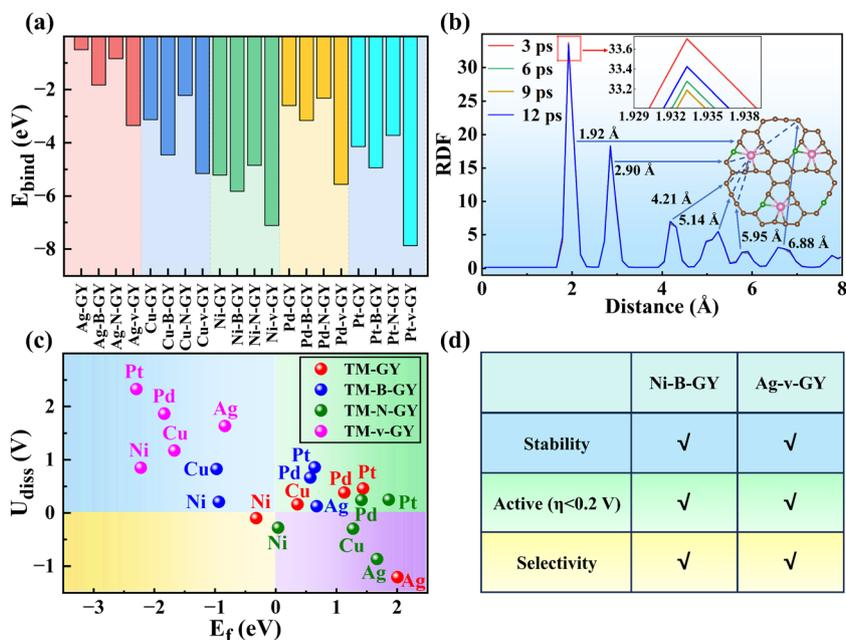
Fig. 5 The stability of TM-NM-GY catalysts: (a) Binding energy ( $E_{\text{bind}}$ ). (b) The RDF between the Ni and C for Ni-B-GY at 300 K and the configuration at 12 ps. (c) Dissolution potentials ( $U_{\text{diss}}$ ) and formation energies ( $E_f$ ). (d) The performances of Ni-B-GY and Ag-v-GY.
