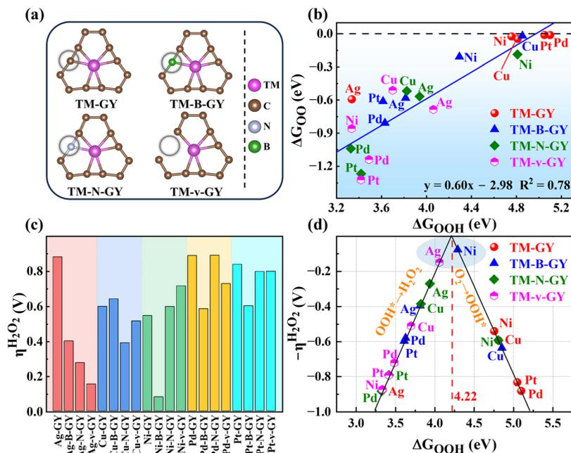
Fig. 3 (a) The configuration of TM-NM-GY (NM = B, N doping or C vacancy). (b) The linear relationship between  $\Delta G_{OOH}$  and  $\Delta G_{OO}$ . (c) The  $\eta_{H_2O_2}$  for TM-NM-GY. (d) Volcano plot of  $\Delta G_{OOH}$  as a function of overpotential  $\eta_{H_2O_2}$ .
