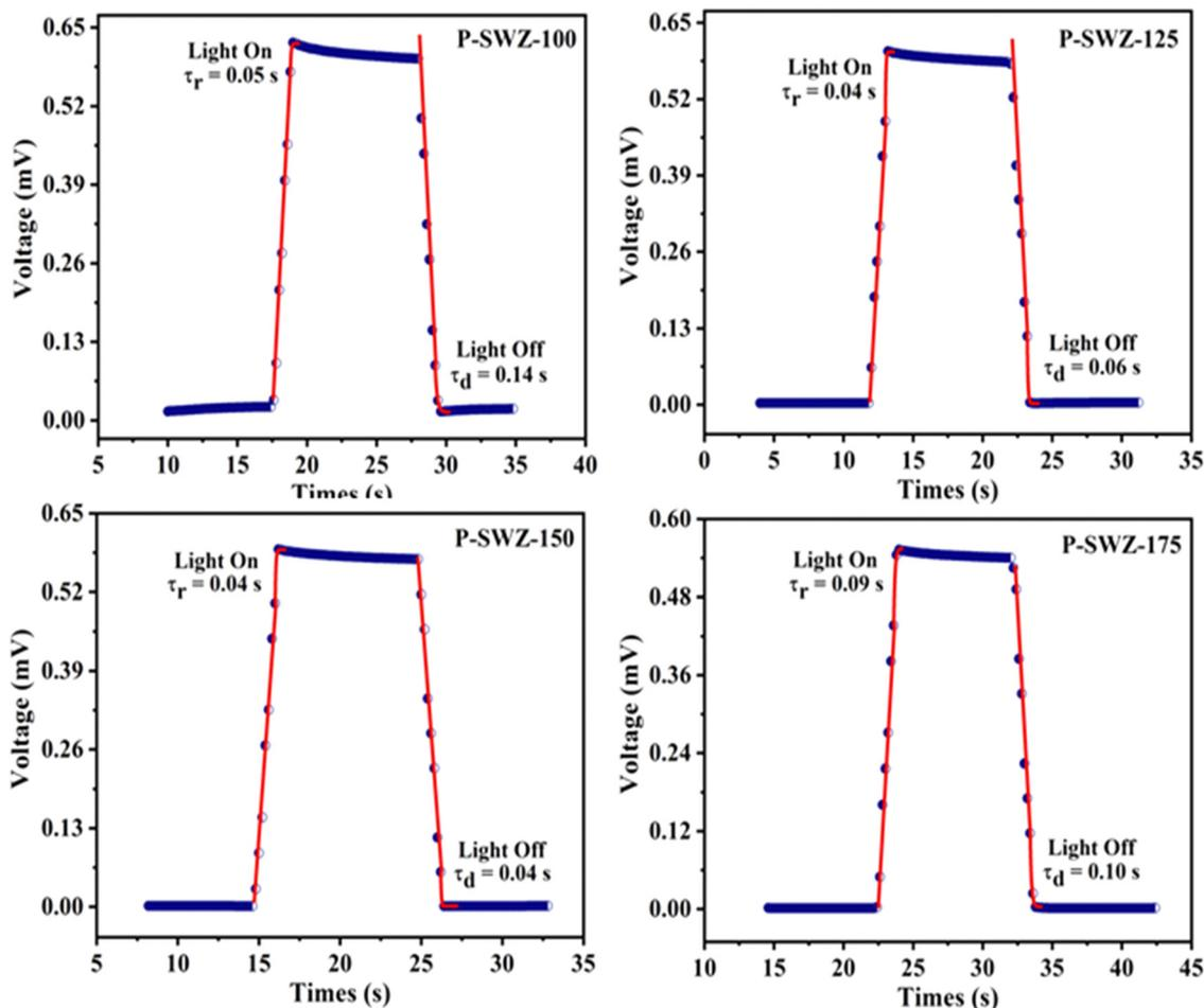
Fig. 11 Photoresponse voltage fitting SWCNT/ZnO NCs on the Si thin film.
