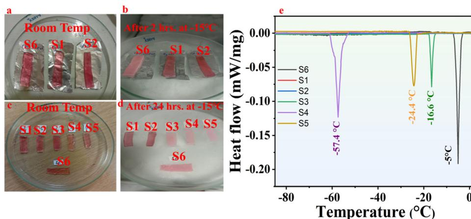
Fig. 2 Photographs showing anti-freezing characteristics of the hydrogels and organohydrogels at  $-15\text{ }^{\circ}\text{C}$ . (a) Room temperature photographs of samples S1, S2 and S6, (b) S1, S2 and S3 after storing for two hours at  $-15\text{ }^{\circ}\text{C}$ , (c) S1–S6 at room temperature and (d) S1–S6 after storing for 24 hours at  $-15\text{ }^{\circ}\text{C}$ . (e) DSC curves.
