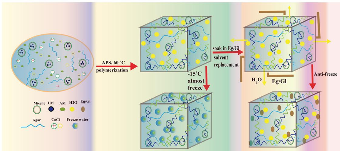
Fig. 1 Diagram showing the polymerization and subsequently simple USRS used to create anti-freezing DN organohydrogels from DN hydrogels. At  $-15\text{ }^{\circ}\text{C}$ , the DN hydrogels solidified; however, the Eg and Gl anti-freezing organohydrogels retained their elasticity even at such low temperatures.
