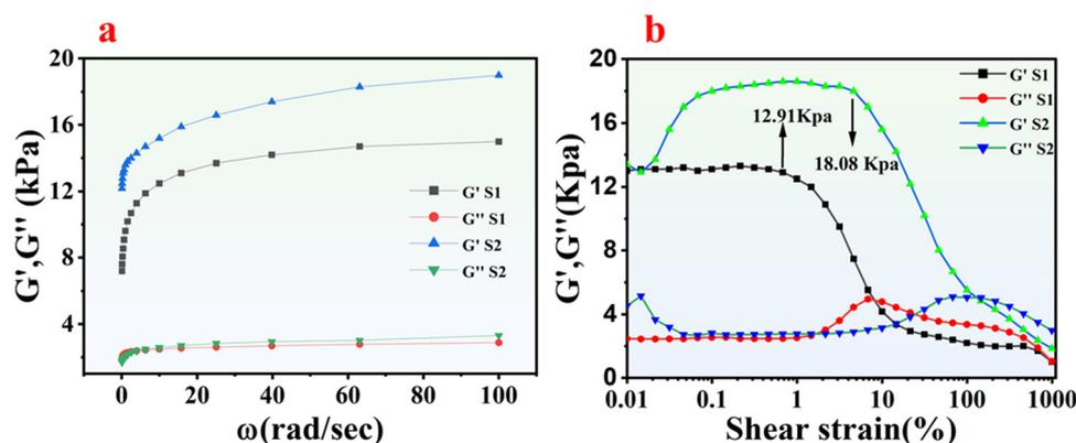
Fig. 5 The rheological investigation of the samples S1 and S2. (a) The frequency sweep test between 0.1 to 100  $\text{rad s}^{-1}$ , (b) the amplitude sweep study performed for strains ranging from 0.01 to 1000% at constant frequency of 10  $\text{rad s}^{-1}$ .
