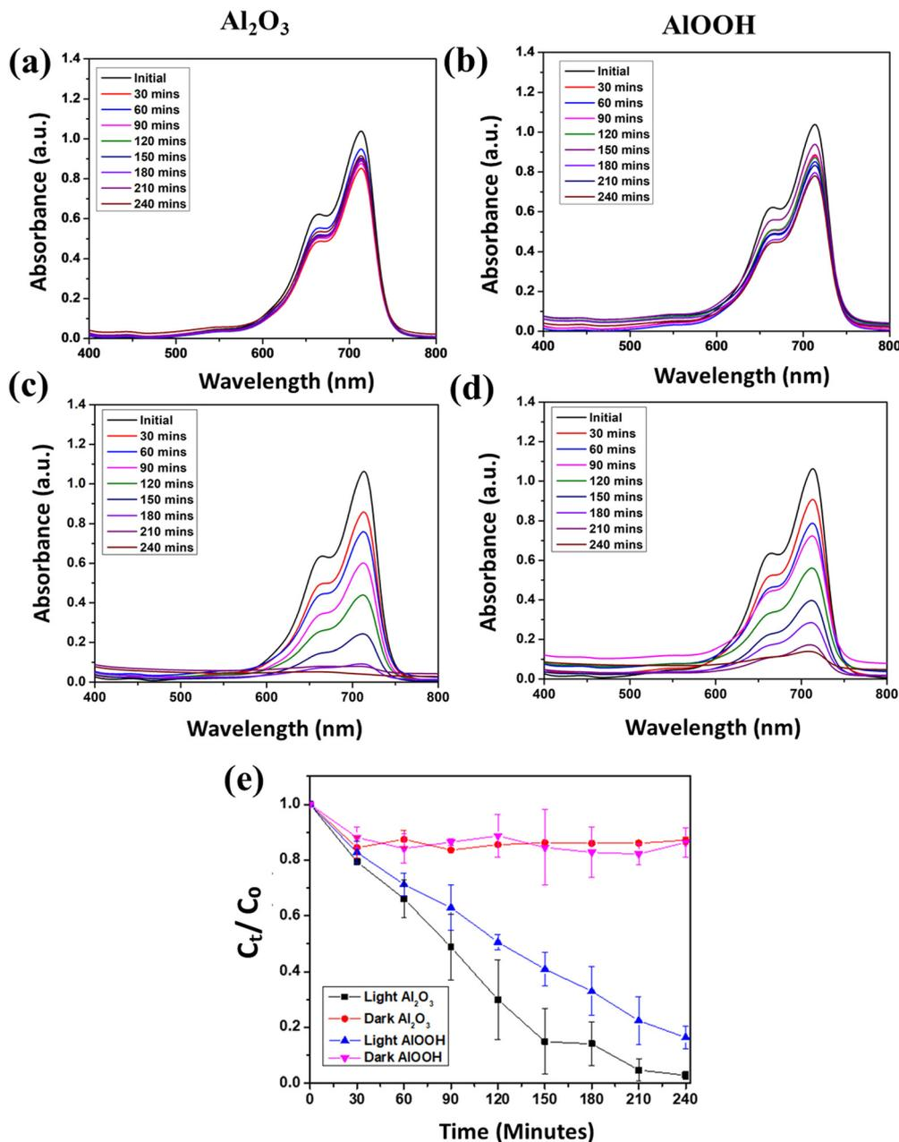
Fig. 7 UV-vis spectra of MB with  $\text{Al}_2\text{O}_3$  (a) and  $\text{AlOOH}$  (b) in the dark and  $\text{Al}_2\text{O}_3$  (c) and  $\text{AlOOH}$  (d) in the light at pH 5. Average degradation efficiency over time at pH 5 (e).
