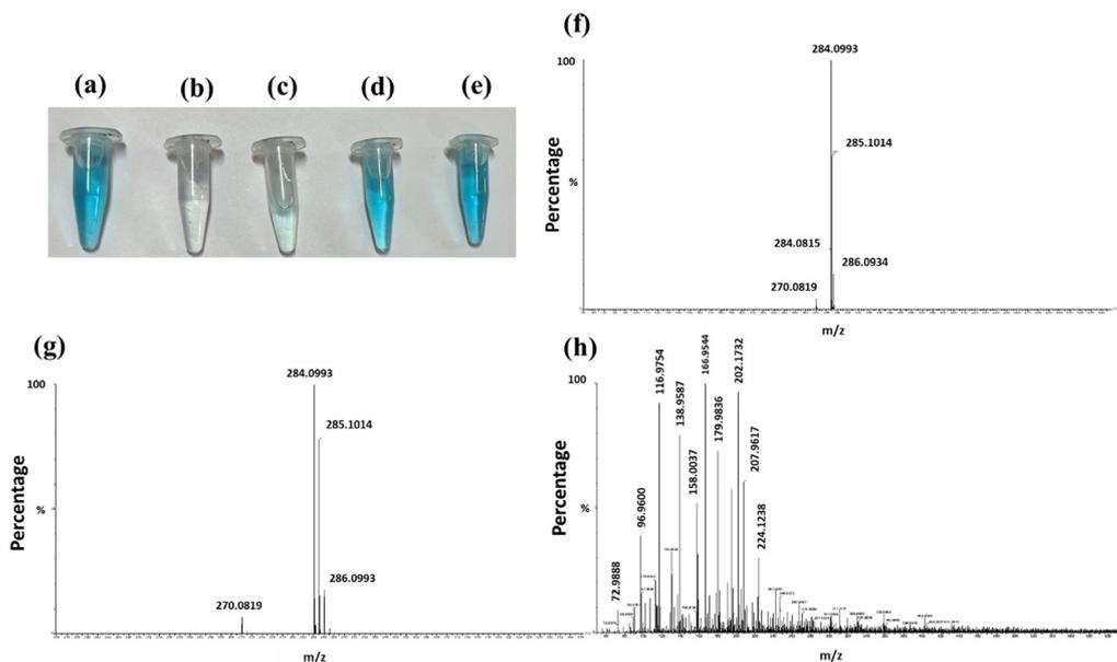
Fig. 8 Samples of MB: (a) initial, (b) with  $\text{Al}_2\text{O}_3$  in the light after 240 min, (c) with  $\text{AlOOH}$  in the light after 240 min, (d) with  $\text{Al}_2\text{O}_3$  in the dark after 240 min, and (e) with  $\text{AlOOH}$  in the dark 240 min. Mass spectra of MB: (f) initial, (g) 240 min in the dark, and (h) 240 min in the light.
