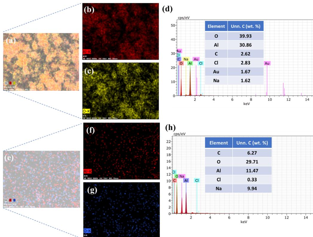
Fig. 4 Mapping of  $\text{Al}_2\text{O}_3$  (a)–(c) and EDX of  $\text{Al}_2\text{O}_3$  (d). Mapping of  $\text{AlOOH}$  (e)–(g) and EDX of  $\text{AlOOH}$  (h).
