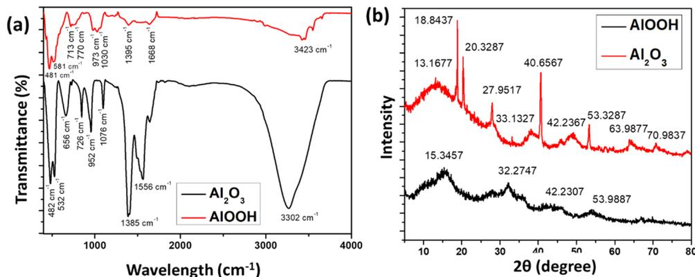
Fig. 2 FTIR (a) of Al<sub>2</sub>O<sub>3</sub> (black) and ALOOH (red). XRD (b) of Al<sub>2</sub>O<sub>3</sub> (red) and ALOOH (black).
