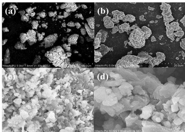
Fig. 3 FE-SEM of  $\text{Al}_2\text{O}_3$  (a) and (b) particles at scales of 40.0  $\mu\text{m}$  and 20.0  $\mu\text{m}$ , respectively. FESEM of  $\text{AlOOH}$  (c) and (d) particles at scales of 4.0  $\mu\text{m}$  and 1.0  $\mu\text{m}$ , respectively.
