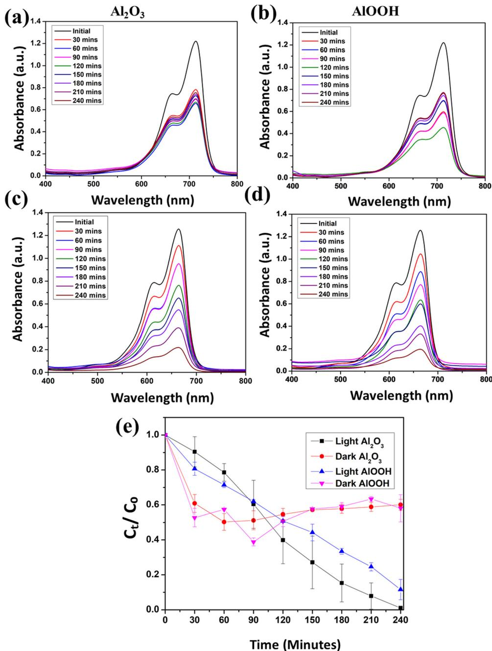
Fig. 6 UV-vis spectra of MB with  $\text{Al}_2\text{O}_3$  (a) and  $\text{AlOOH}$  (b) in the dark and  $\text{Al}_2\text{O}_3$  (c) and  $\text{AlOOH}$  (d) in the light at pH 9. Average degradation efficiency over time at pH 9 (e).
