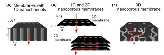
Fig. 2 Illustrations of the solid-state membrane film structures included in our review: (a) 1D nanochannels with a longer channel length (or film thickness, t) than the diameter (d) of the nanopores; (b) 2D membrane thin films with 1D nanopores where d > t or the stacks of such 1D membranes (called 2D membranes); (c) 3D nanoporous membranes with irregularly connected nanopores.
