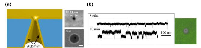
Fig. 8 (a) Schematic illustration of uniform ALD coating on a single conical nanochannel and SEM images of the tip and base sides. The scale bar is 100 nm. Reprinted with permission from ref. 279 Copyright 2015, American Chemical Society. (b) (Left) Resistive pulse signals of a 1:1 mixture of 22 b ss-DNA and ds-DNA after 5 min and 10 min. (Right) STED super-resolution microcopy image at 30 min. Reprinted from ref. 280 with the permission of AIP Publishing
