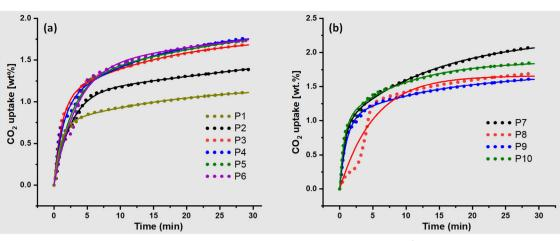
Fig. 2 TGA profiles of adsorption of CO<sub>2</sub>; (a) effect of size and (b) effect of shape at 25 °C, 50 ml min<sup>-1</sup>, 15% CO<sub>2</sub> in N<sub>2</sub>. The solid line represents the pseudo-first-order fitting.
