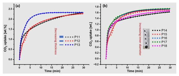
Fig. 3 (a) Effect of thickness of flakes' on the CO<sub>2</sub> adsorption capacity and kinetics. (b) Effect of pellets' inner diameter size (cylindrical) on the adsorption capacity and kinetics.
