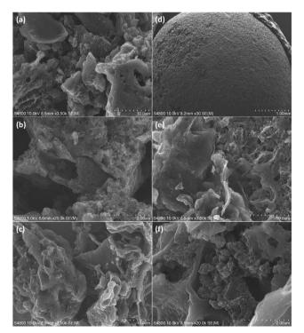
Fig. 1 (a)–(c) SEM images of activated carbon (powder). (d)–(f) SEM image of pellets (P3).
