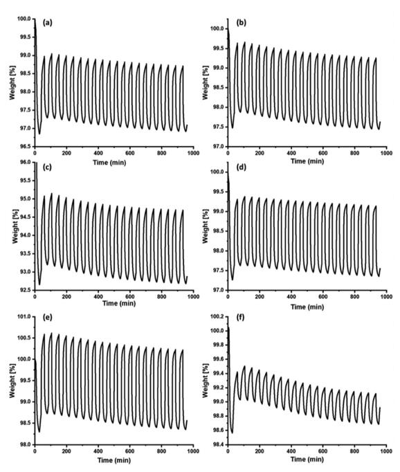
Fig. 5 20 cycles of CO<sub>2</sub> adsorption-desorption of porous carbon pellets. (a) P4, (b) P6, (c) P7, (d) P9, (e) P10. (f) Cyclic N<sub>2</sub> adsorption-desorption of the P7 pellet.
