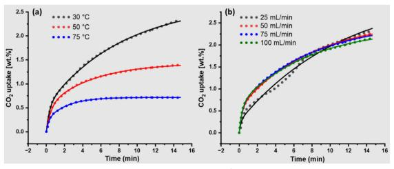
Fig. 4 (a) Effect of adsorption temperature at a fixed  $CO_2$  flow rate of 50 ml min<sup>-1</sup>. (b) Effect of different flow rates of  $CO_2$  at a fixed adsorption temperature (30 °C).
