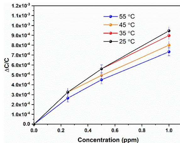
Fig. 4 NOTT (Al) 300 MOF sensor response under various NO<sub>2</sub> concentrations as a function of the working temperature.
