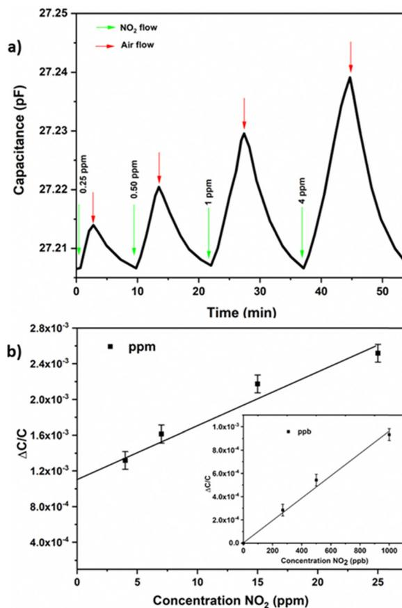
Fig. 2 (a) Dynamic response–recovery curve of the NOTT-300 (Al) MOF sensor to different concentrations of NO<sub>2</sub>. (b) The detection of NO<sub>2</sub> in different concentration ranges: 250 ppb–4 ppm and (inset) 250–1000 ppb linear response for the corresponding range.
