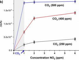
Fig. 5 Effects of various exposure conditions: (a) variable relative humidity ranging from 26 to 60% RH and (b) variable  $CO_2$  concentrations ranging from 250 to 500 ppm on the performance of the Al-NOTT-300 sensor.
