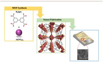
Scheme 1 Schematic representation of the optimized solvothermal preparation approach of the NOTT-300 (Al) MOF and its thin film fabrication on the interdigitated electrodes (IDEs).
