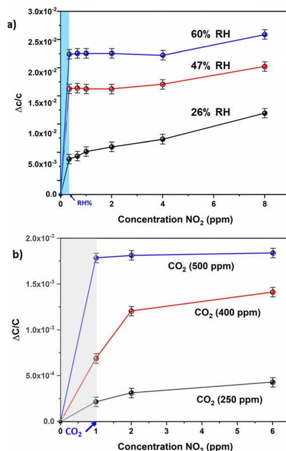
Fig. 5 Effects of various exposure conditions: (a) variable relative humidity ranging from 26 to 60% RH and (b) variable CO<sub>2</sub> concentrations ranging from 250 to 500 ppm on the performance of the Al-NOTT-300 sensor.
