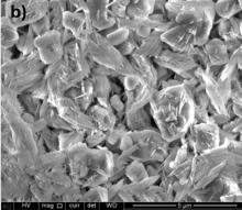
Fig. 1 (a) Calculated X-ray diffraction (XRD) patterns of the NOTT-300 (Al) MOF (black) and thin film deposited on the IDE substrate (red) and (b) top view SEM image of the thin film.
