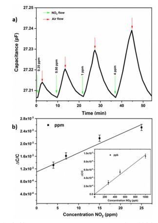
Fig. 2 (a) Dynamic response-recovery curve of the NOTT-300 (Al) MOF sensor to different concentrations of NO2. (b) The detection of NO2 in different concentration ranges: 250 ppb-4 ppm and (inset) 250-1000 ppb linear response for the corresponding range.
