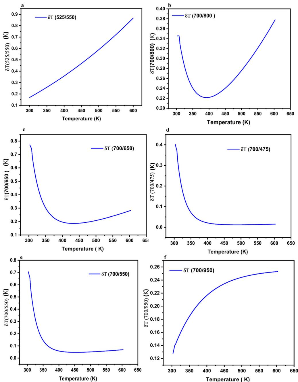
Fig. 14 Temperature uncertainty of BGVO: $\text{Er}^{3+}/\text{Tm}^{3+}/\text{Yb}^{3+}$ : (a)  $\delta T$  (525/550) nm, (b)  $\delta T$  (700/800) nm, (c)  $\delta T$  (700/475) nm, (d)  $\delta T$  (700/650), (e)  $\delta T$  (700/550) nm, and (f)  $\delta T$  (700/950) under 975 nm excitation.
