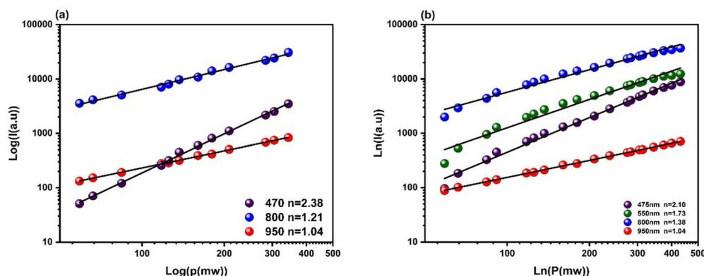
Fig. 5 Dependence of the intensity with the pump power at 975 nm of (a) BGVO:Tm<sup>3+</sup>/Yb<sup>3+</sup> and (b) BGVO:Er<sup>3+</sup>/Tm<sup>3+</sup>/Yb<sup>3+</sup>.
