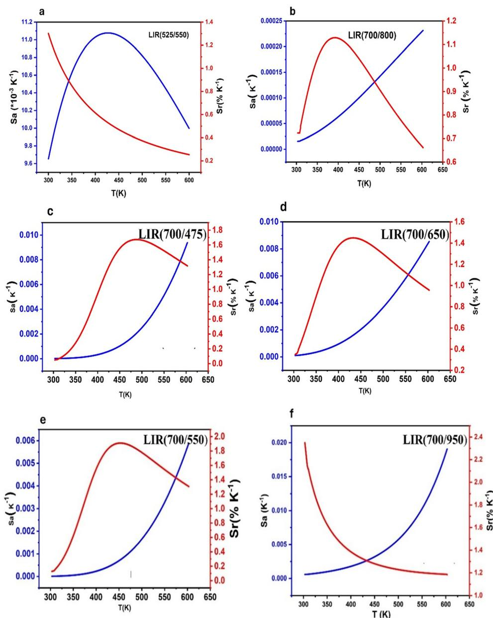
Fig. 13 The calculated  $S_a$  and  $S_r$  values based on  $\text{Er}^{3+}/\text{Tm}^{3+}/\text{Yb}^{3+}$ : (a) 700/800 nm, (b) 700/650, (c) 700/475, (d) 700/550 nm, (e) 525/550 nm and (f) 700/950 nm as a function of temperature.
