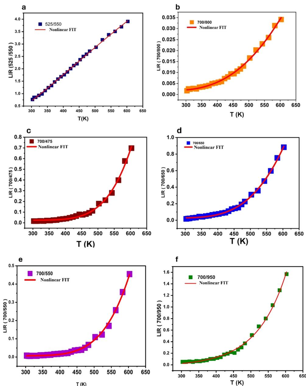
Fig. 12 LIR variations of  $\text{Er}^{3+}/\text{Tm}^{3+}/\text{Yb}^{3+}$ ; (a) 525/550 nm, (b) 700/800 nm, (c) 700/475 nm, (d) 700/650 nm, (e) 700/550 nm and (f) 700/950 nm as a function of temperature.
