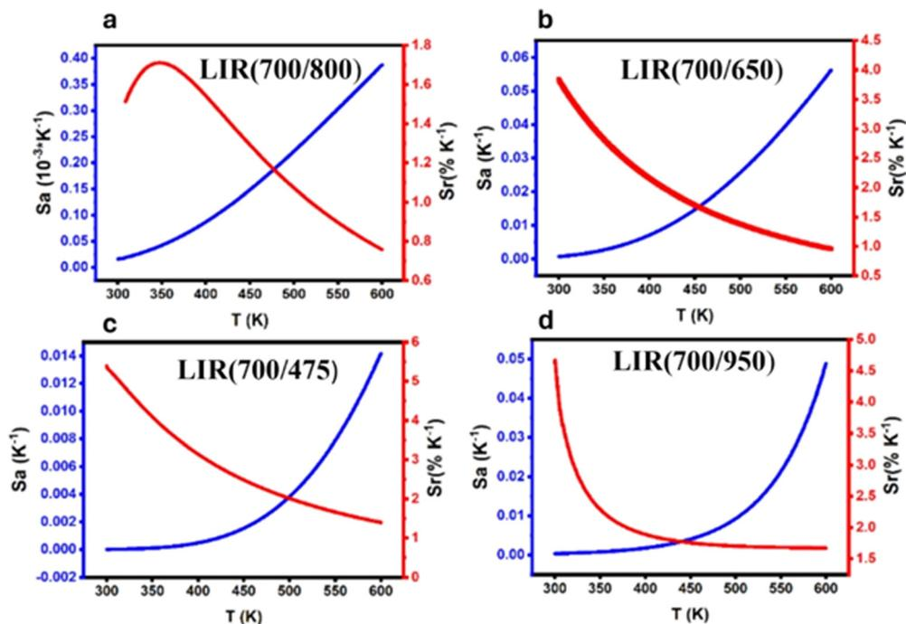
Fig. 9 The calculated  $S_a$  and  $S_r$  values based on  $\text{Tm}^{3+}/\text{Yb}^{3+}$  (a) LIR 700/800 nm, (b) LIR 700/650 nm, (c) LIR 700/475 nm and (d) LIR 700/950 nm as a function of temperature.
