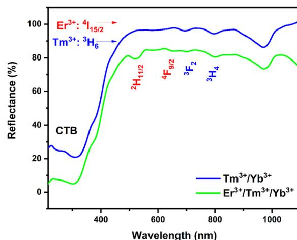
Fig. 3 The reflectance spectra of BGVO doped Tm<sup>3+</sup>, Er<sup>3+</sup>, Yb<sup>3+</sup>.
