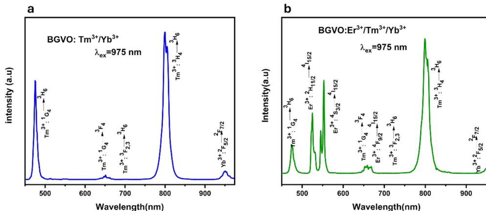
Fig. 4 Up-conversion emission spectra (a) of the BGVO:Tm<sup>3+</sup>/Yb<sup>3+</sup> and (b) of the BGVO:Er<sup>3+</sup>/Tm<sup>3+</sup>/Yb<sup>3+</sup> upon 975 nm excitation.
