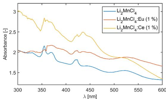
Fig. 3 Absorption spectra of the  $\text{Li}_2\text{MnCl}_4$  samples.
