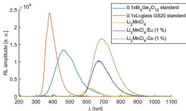
Fig. 11 RL spectra of all three Li<sub>2</sub>MnCl<sub>4</sub> samples together with BGO and glass neutron scintillator GS20 reference samples. The amplitude of BGO and GS20 spectra was divided by 10 for better comparison.
