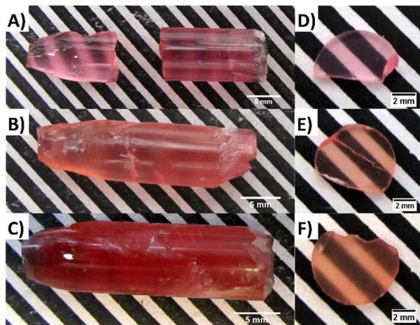
Fig. 1 Photos of as the grown crystals of (A–C) and samples prepared for optical characterization (D–F) of undoped  $\text{Li}_2\text{MnCl}_4$  (A) and (D),  $\text{Li}_2\text{MnCl}_4:\text{Eu}^{2+}$  (B) and (E), and  $\text{Li}_2\text{MnCl}_4:\text{Ce}^{3+}$  (C) and (F) respectively.
