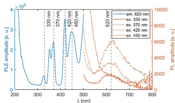
Fig. 6 PLE and PL spectra of the undoped  $\text{Li}_2\text{MnCl}_4$  sample. The excitation and emission wavelengths are indicated by dashed lines. The high intensity at around 200 and 500 nm is due to overcorrection and light scattering respectively.
