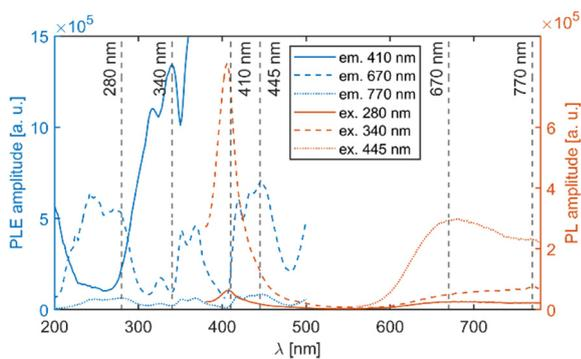
Fig. 7 PLE and PL spectra of the Li<sub>2</sub>MnCl<sub>4</sub>:Eu<sup>2+</sup> (1%) sample. The excitation and emission wavelengths are indicated by dashed lines. The high intensity at around 200 nm is due to overcorrection.
