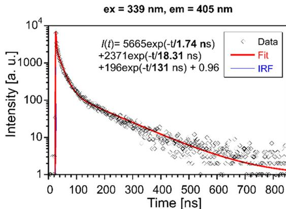
Fig. 9 PL decay curve of  $\text{Li}_2\text{MnCl}_4:\text{Eu}$  ( $\lambda_{\text{ex}} = 339 \text{ nm}$ ,  $\lambda_{\text{em}} = 405 \text{ nm}$ ). Red solid line is convolution of function  $I(t)$  and instrumental response function IRF.
