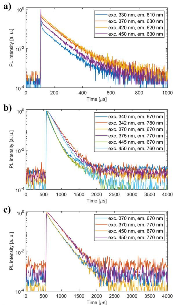
Fig. 10 PL decay curves of (a) undoped  $\text{Li}_2\text{MnCl}_4$  (b)  $\text{Li}_2\text{MnCl}_4:\text{Eu}^{2+}$  and (c)  $\text{Li}_2\text{MnCl}_4:\text{Ce}^{3+}$ . Excitation and emission wavelengths are noted in the legend.
