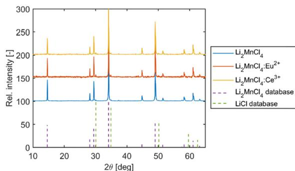
Fig. 2 X-ray powder diffraction of samples prepared from all three  $\text{Li}_2\text{MnCl}_4$  crystals. The database records for  $\text{Li}_2\text{MnCl}_4$  (ICSD PDF no. 01-070-0935) and  $\text{LiCl}$  (ICSD PDF no. 00-004-0664) are shown in dashed lines.
