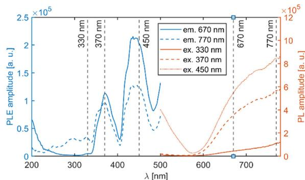
Fig. 8 PLE and PL spectra of the Li<sub>2</sub>MnCl<sub>4</sub>:Ce<sup>3+</sup> (1%) sample. The excitation and emission wavelengths are indicated by dashed lines. The high intensity at around 200 and 500 nm is due to overcorrection and light scattering respectively.
