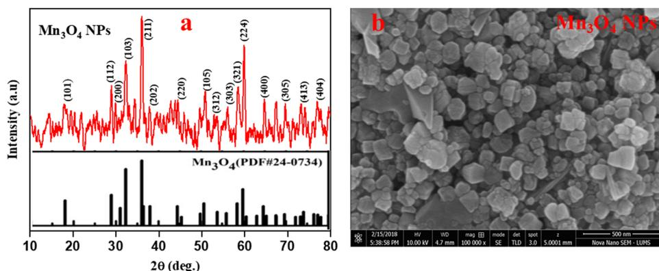
Fig. 1 (a) XRD spectra, and (b) SEM micrograph of the as-prepared Mn<sub>3</sub>O<sub>4</sub> NPs.
