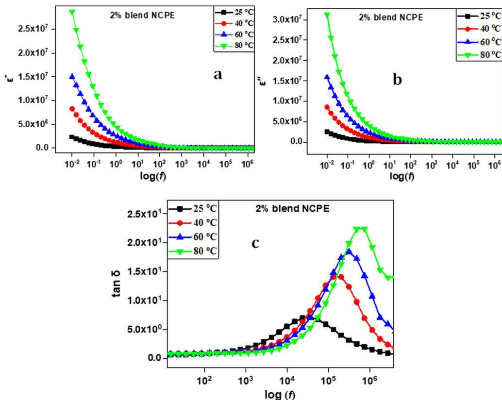
Fig. 11 Dielectric data for the 2% blend NCPE representing frequency dependent (a) dielectric constant, (b) dielectric loss and (c) loss tangent at various temperatures.
