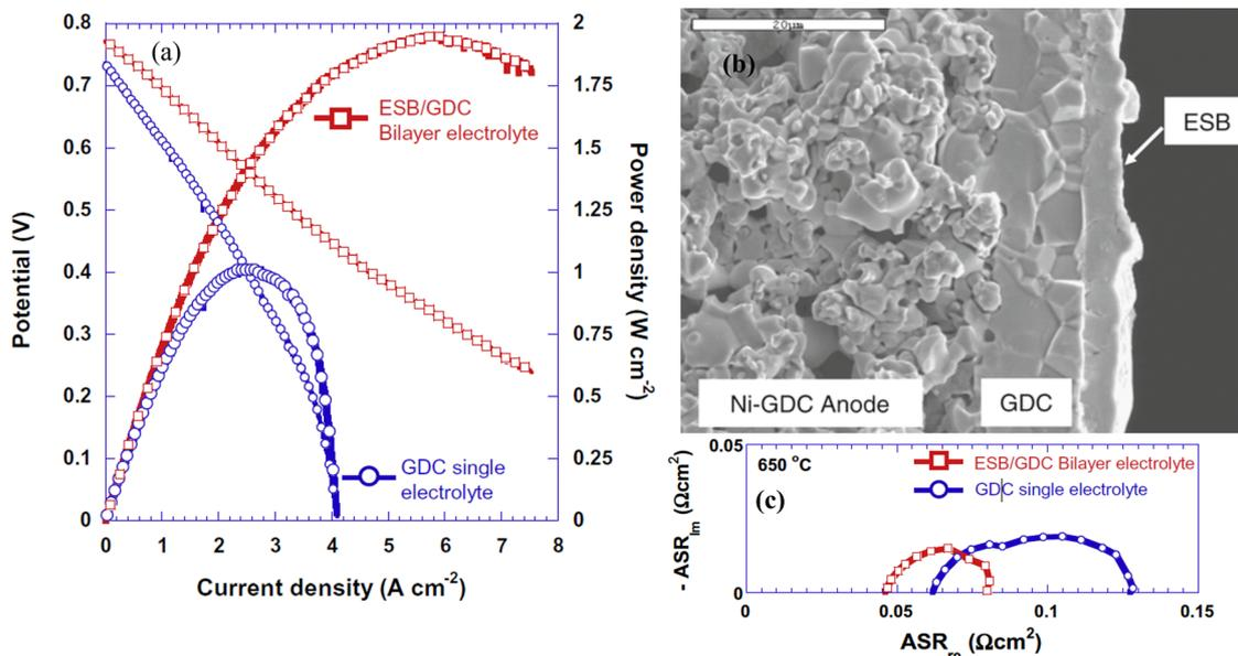
Fig. 19  $I$ - $V$  characteristics of fuel cell samples with single layer GDC and bilayer ESB/GDC electrolyte at 650 °C using 90 sccm of air and wet hydrogen. (b) SEM micrograph of the cross-section of ESB/GDC bilayer electrolyte with anode support. (c) Impedance spectra of the GDC and ESB/GDC electrolyte.<sup>349</sup> Reproduced from ref. 349 with permission from [Elsevier], copyright [2009].
