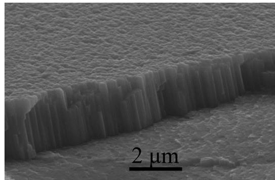
Fig. 14 PVD ceramic layer.<sup>306</sup> Reproduced from ref. 306 with permission from [Springer], copyright [2014].
