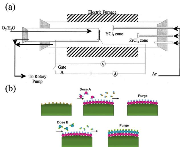
Fig. 16 The illustration of (a) the CVD reactor and (b) the ALD process.<sup>237,268</sup> Reproduced from ref. 237 with permission from [Springer], copyright [2020].
