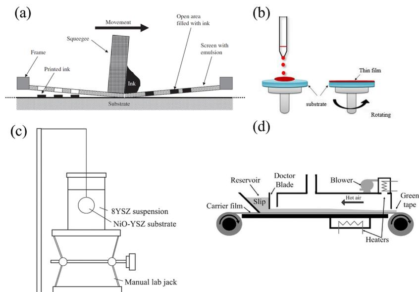
**Fig. 13** Illustration of (a) the screen-printing process; (b) the spin-coating process; (c) the dip-coating process; and (d) the tape-casting process.<sup>272–275</sup> Reproduced from ref. 272 with permission from [Elsevier], copyright [2017]. Reproduced from ref. 273 with permission from [Elsevier], copyright [2009]. Reproduced from ref. 274 with permission from [Elsevier], copyright [2011]. Reproduced from ref. 275 with permission from [Elsevier], copyright [2017].
