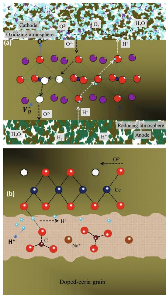
Fig. 11 (a) Schematic model of mixed conduction for single perovskite-based electrolyte. (b) Schematic model of SDC/Na<sub>2</sub>CO<sub>3</sub> nanocomposite.<sup>213,216</sup> Reproduced from ref. 213 with permission from [Elsevier], copyright [2021].
