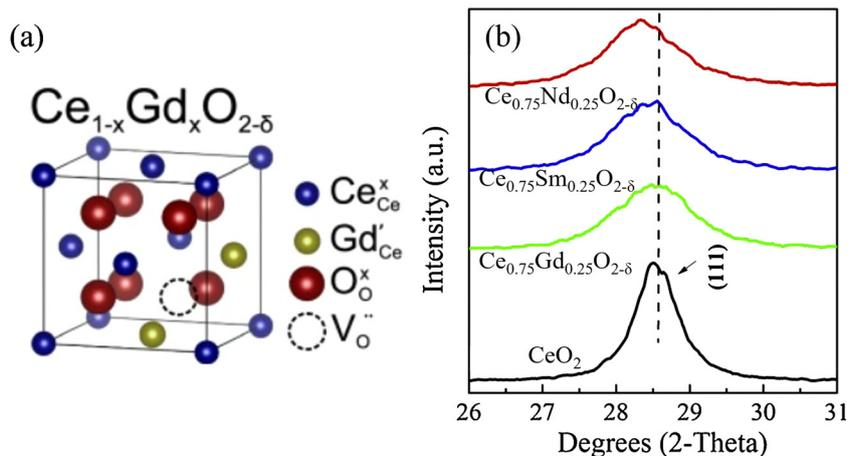
Fig. 7 (a) Crystal structure of  $\text{Ce}_{1-x}\text{Gd}_x\text{O}_{2-\delta}$ .<sup>140</sup> (b) XRD patterns of  $\text{Ce}_{0.8}\text{Sm}_{0.2}\text{O}_{2-\delta}$ ,  $\text{Ce}_{0.8}\text{Gd}_{0.2}\text{O}_{2-\delta}$  and  $\text{Ce}_{0.8}\text{Nd}_{0.2}\text{O}_{2-\delta}$ . Reproduced from ref. 140 with permission from [Elsevier], copyright [2017]. Reproduced from ref. 141 with permission from [Elsevier], copyright [2017].
