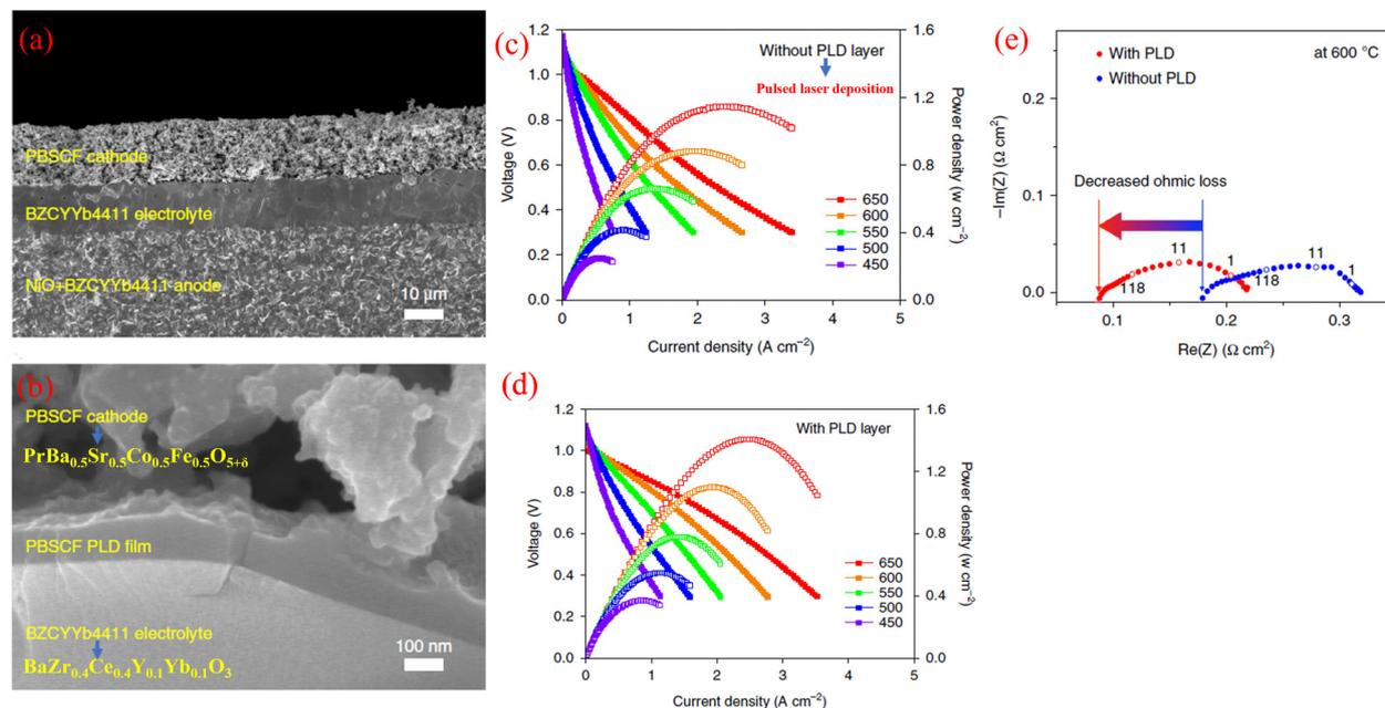
**Fig. 18** Scanning electron microscope images of a cross-section of (a) PBSCF/BZCYYb/BZCYYb + NiO cermet anode fuel cell without PLD layer and (b) with PLD layer. The polarization and power density of cermet anode fuel cell (c) without PLD layer and (d) with PLD layer using humidified  $H_2$  as fuel and dry air as oxidant. (e) Impedance spectra at 600 °C with and without PLD layer.<sup>346</sup> Reproduced from ref. 346 with permission from [Springer Nature], copyright [2018].
