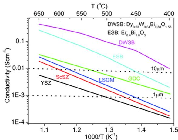
Fig. 6 Conductivities of electrolyte materials at different operating temperatures. The horizontal dashed line indicated the conductivity requirement to achieve ASR < 0.1 Ω cm<sup>-1</sup> at the thickness of 1 μm and 10 μm.<sup>118</sup> Reproduced from ref. 118 with permission from [Royal Society of Chemistry], copyright [2016].
