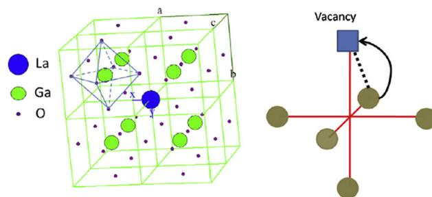
Fig. 9 The cubic ABO<sub>3</sub> perovskite structure, and the path of oxygen ions migration along BO<sub>6</sub> octahedron edge.<sup>184</sup> Reproduced from ref. 184 with permission from [Elsevier], copyright [1995].
