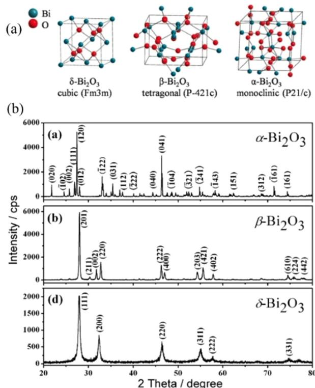
Fig. 8 (a) The crystal structure<sup>170</sup> and XRD pattern<sup>7</sup> of α-Bi<sub>2</sub>O<sub>3</sub>, β-Bi<sub>2</sub>O<sub>3</sub> and γ-Bi<sub>2</sub>O<sub>3</sub>. Reproduced from ref. 170 with permission from [Elsevier], copyright [2023]. Reproduced from ref. 7 with permission from [Royal Society of Chemistry], copyright [2010].
