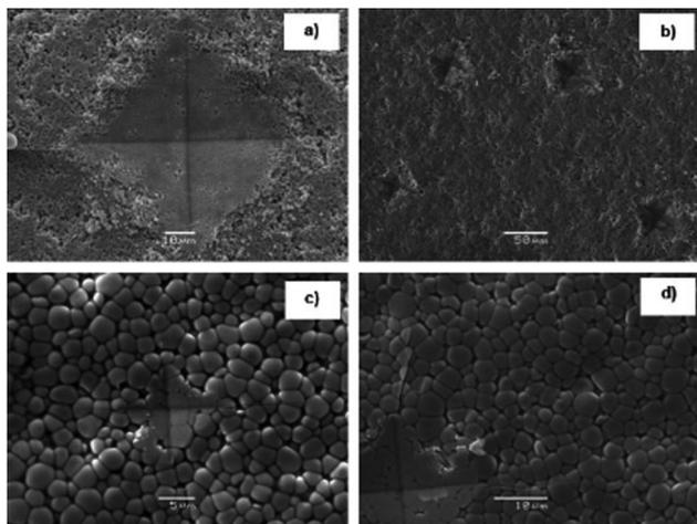
**Fig. 21** The sample of  $\text{Ce}_{0.9}\text{Gd}_{0.1}\text{O}_{1.95}$  of Pyramid-shaped Vickers indentation marks on tape sintered at (a) 1300, (b) 1400 °C/2 h, (c) and (d) indentation imprint and emanated crack on the tapes sintered at 1500 °C 2 h<sup>-1</sup>.<sup>358</sup> Reproduced from ref. 358 with permission from [Wiley], copyright [2013].
