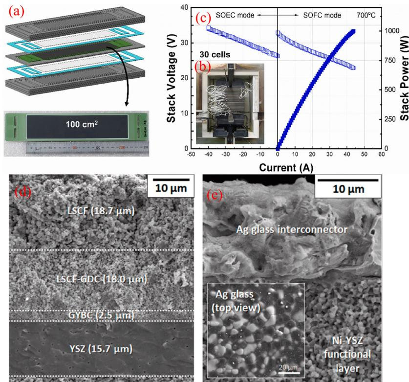
**Fig. 23** (a) Schematic diagram of reversible SOC with repeating cell units; (b) photograph of 1 kW class stack; (c)  $I$ - $V$  curves of both SOEC and SOFC mode for 30-cell stack at 700 °C; (d) and (e) cross-section SEM image of the cell area and Ag glass interconnector.<sup>369</sup> Reproduced from ref. 369 with permission from [Elsevier], copyright [2022].
