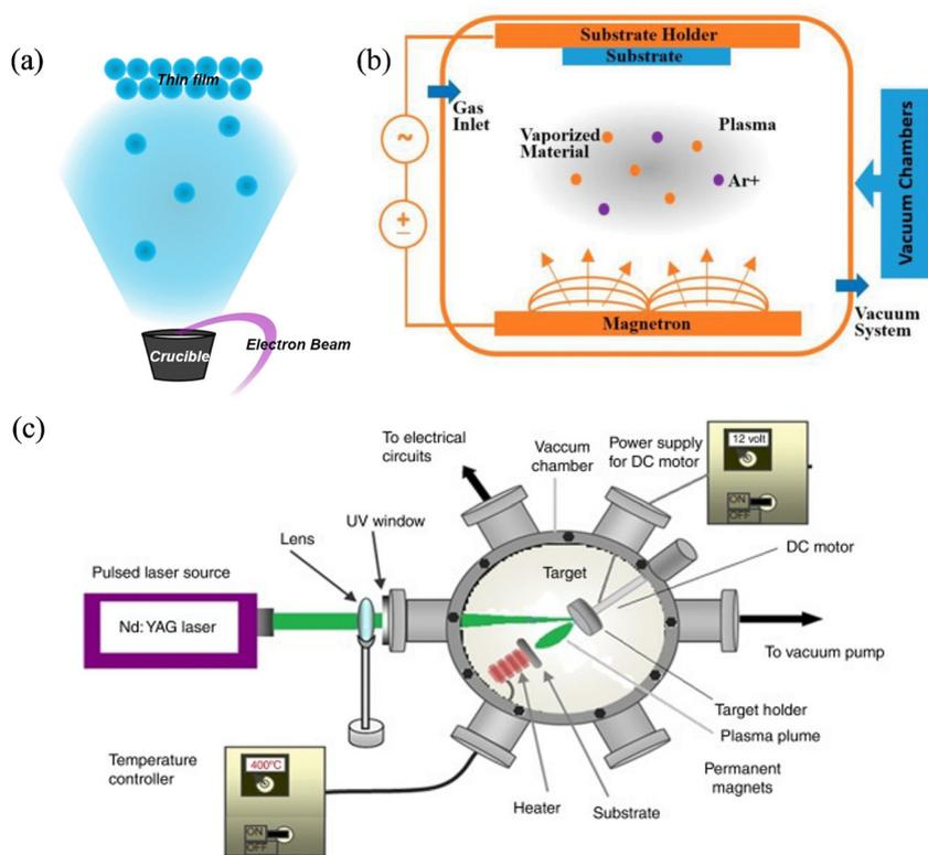
Fig. 15 Schematic illustration of the (a) EB-PVD, (b) sputtering, (c) PLD.<sup>244,268,309</sup> Reproduced from ref. 244 with permission from [Springer], copyright [2020]. Reproduced from ref. 309 with permission from [MDPI], copyright [2023].
