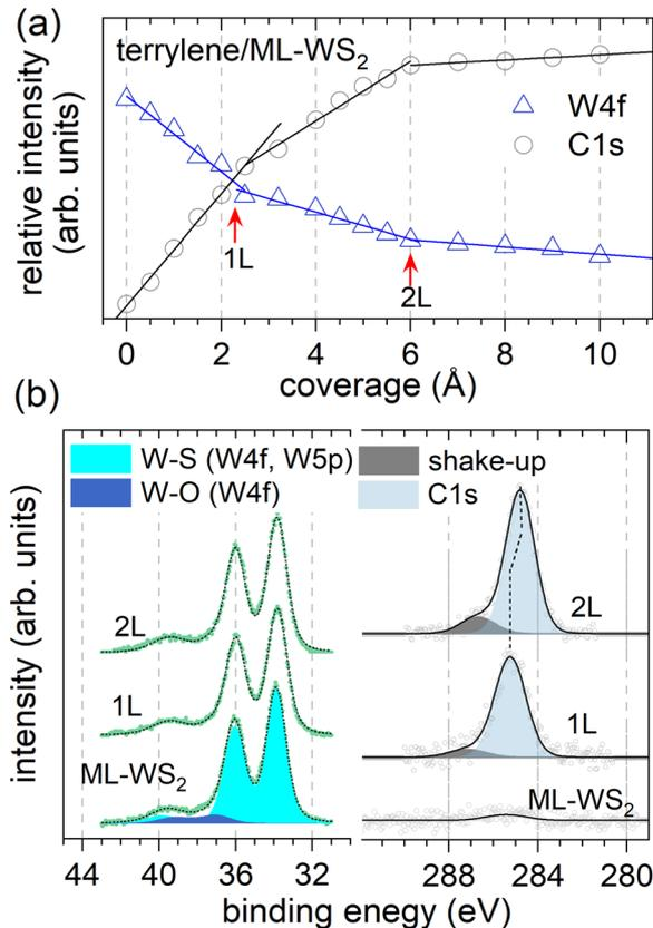
Fig. 3 (a) Variation of the relative XPS intensities of W 4f and C 1s of terrylene/ML-WS<sub>2</sub> as a function of coverage based on XPS data (Fig. S4, ESI†). For W 4f (C 1s), three linear decreasing (increasing) intensity regions could be fitted, with corresponding slope changes (red arrows). (b) W 4f and C 1s XPS spectra (Shirley background subtracted) of bare ML-WS<sub>2</sub> and 1L and 2L of terrylene/ML-WS<sub>2</sub>.
