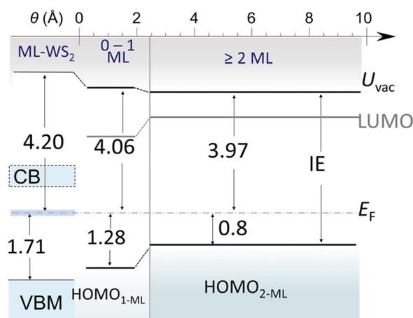
Fig. 7 Schematic energy level alignment in terrylene/ML-WS<sub>2</sub> heterostructures. The energy difference between energy levels and  $E_F$  is shown by arrows and numbers (unit, eV). The partially filled CB in ML-WS<sub>2</sub> is indicated by blue shading. Note that the "0-1 ML" region was no longer present as soon as the 2 ML coverage region has formed because the 1L flat-lying wetting layer of terrylene was consumed to form the 2L inclined layer (see Fig. 5 and associated text).
