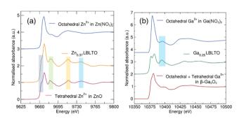
Fig. 4 (a) XANES region of the XAS data measured on the Zn K-edge for  $\text{Li}_{5.25}\text{Zn}_{0.37}\text{BaLa}_2\text{Ta}_2\text{O}_{12}$ , and  $\text{Zn}(\text{NO}_3)_2\cdot 6\text{H}_2\text{O}$  and ZnO standards. (b) XANES region of the XAS data measured on the Ga K-edge for Li<sub>5.25</sub>Ga<sub>0.25</sub>BaLa<sub>2</sub>- $Ta_2O_{12}$  and,  $Ga(NO_3)_3 \cdot 9H_2O$  and  $Ga_2O_3$  standards. Coloured boxes indicate common features in the XANES profiles between the different
