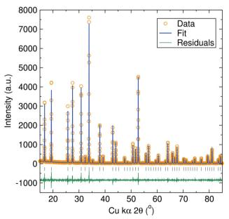
Fig. 2 Rietveld refinements of PXRD data for the Li<sub>6</sub>BaLa<sub>2</sub>Ta<sub>2</sub>O<sub>12</sub> material. Bragg peak positions for the cubic Li<sub>6</sub>BaLa<sub>2</sub>Ta<sub>2</sub>O<sub>12</sub> garnet structure are indicated by vertical grey tick marks. Fit was in good agreement with the cubic space group  $Ia\bar{3}d$  with the following cell parameters: a=13.0018(1) Å and V=2197.89(3) Å $^3$ .  $R_{wp}=0.1381$ ,  $R_p=0.1002$ ,  $R_F2=0.0344$  and  $\gamma^2=2.055$ .
