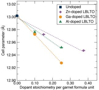
Fig. 3 Unit cell parameter evolution following Vegard's law for the cubic la3d garnet crystal structure with an increase in Al3+, Ga3+ and Zn2+ dopant concentrations.
