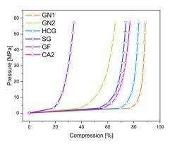
Fig. 11 Compression curves of different conductive additives and a carbon aerogel CA2
