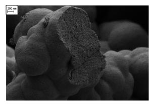
Fig. 1 Microstructure of a carbon aerogel with inter- and intraconnected particles
