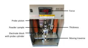
Fig. 3 Setup for measurements on powdered materials. 31
