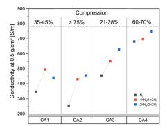
Fig. 6 Conductivities of CA1–CA4 aerogels at the bulk density  $\rho = 0.5$  g cm<sup>-3</sup> showing a linear increase of conductivity from non-activated to activated samples.
