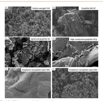
Fig. 12 SEM images of different additives.
