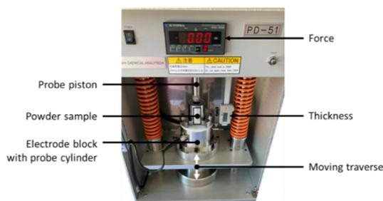
Fig. 3 Setup for measurements on powdered materials.<sup>31</sup>
