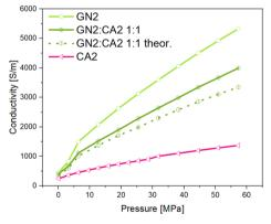
Fig. 17 Measured and theoretical conductivity curves of composites GN2:CA2 under pressure.
