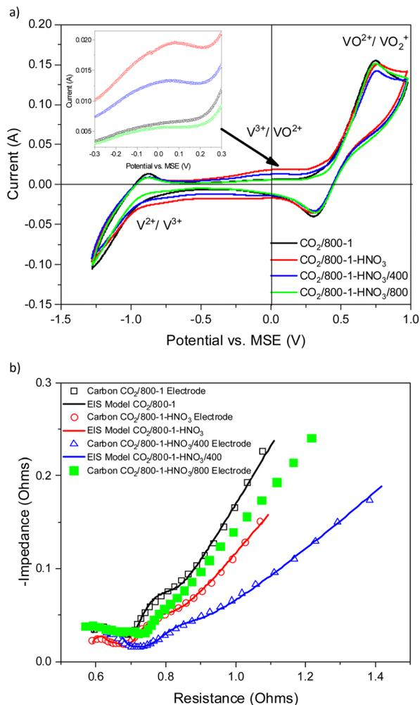
Fig. 9 Comparison of electrochemical results for electrodes prepared from carbons  $\text{CO}_2/800-1$ ,  $\text{CO}_2/800-1-\text{HNO}_3$ ,  $\text{CO}_2/800-1-\text{HNO}_3/400$ , and  $\text{CO}_2/800-1-\text{HNO}_3/800$  prepared by oxidation in nitric acid and heat treatment (a) cyclic voltammograms with inset figure for potential range  $-0.3$  to  $0.3$  V, and (b) Nyquist plots and corresponding models.
