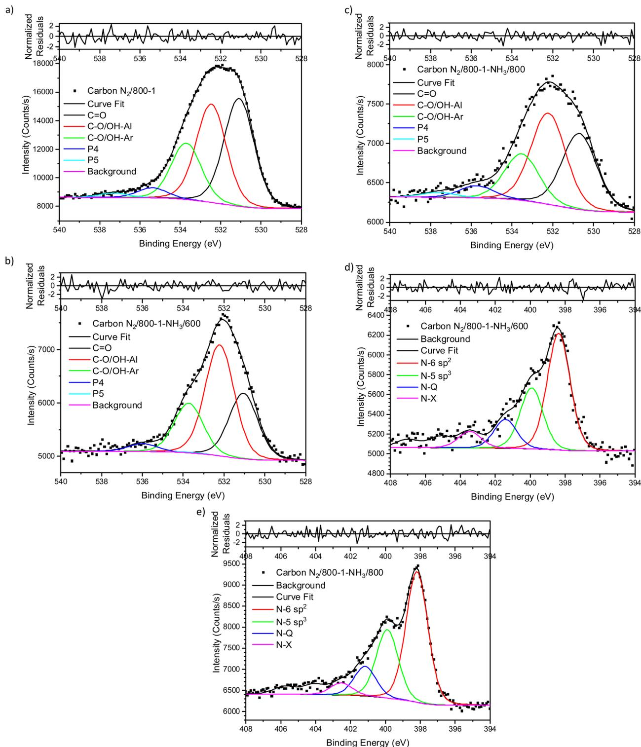
Fig. 3 Comparison of XPS spectra, curve fitting, and residuals of untreated carbon and  $\text{NH}_3$  treated carbons (a) O 1s, carbon  $\text{N}_2/800-1$ , (b) O 1s, carbon  $\text{N}_2/800-1-\text{NH}_3/600$  (c) O 1s, carbon  $\text{N}_2/800-1-\text{NH}_3/800$ , (d) N 1s, carbon  $\text{N}_2/800-1-\text{NH}_3/600$  and (e) N 1s, carbon  $\text{N}_2/800-1-\text{NH}_3/800$ .
