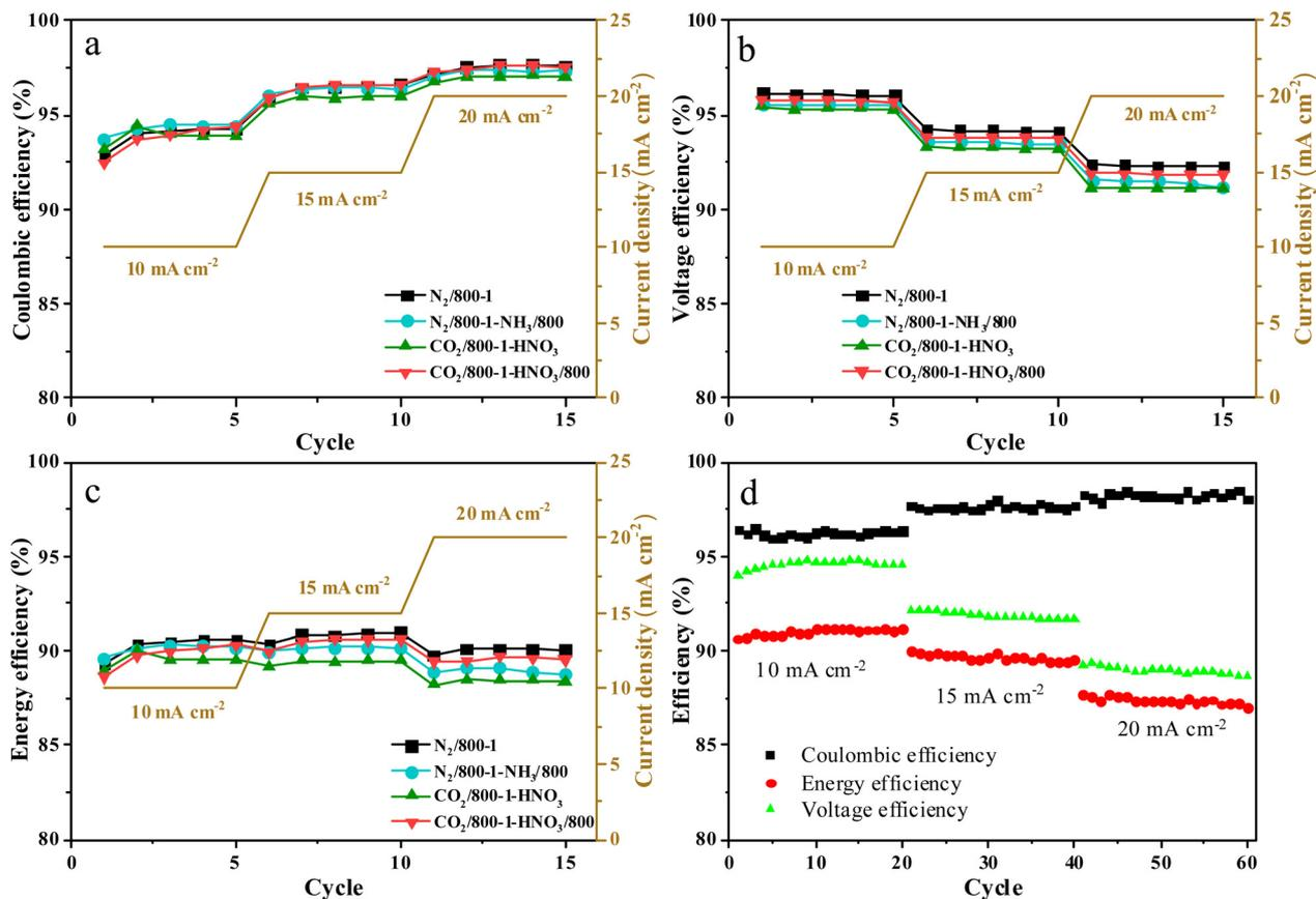
Fig. 12 Comparison of cell performance for carbons  $N_2/800-1$ ,  $N_2/800-1-NH_3/800$ ,  $CO_2/800-1-HNO_3$  and  $CO_2/800-1-HNO_3/800$ . (a) Coulombic, (b) voltage, (c) energy efficiency, and (d) stability test of  $N_2/800-1$  for 20 cycles at each current density of 10, 15, and 20  $mA\ cm^{-2}$ .
