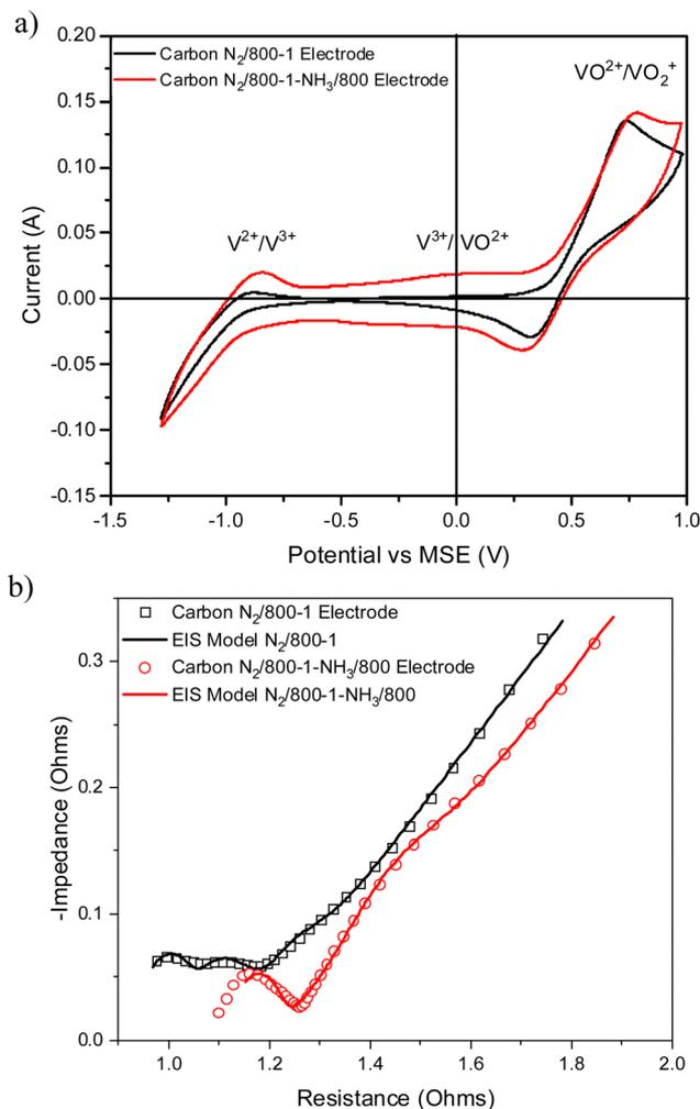
Fig. 11 Comparison of electrochemical results for electrodes prepared from carbons N<sub>2</sub>/800-1 and N<sub>2</sub>/800-1-NH<sub>3</sub>/800 (a) cyclic voltammograms and (b) Nyquist plots and corresponding models.
