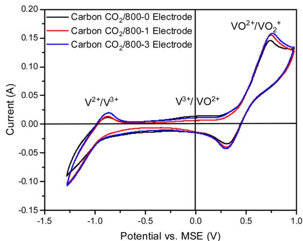
Fig. 7 Comparison of cyclic voltammograms of electrodes prepared from carbons with HTT 800 °C and various hold times (carbons CO<sub>2</sub>/800-0, CO<sub>2</sub>/800-1, and CO<sub>2</sub>/1000-3) for vanadium redox reactions, Sweep rate 20 mV s<sup>-1</sup>.
