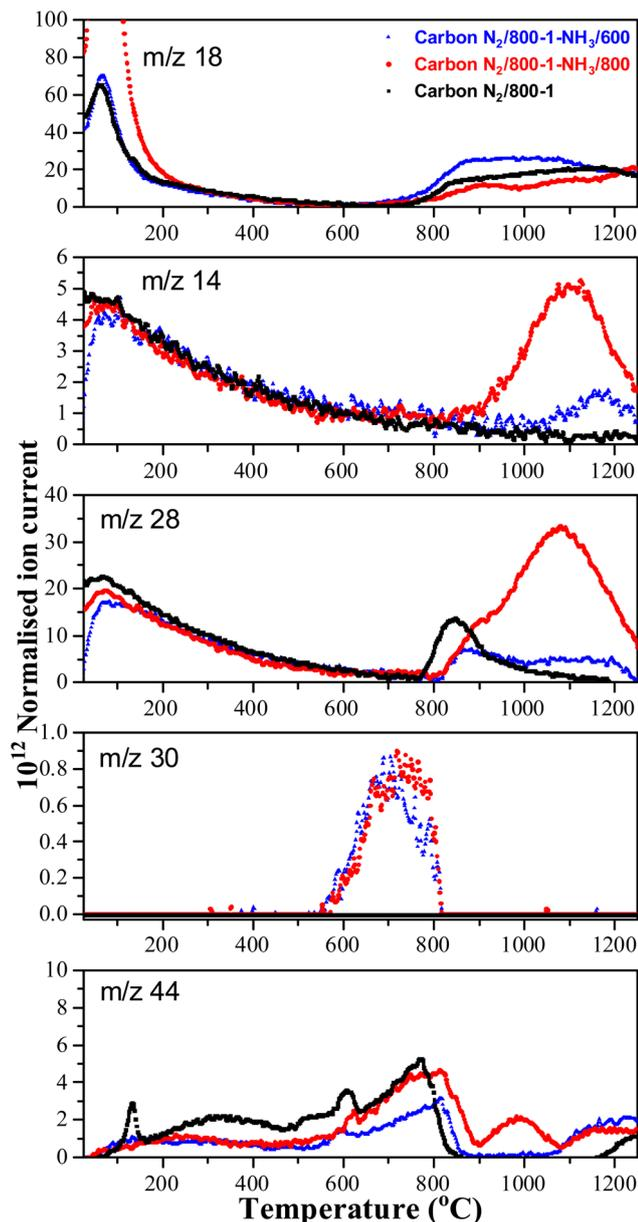
Fig. 6 Comparison TPD profiles of carbon N<sub>2</sub>/800-1 and NH<sub>3</sub> treated carbons N<sub>2</sub>/800-1-NH<sub>3</sub>/600 and N<sub>2</sub>/800-1-NH<sub>3</sub>/800 in He (35 mL min<sup>-1</sup>) at 10 °C min<sup>-1</sup>.
