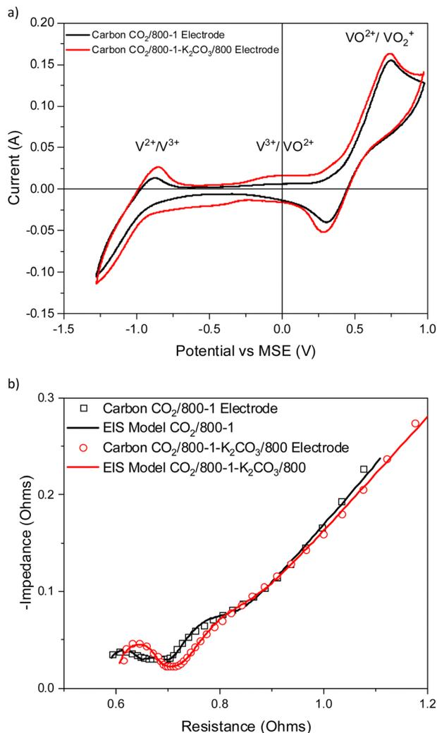
Fig. 10 Comparison of electrochemical results for electrodes prepared from carbons CO<sub>2</sub>/800-1 and CO<sub>2</sub>/800-1-K<sub>2</sub>CO<sub>3</sub>/800 (a) cyclic voltammograms and (b) Nyquist plots and corresponding models.
