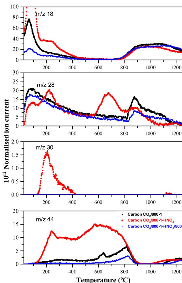
Fig. 4 Comparison of TPD profiles of carbon CO<sub>2</sub>/800-1 and HNO<sub>3</sub> oxidized and heat-treated carbons (CO<sub>2</sub>/800-1-HNO<sub>3</sub> and CO<sub>2</sub>/800-1-HNO<sub>3</sub>/800) in He (35 mL min<sup>-1</sup>) at 10 °C min<sup>-1</sup>.
