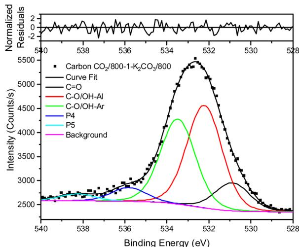
Fig. 2 XPS O 1s spectrum, curve fitting, and residuals of carbon CO<sub>2</sub>/800-1-K<sub>2</sub>CO<sub>3</sub>/800.
