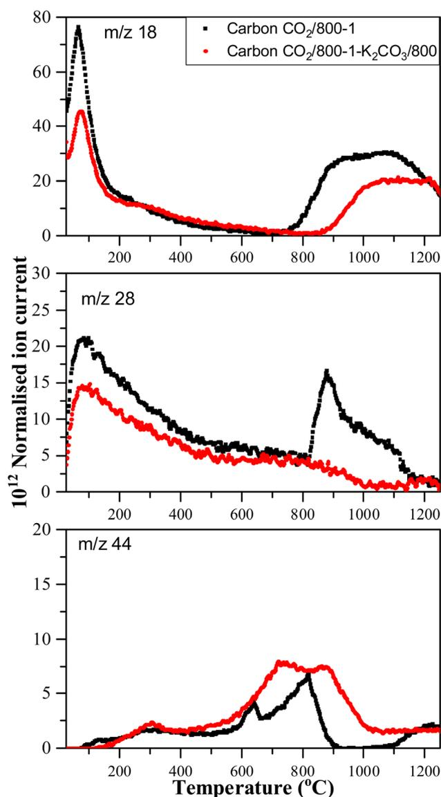
Fig. 5 Comparison of TPD profiles of carbons CO<sub>2</sub>/800-1 and CO<sub>2</sub>/800-1-K<sub>2</sub>CO<sub>3</sub>/800 in He (35 mL min<sup>-1</sup>) at 10 °C min<sup>-1</sup>.
