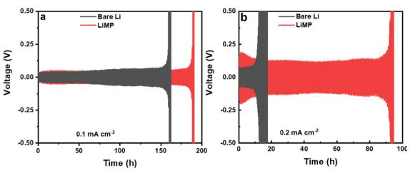
Fig. 7 Galvanostatic cycling results at current densities of (a) 0.1 mA cm<sup>-2</sup> and (b) 0.2 mA cm<sup>-2</sup> in the Li/CSE/Li cell configuration.
