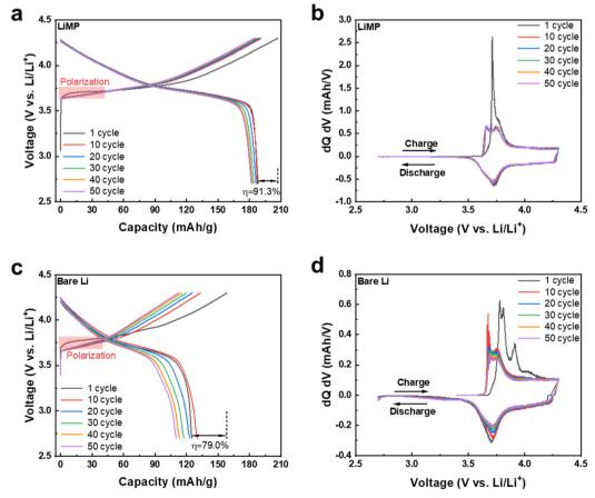
Fig. 9 (a) Charge-discharge profiles of LiMP||CSE||NCM622 with corresponding (b) dQ/dV results. (c) Charge-discharge profiles of bare Li||C-SE||NCM622 cells with the corresponding (d) dQ/dV results.
