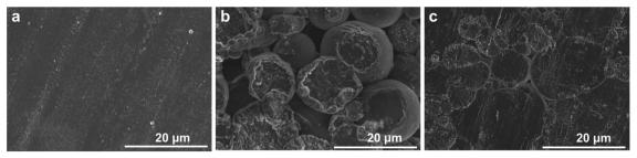
FE-SEM surface images of (a) bare Li foil, (b) 10% pressed LiMP electrode, and (c) 10% pressed LiMP electrode
