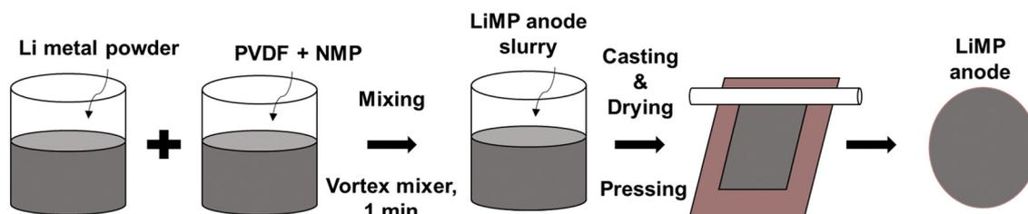
Fig. 1 Schematic diagram of LiMP electrode fabrication.
