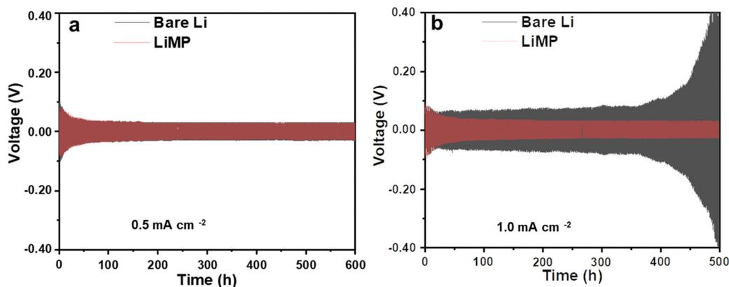
Fig. 3 Galvanostatic cycling results at current densities of (a)  $0.5 \text{ mA cm}^{-2}$  and (b)  $1 \text{ mA cm}^{-2}$  in the Li symmetric cell configuration using a liquid electrolyte.
