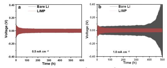
Fig. 3 Galvanostatic cycling results at current densities of (a) 0.5 mA cm<sup>-2</sup> and (b) 1 mA cm<sup>-2</sup> in the Li symmetric cell configuration using a liquid electrolyte.
