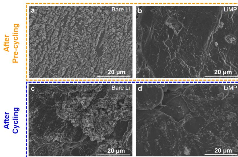
**Fig. 6** Surface FE-SEM images of (a) bare Li foil and (b) LiMP electrode after pre-cycling, and (c) bare Li foil and (d) LiMP electrode after cycling.
