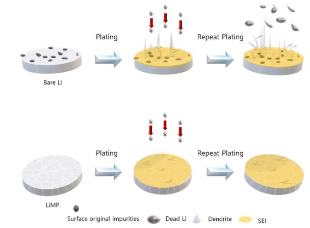
Fig. 10 The schematic of Li dendrite formation in the bare Li foil and LiMP electrode
