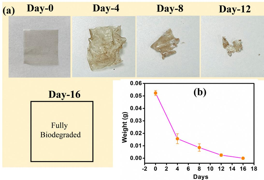
Fig. 8 (a) Photographs of 0.25CNF-4WME-SA film during biodegradable test. (b) Changes of weight during biodegradation 0.25CNF-4WME-SA film.
