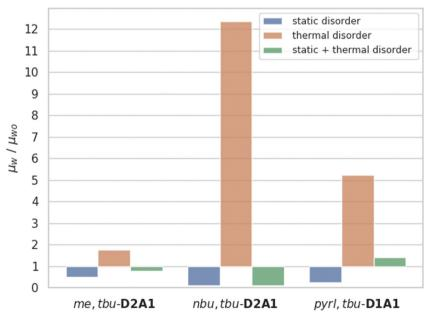
Fig. 5 Ratio of the computed hole mobilities  $(\mu_w/\mu_{wo})$  with the static (blue), thermal (red) and both static and thermal disorder effects (green) to the Brownian charge mobility without disorder effects for me,tbu-, nbu,tbu-D2A1 and pyrl,tbu-D1A1.
