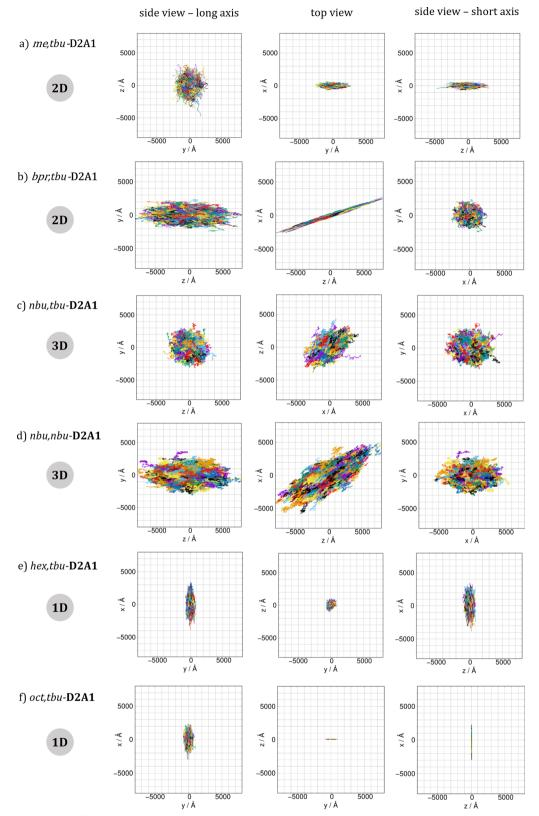
Fig. 3 kMC trajectories (1000, 10<sup>5</sup> steps each) for each crystal of **D2A1** ((a) me,tbu-, (b) bpr,tbu-, (c) nbu,tbu-, (d) nbu,nbu-, and (e) hex,tbu-, (f) oct,tbu-D2A1) in the absence of disorder. kMC trajectories are reported for the three Cartesian planes xy, xz and yz. The planes were ordered as: the side view (first column) onto the long molecular axis, the top (second column) and the side view (third column) onto the short molecular axis.
