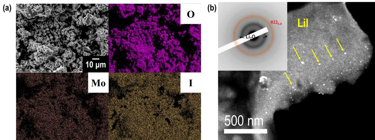
Fig. 2 (a) SEM-EDS images and (b) HCDF image and ED pattern of  $63\text{Li}_2\text{O}\cdot 32\text{LiI}\cdot 5\text{MoO}_3$ . In (b), bright-contrast regions indicated by arrows in yellow correspond to the LiI nanocrystals.
