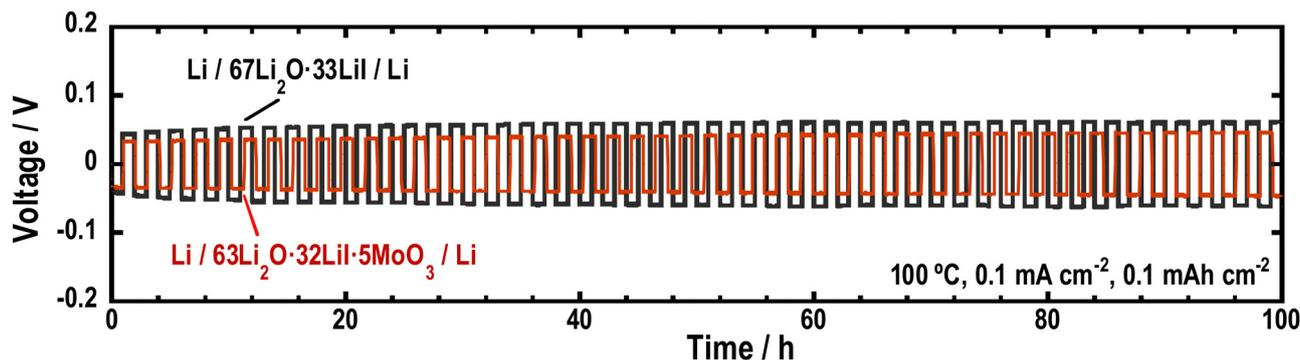
**Fig. 8** Galvanostatic cycling tests of the symmetric cells (Li/67Li<sub>2</sub>O·33LiI/Li) and (Li/63Li<sub>2</sub>O·32LiI·5MoO<sub>3</sub>/Li).
