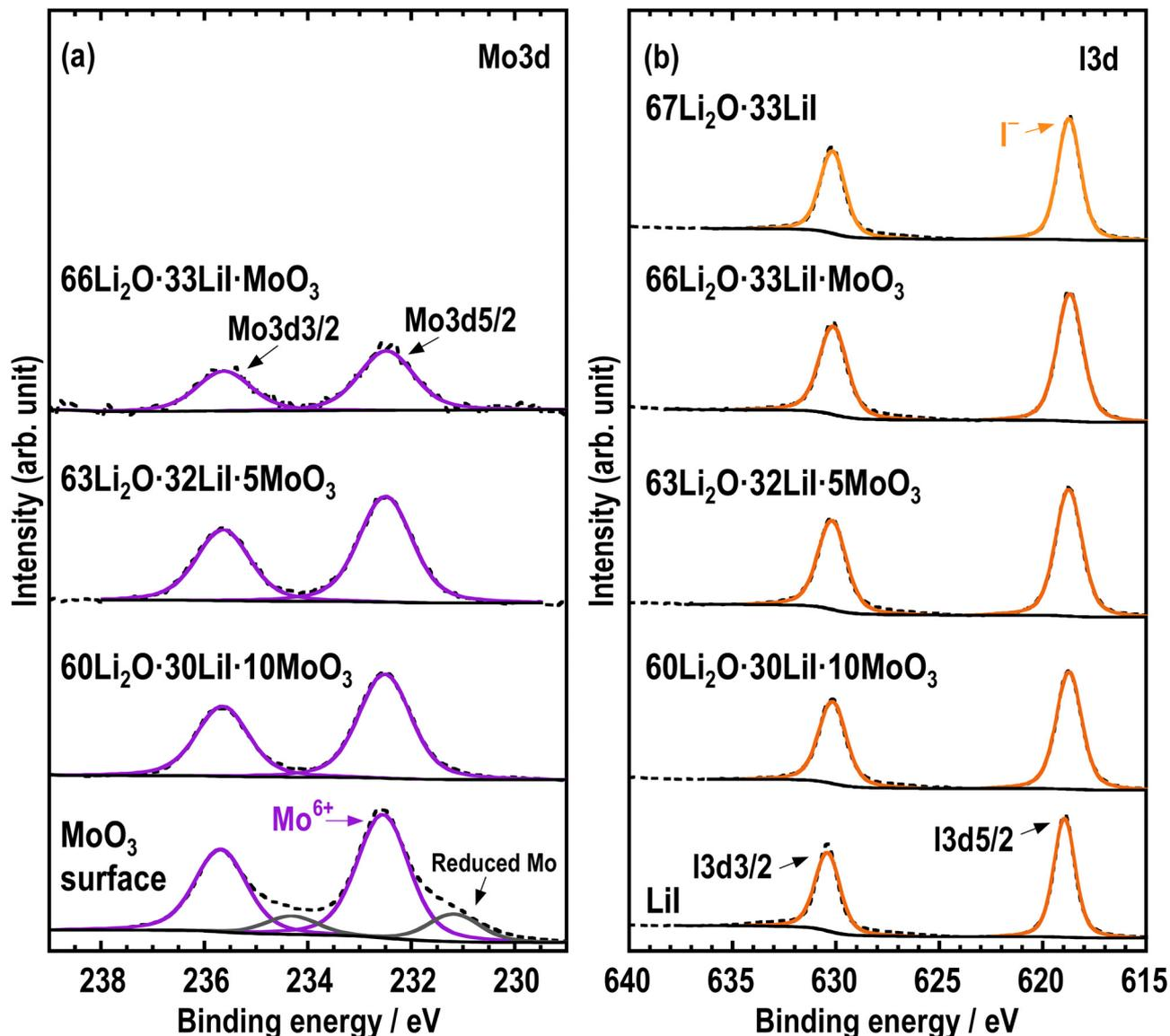
Fig. 5 (a) Mo 3d and (b) I 3d XPS spectra of  $67\text{Li}_2\text{O}\cdot 33\text{LiI}$ ,  $66\text{Li}_2\text{O}\cdot 33\text{LiI}\cdot \text{MoO}_3$ ,  $63\text{Li}_2\text{O}\cdot 32\text{LiI}\cdot 5\text{MoO}_3$ ,  $60\text{Li}_2\text{O}\cdot 30\text{LiI}\cdot 10\text{MoO}_3$ ,  $\text{MoO}_3$ , and LiI.
