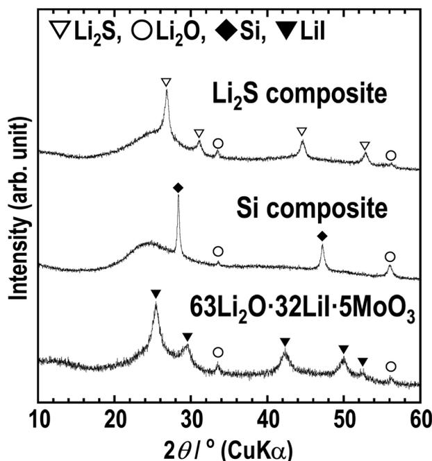
**Fig. 9** XRD patterns of the Li<sub>2</sub>S-VGCF–63Li<sub>2</sub>O·32LiI·5MoO<sub>3</sub> composite (Li<sub>2</sub>S composite), Si-VGCF–63Li<sub>2</sub>O·32LiI·5MoO<sub>3</sub> composite (Si composite), and 63Li<sub>2</sub>O·32LiI·5MoO<sub>3</sub>.
