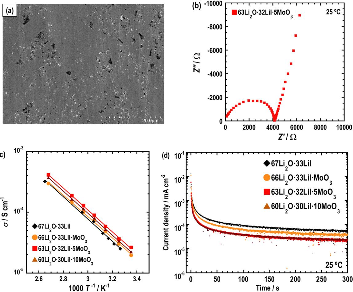
Fig. 7 (a) Cross-sectional SEM image of pellets of  $63\text{Li}_2\text{O}\cdot 32\text{LiI}\cdot 5\text{MoO}_3$ . (b) Nyquist plots, (c) temperature dependence and (d)  $I$ - $V$  curves of  $67\text{Li}_2\text{O}\cdot 33\text{LiI}$ ,  $66\text{Li}_2\text{O}\cdot 33\text{LiI}\cdot \text{MoO}_3$ ,  $63\text{Li}_2\text{O}\cdot 32\text{LiI}\cdot 5\text{MoO}_3$ , and  $60\text{Li}_2\text{O}\cdot 30\text{LiI}\cdot 10\text{MoO}_3$ .
