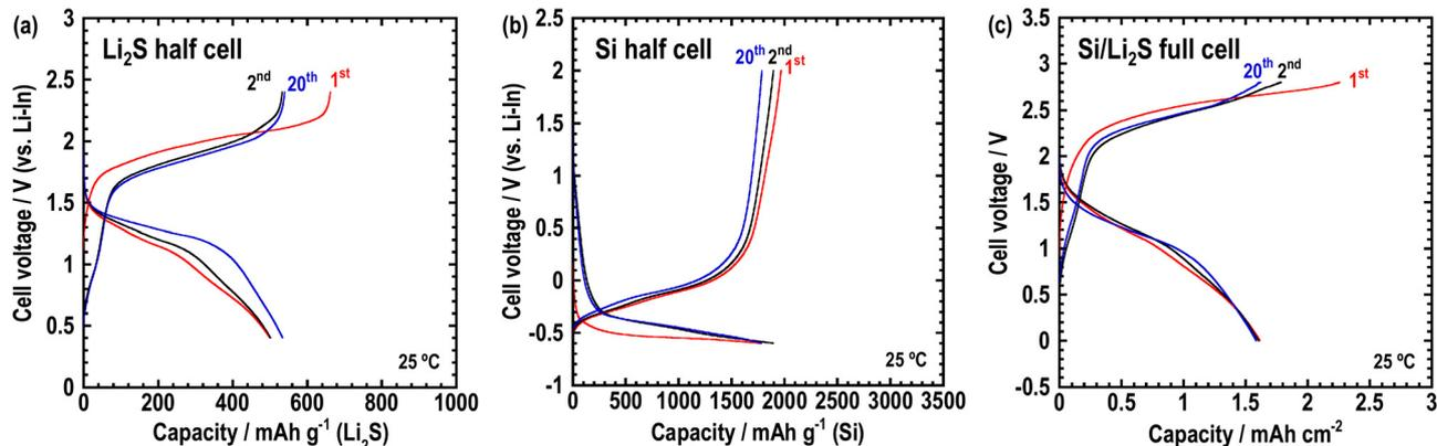
Fig. 10 Charge-discharge curves of the cell at 25 °C (a) (Li-In/Li<sub>3</sub>PS<sub>4</sub>/Li<sub>2</sub>S-VGCF-63Li<sub>2</sub>O-32LiI-5MoO<sub>3</sub>), (b) (Li-In/Li<sub>3</sub>PS<sub>4</sub>/Si-VGCF-63Li<sub>2</sub>O-32LiI-5MoO<sub>3</sub>), and (c) (Si-VGCF-63Li<sub>2</sub>O-32LiI-5MoO<sub>3</sub>/63Li<sub>2</sub>O-32LiI-5MoO<sub>3</sub>/Li<sub>2</sub>S-VGCF-63Li<sub>2</sub>O-32LiI-5MoO<sub>3</sub>).
