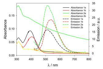
Fig. 6 Absorbance (solid lines) and emission spectra (dashed lines,  $\lambda_{\rm exc}$  = 400 nm and cut-off filter at 435 nm) of NPs embedding compounds **1a**, **1b**, **2a**, and **2b**.
