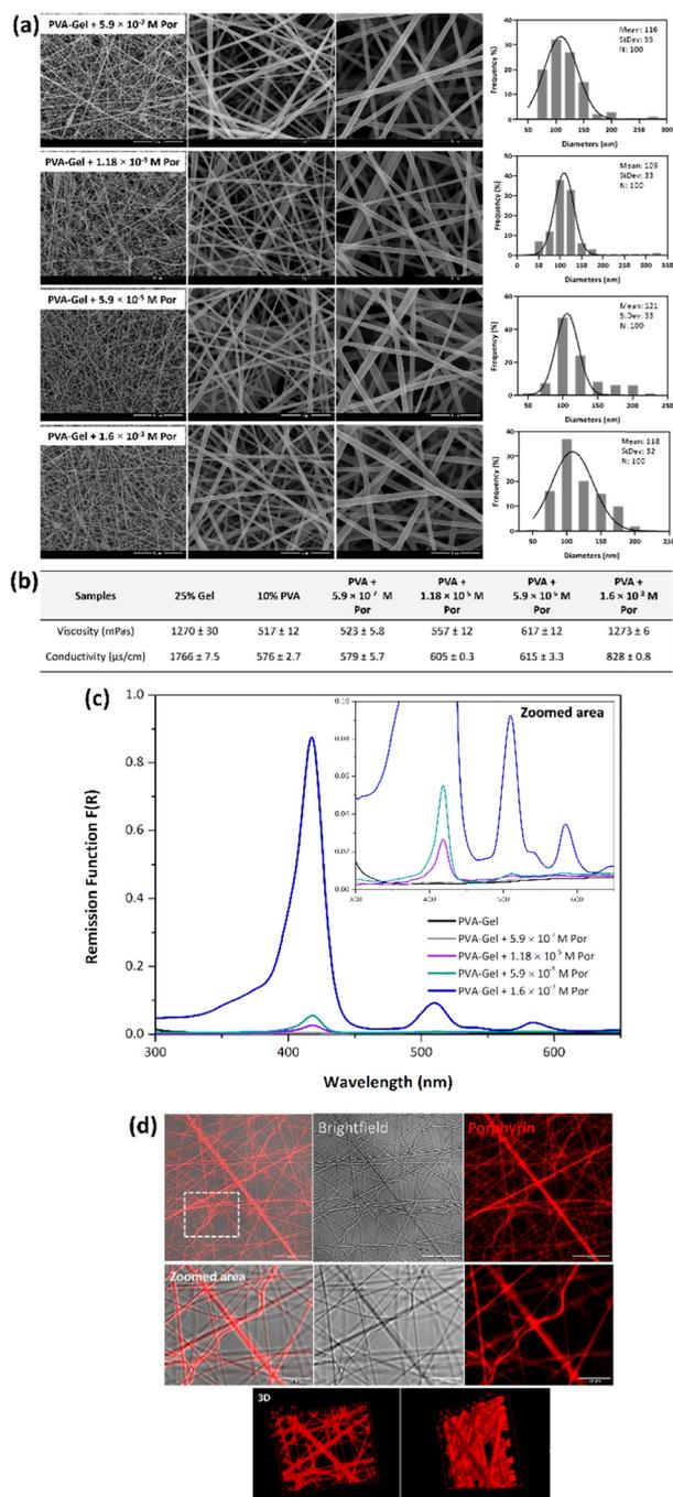
**Fig. 3** Images of (a) FESEM and the respective diameter distribution histograms of PVA-Gel nanofibers containing  $5.9 \times 10^{-7}$ ,  $1.18 \times 10^{-5}$ ,  $5.9 \times 10^{-5}$ , and  $1.6 \times 10^{-3}$  M of Por, (b) viscosity and conductivity values of the different solutions; spectra of (c) GSDR of PVA-Gel without and with different Por concentrations; and images of (d) CLSM of PVA-Gel + Por nanofibers excited at 405 nm and detected at 500–699 nm.
