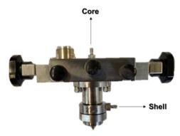
Co-axial accessory used to produce core-shell nanofibers
