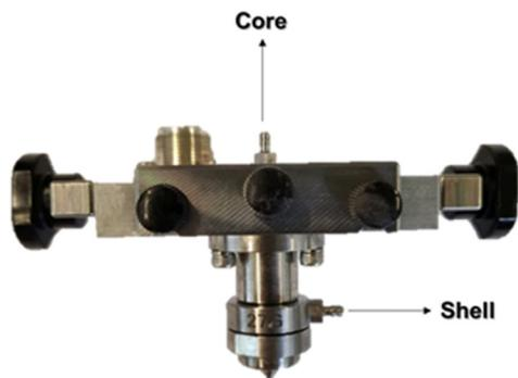
Fig. 1 Co-axial accessory used to produce core-shell nanofibers.
