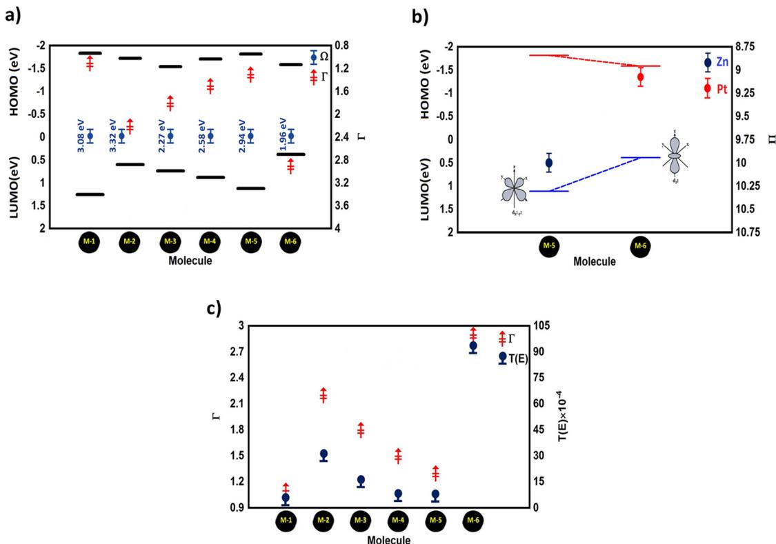
Fig. 4 (a) HOMO–LUMO gap ( $\Omega$ ) versus the number of transferred electrons ( $\Gamma$ ) of the molecular junctions; (b) orbital energies versus the number of electrons in the d-orbital ( $\Pi$ ) for M-5 and M-6 molecules, as example system with even and odd numbers of electrons; (c) number of transferred electrons from the molecule to the electrodes ( $\Gamma$ ) versus the transmission coefficient  $T(E)$  of all the molecular junctions.
