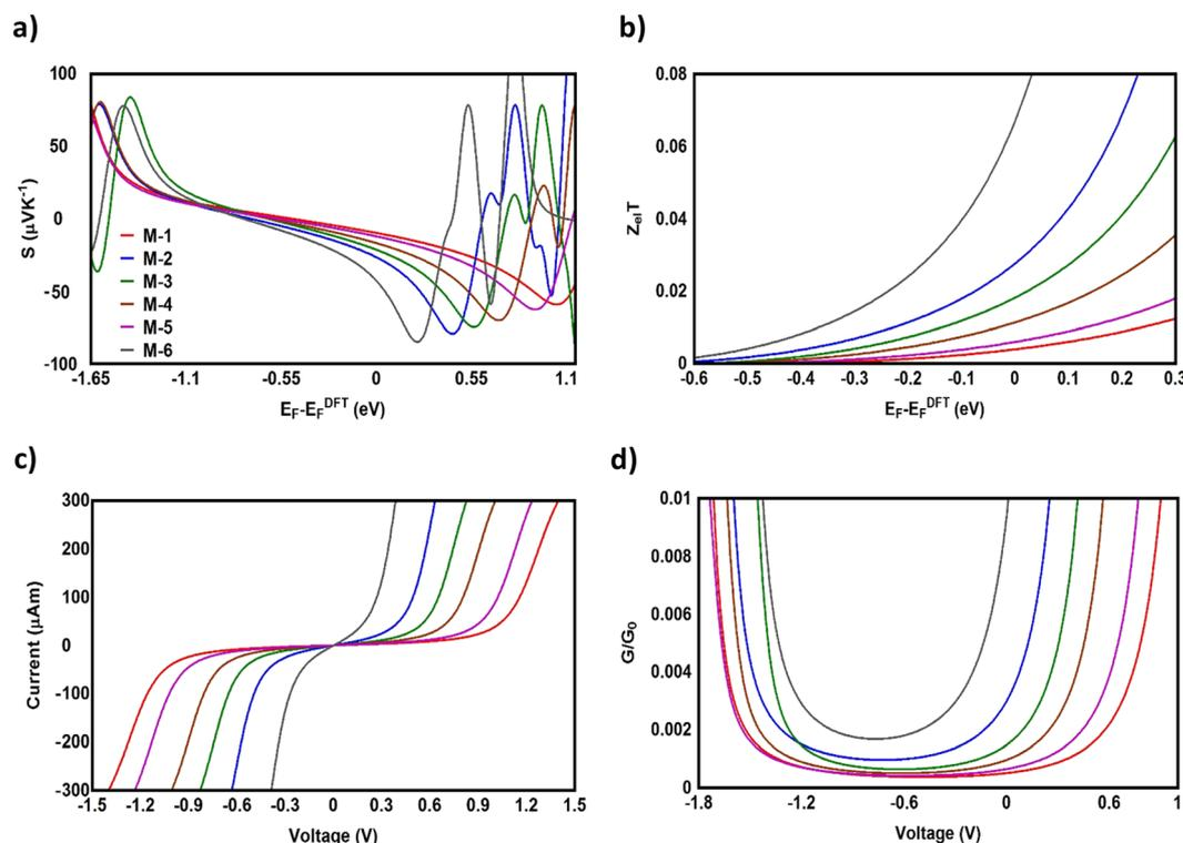
**Fig. 5** (a) Seebeck coefficient ( $S$ ); (b) electronic figure of merit ( $Z_{el}T$ ), as a function of the Fermi energy; (c) current-voltage characteristics; (d) electrical conductance ( $G/G_0$ ) as a function of voltage for all the molecular junctions.
