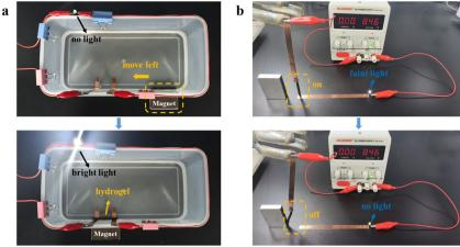
Fig. 6 (a) The  $Ca^{2+}$ - $Fe_3O_4$ @XLG/SL/PAM hydrogel connected the circuit in a non-contact form under the attraction of the external magnetic field. (b) The  $Ca^{2+}$ - $Fe_3O_4$ @XLG/SL/PAM hydrogel can control the disconnection and connection of circuits by applying a magnetic field.
