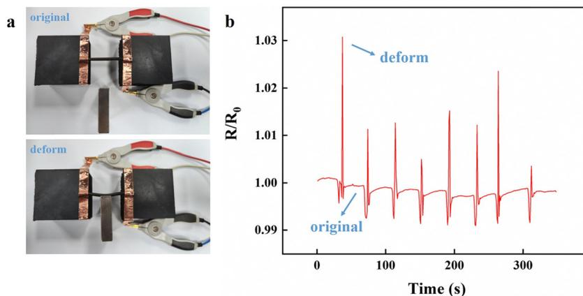
Fig. 5 (a) The  $\text{Ca}^{2+}\text{-Fe}_3\text{O}_4\text{@XLG/SL/PAM}$  hydrogel deformed under the external magnetic field. (b) Cyclic resistance change rate-time curves of the  $\text{Ca}^{2+}\text{-Fe}_3\text{O}_4\text{@XLG/SL/PAM}$  hydrogel.
