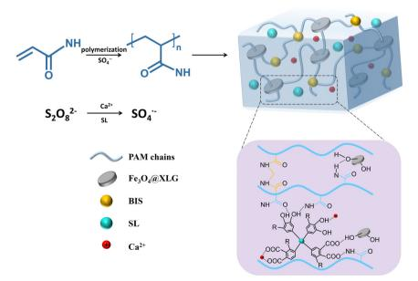
$Scheme \ 1 \quad Schematic \ illustration \ of \ fabrication \ process \ and \ structure \ of \ the \ proposed \ Ca^{2+} - Fe_3O_4@XLG/LS/PAM \ hydrogels.$
