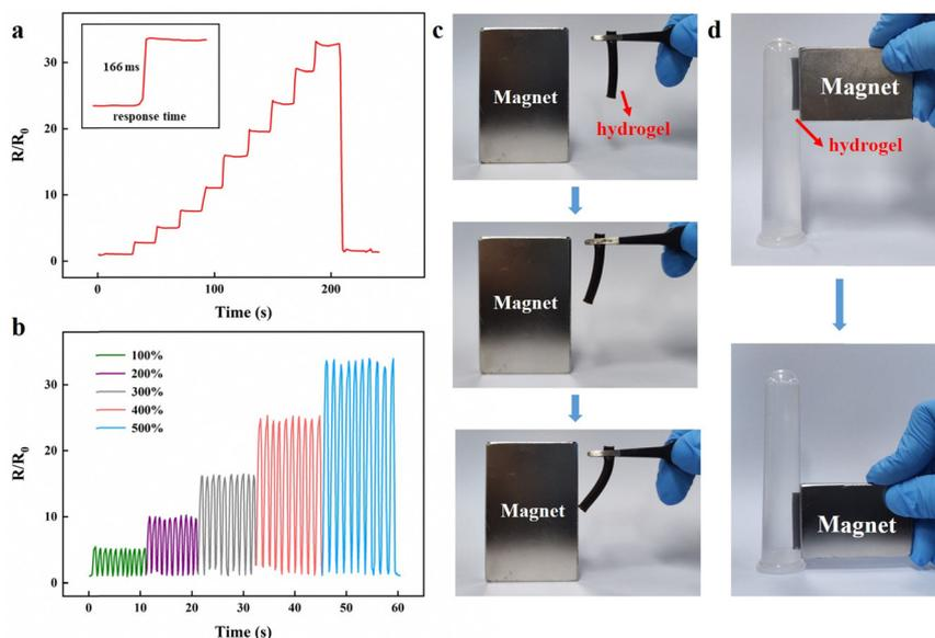
Fig. 4 (a) The resistance change of the  $\text{Ca}^{2+}\text{-Fe}_3\text{O}_4\text{@XLG/SL/PAM}$  hydrogel under different tensile strain. (b) Stability tests of the  $\text{Ca}^{2+}\text{-Fe}_3\text{O}_4\text{@XLG/SL/PAM}$  hydrogel when repeatedly stretched. (c) and (d) Magnetic responsive properties of the  $\text{Ca}^{2+}\text{-Fe}_3\text{O}_4\text{@XLG/SL/PAM}$  hydrogel.
