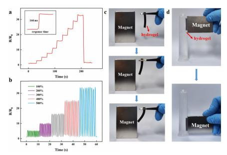
Fig. 4 (a) The resistance change of the Ca<sup>2+</sup>-Fe<sub>3</sub>O<sub>4</sub>@XLG/SL/PAM hydrogel under different tensile strain. (b) Stability tests of the Ca<sup>2+</sup>-Fe<sub>3</sub>O<sub>4</sub>@XLG/SL/PAM PAM hydrogel when repeatedly stretched. (c) and (d) Magnetic responsive properties of the Ca<sup>2+</sup>-Fe<sub>3</sub>O<sub>4</sub>@XLG/SL/PAM hydrogel.
