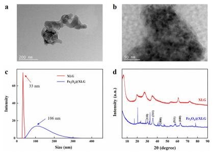
Fig. 1 The TEM images of (a) XLG and (b) Fe<sub>3</sub>O<sub>4</sub>@XLG NPs. (c) The size and (d) XRD spectra of XLG and Fe<sub>3</sub>O<sub>4</sub>@XLG NPs.
