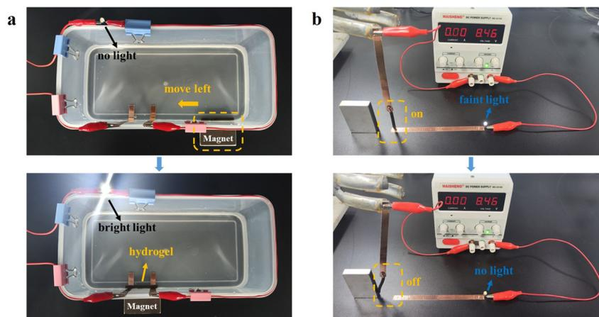
Fig. 6 (a) The  $\text{Ca}^{2+}\text{-Fe}_3\text{O}_4\text{@XLG/SL/PAM}$  hydrogel connected the circuit in a non-contact form under the attraction of the external magnetic field. (b) The  $\text{Ca}^{2+}\text{-Fe}_3\text{O}_4\text{@XLG/SL/PAM}$  hydrogel can control the disconnection and connection of circuits by applying a magnetic field.
