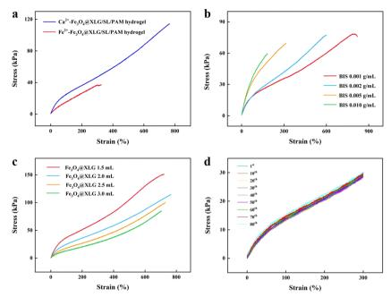
Fig. 2 Mechanical properties of the  $Ca^{2+}$ -Fe $_3O_4$ @XLG/SL/PAM hydrogel. (a) Stress-strain curves of the  $Ca^{2+}$ -Fe $_3O_4$ @XLG/SL/PAM hydrogel and the  $Fe^{3+}$ - $Fe_3O_4$ @XLG/SL/PAM hydrogel. Stress-strain curves of the  $Ca^{2+}$ - $Fe_3O_4$ @XLG/SL/PAM hydrogel with different dosage of (b) BIS and (c)  $Fe_3O_4$ @XLG. (d) Elasticity of the Ca<sup>2+</sup>-Fe<sub>3</sub>O<sub>4</sub>@XLG/SL/PAM hydrogel under 80 successive loading-unloading cycles.
