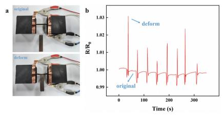
Fig. 5 (a) The Ca<sup>2+</sup>-Fe<sub>3</sub>O<sub>4</sub>@XLG/SL/PAM hydrogel deformed under the external magnetic field. (b) Cyclic resistance change rate-time curves of the Ca2+-Fe3O4@XLG/SL/PAM hydrogel.
