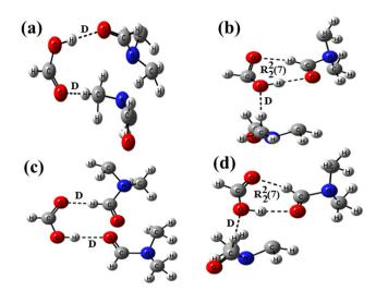
Fig. 3 Optimized structures of formic acid–DMF at the B3LYP/6-31+ $G^*$  level showing (a) two D motifs, (b) D and  $R_2^2(7)$  motifs, (c) two D motifs and (d) D and  $R_2^3(7)$  motifs.
