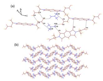
Fig. 1 (a) Part of the crystal lattice of  ${\bf 1a}$  showing intermolecular host-host and host-guest interactions. (b) A 3D supramolecular host-guest helical network of  ${\bf 1a}$  (along the c axis).
