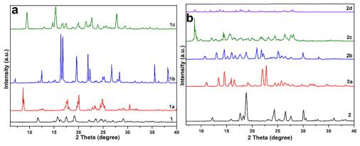
Fig. 12 PXRD patterns of (a) host 1 and its solvates 1a, 1b and 1c and (b) host 2 and its solvates 2a, 2b, 2c and 2d.
