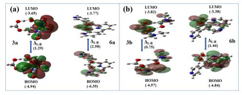
Fig. 11 Optimized Frontier molecular orbitals and orbital energies (in eV) of structures (a) 3a and 6a and (b) 3b and 6b via DFT at the B3LYP/6-31+G\*
