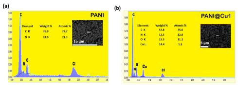
Fig. 7 (a) EDX spectra of PANI and (b) the PANI@Cu nanocomposite
