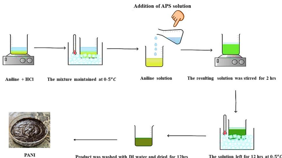
Scheme 1 Aniline and ammonium persulfate are used in the synthesis of PANI in acidic medium.
