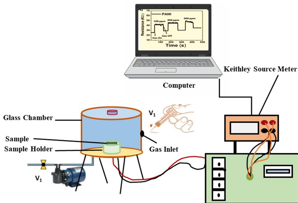
Fig. 2 Schematic diagram of a gas sensing experimental setup.
