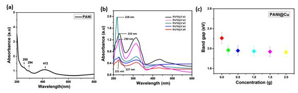
UV spectrum of (a) pure PANI and (b) the PANI@Cu nanocomposite, (c) the band gap of PANI and PANI@Cu1-5 with various concentrations.
