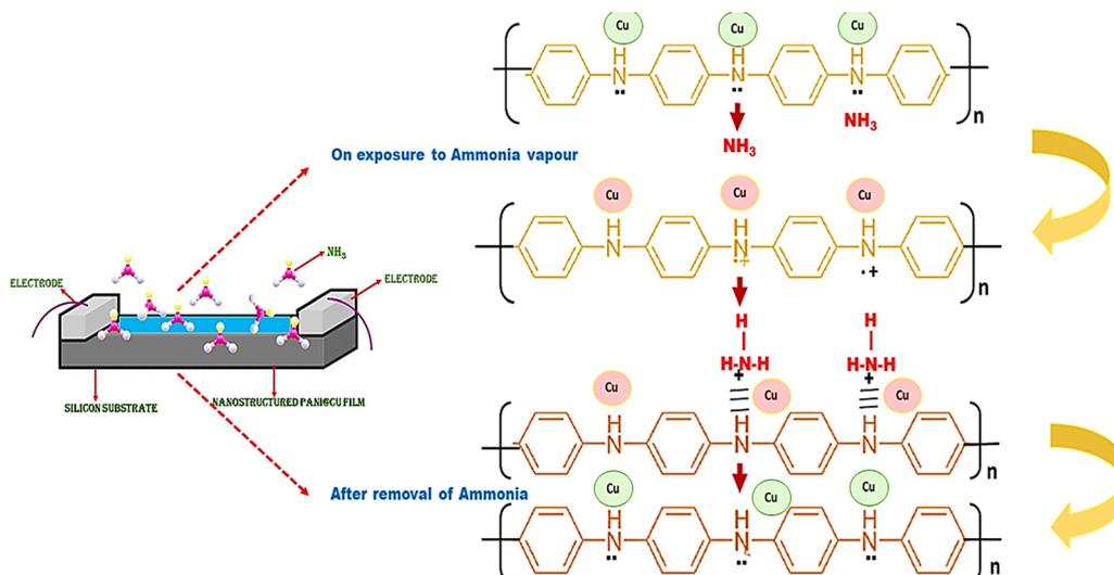
Fig. 12 Schematic of the ammonia sensing mechanism.
