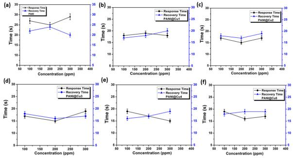
Fig. 10 Response and recovery time plot for (a) pure PANI film and (b)–(f) the PANI@Cu nanocomposite film when exposed to various concentrations of  $NH_{\pi}$  gas at room temperature.
