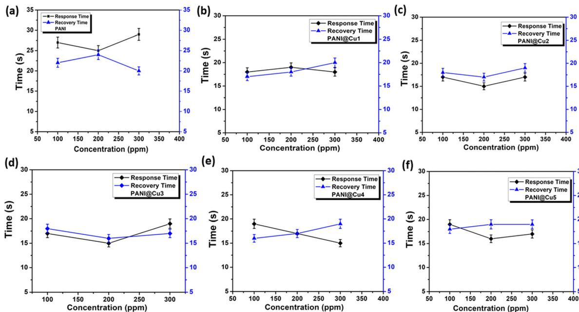
Fig. 10 Response and recovery time plot for (a) pure PANI film and (b)–(f) the PANI@Cu nanocomposite film when exposed to various concentrations of NH<sub>3</sub> gas at room temperature.
