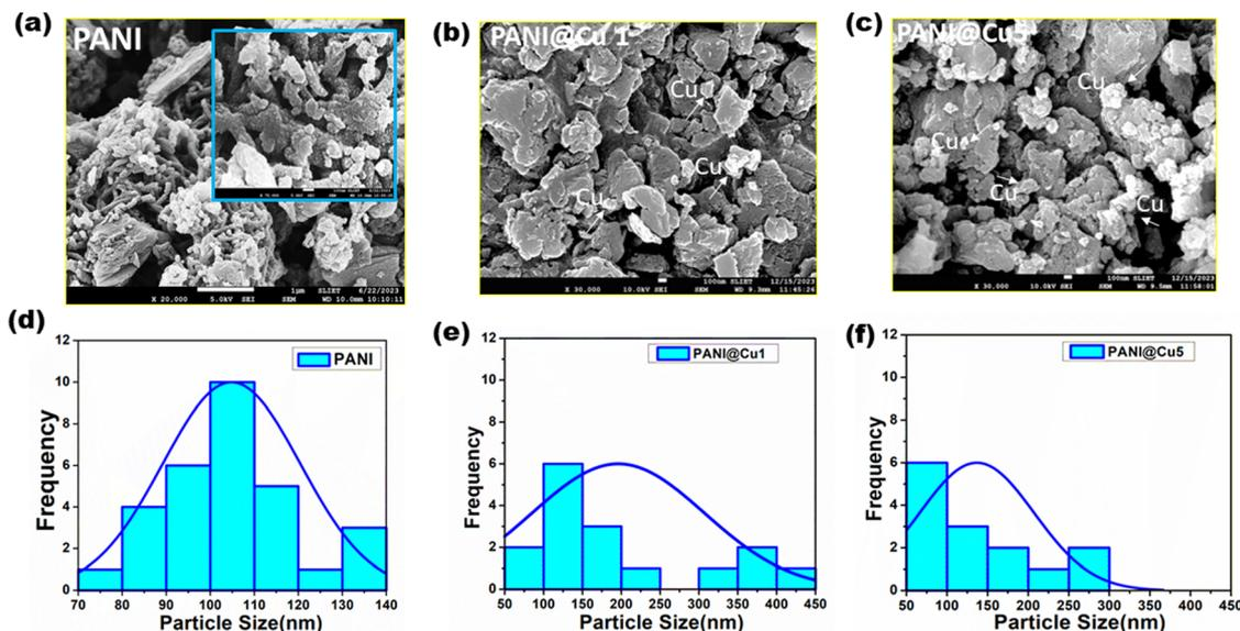
Fig. 6 FE-SEM of (a) PANI and (b) and (c) the PANI@Cu nanocomposites, and (d)–(f) particle size analysis of the samples.
