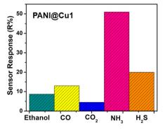
Fig. 11 Selectivity of (a) PANI and (b) the PANI@Cu1 nanocomposite film gas sensor.
